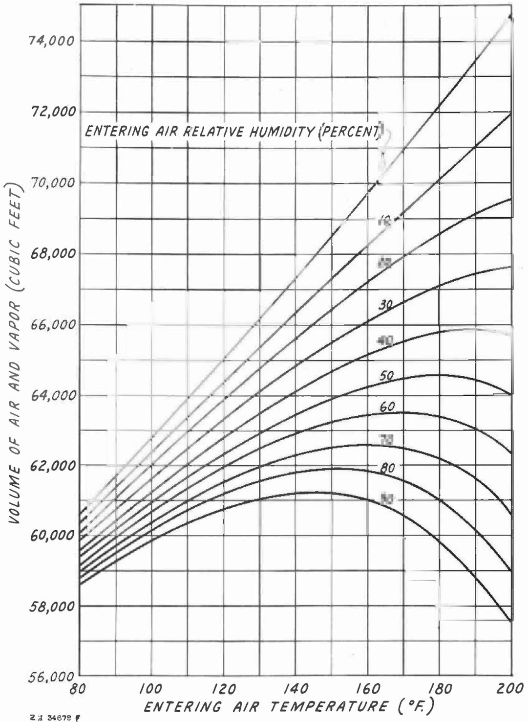
Figure 1.--Amount of air and vapor needed to evaporate 1 pound of water when the temperature drop across the load is 1° F.
