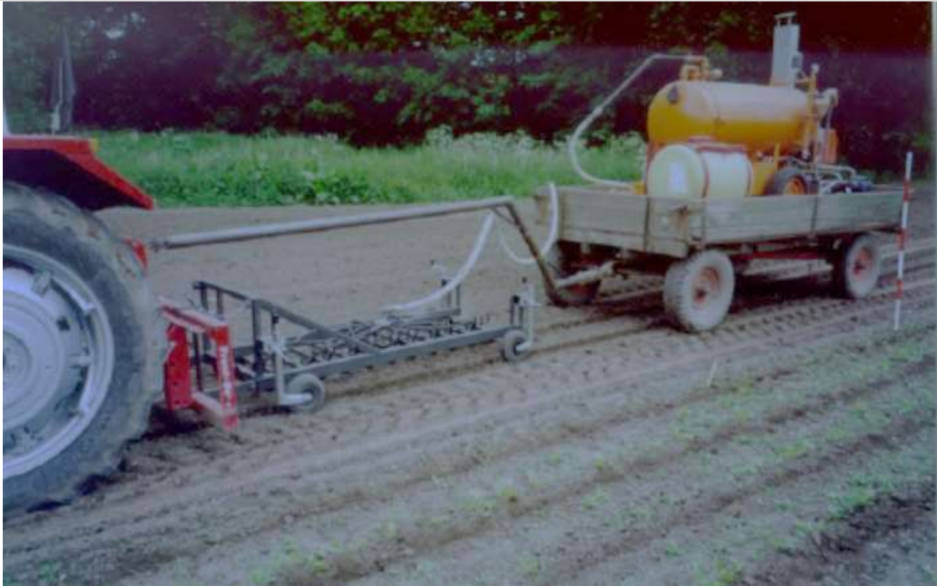
2000 KW bed steamer with 13 tines
