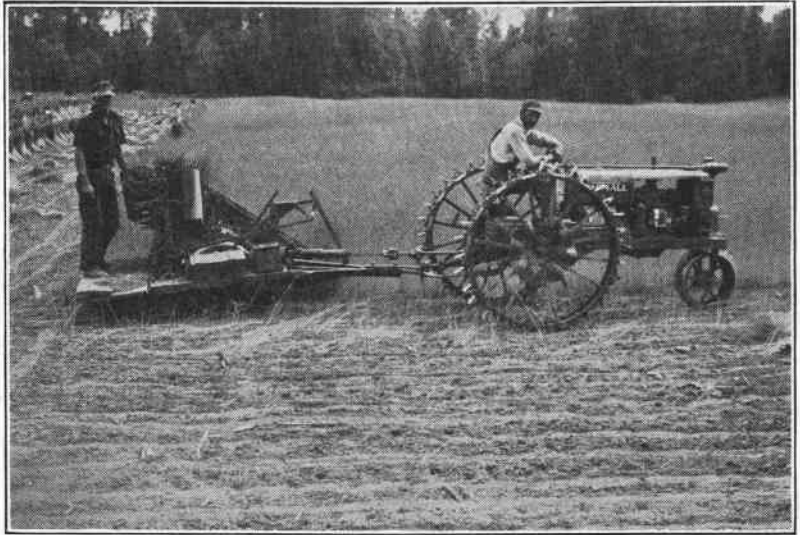
Figure 1. Flax pulling machines harvest Oregon's fiber flax economically. A machine will pull approximately five acres of flax in a day.
