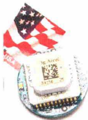
Figure 2: MEMS based analog accelerometer in comparison to a USA stamp [7].
