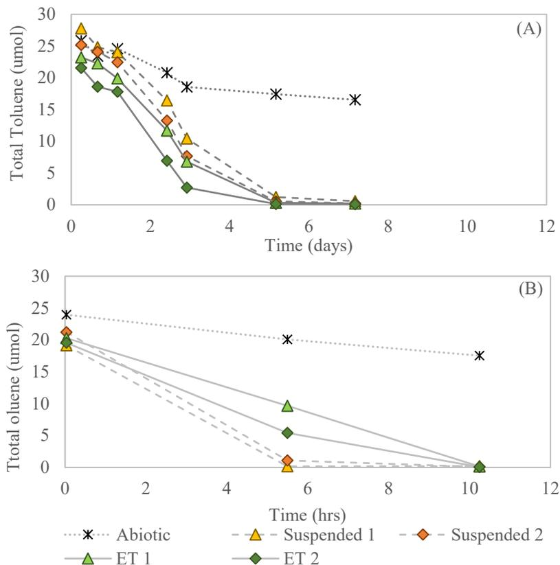
**Figure E- 1** Toluene utilization by suspended and encapsulated in gellan gum macrobeads *B. vietnamiensis* G4 at approximately the same biomass ( $4 \text{ mg}_{TSS}$ ) (A) after beads were made and (B) after 237 days stored at  $4^\circ\text{C}$ . Beads had a biomass loading of  $1 \text{ mg}_{TSS}/\text{g}_{bead}$ . Data shown for duplicates of each treatment and a single abiotic control.
