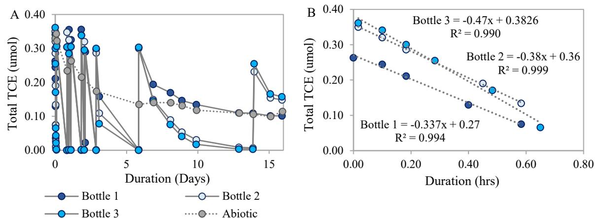
**Figure 3.3** Kinetic degradation results of TCE by resting benzyl alcohol grown *B. vietnamiensis* G4 (4.2  $\text{mg}_{\text{TSS}}$ ) showing (A) TCE reinjections to determine total transformation capacity ( $\mu\text{mol}/\text{mg}_{\text{TSS}}$ ) and (B) initial degradation of TCE to determine initial zero order rate ( $\mu\text{mol}/\text{day}/\text{mg}_{\text{TSS}}$ ).
