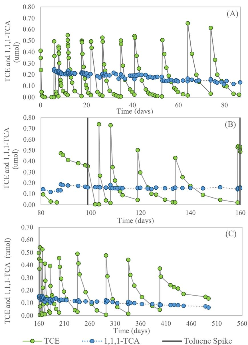
**Figure 4.4** Cometabolic transformation of TCE by G4 in gellan gum macrobeads (2 g beads/reactor) at a biomass loading of 1  $\text{mg}_{\text{TSS}}/\text{g}_{\text{bead}}$ . Data shown for singlet that deviated. Beads (~20%) were removed on day 88 and the media was replaced. Toluene was added (74  $\mu\text{mol}$ ) on day 99.
