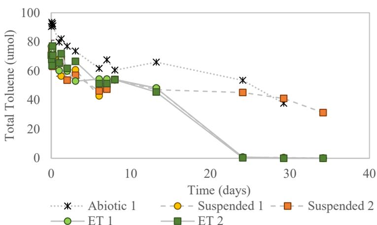
**Figure 4.12** Toluene consumption by encapsulated and suspended *B. vietnamiensis* G4 after an addition made on day 84 in all treatment. It took at least 24 days for all treatments (except Suspended 2) for complete toluene uptake.
