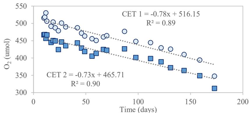
**Figure 4.18** Zero-order oxygen utilization rates for duplicate CET active reactors from day 10 – 173.
