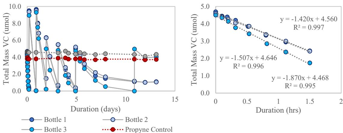
**Figure S- 4** Kinetic degradation results of VC by resting benzyl alcohol grown *B. vietnamiensis* G4 (5.0 mg<sub>TSS</sub>) showing (A) VC reinjections to determine total transformation capacity (umol/ mg<sub>TSS</sub>) and (B) initial degradation of VC to determine initial zero order rate (umol/day/mg<sub>TSS</sub>).
