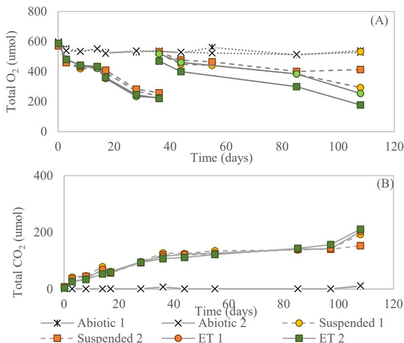
**Figure 4.11** (A) O<sub>2</sub> utilization and (B) CO<sub>2</sub> production by encapsulated G4 macrobeads (2 g beads/reactor) at a biomass loading of 8 mg<sub>TSS</sub>/g<sub>bead</sub>. Treatments consisted of duplicate encapsulated and suspended treatments at approximately equivalent biomass loadings. Pure oxygen was added to the headspace on day 26 for both encapsulated and suspended treatments. ET—encapsulated treatment.
