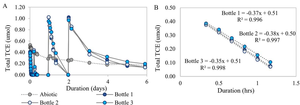
**Figure 3.2** Kinetic degradation results of TCE by resting toluene grown *B. vietnamiensis* G4 (5  $\text{mg}_{\text{TSS}}$ ) showing (A) TCE reinjections to determine total transformation capacity ( $\mu\text{mol}/\text{mg}_{\text{TSS}}$ ) and (B) initial degradation of TCE to determine initial zero order rate ( $\mu\text{mol}/\text{day}/\text{mg}_{\text{TSS}}$ ).
