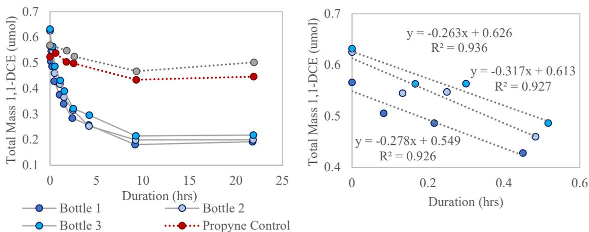
**Figure S6.** Kinetic degradation results of 1,1-DCE by resting benzyl alcohol grown *B. vietnamiensis* G4 (4.8 mg<sub>TSS</sub>) showing (A) 1,1-DCE reinjections to determine total transformation capacity (umol/ mg<sub>TSS</sub>) and (B) initial degradation of 1,1-DCE to determine initial zero order rate (umol/day/mg<sub>TSS</sub>).
