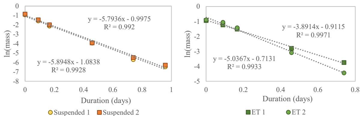
**Figure 4.2** First-order plots of initial TCE transformation over time for (A) suspended reactors and (B) encapsulated reactors ( $1 \text{ mg}_{\text{TSS}}/\text{g}_{\text{bead}}$ ) of *B. vietnamiensis* G4 at biomass of ( $2 \text{ mg}_{\text{TSS}}/\text{reactor}$ ). Reactors were in duplicate.
