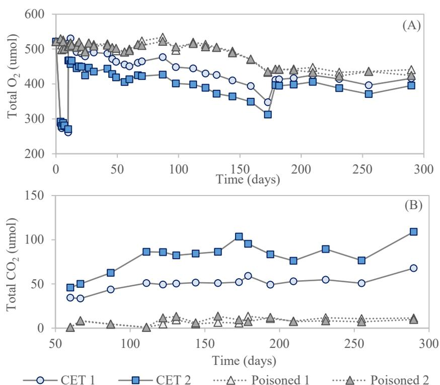
**Figure 4.17** (A) Oxygen utilization and (B) carbon dioxide production by co-encapsulated TPhOS and G4 beads (2 g). Beads were made at a biomass loading of 1.45  $\text{mg}_{\text{TSS}}/\text{g}_{\text{bead}}$  and 1.9% (w/w) TPhOS. Treatments consisted of duplicate sodium azide (2% v/v) poisoned controls with co-encapsulated beads, and duplicate active co-encapsulated treatments in media. Active treatments were opened on day 181, and 15% of beads were removed. (CET)—Co-encapsulated Treatment.
