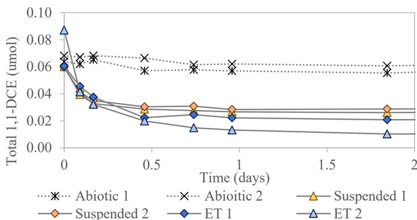
**Figure 4.1** Cometabolic transformation of (A) 1,1-DCE by immobilized *G4* in gellan gum macrobeads (2 g beads/reactor) at a biomass loading of  $1 \text{ mg}_{\text{TSS}}/\text{g}_{\text{bead}}$ . Encapsulated treatment—ET
