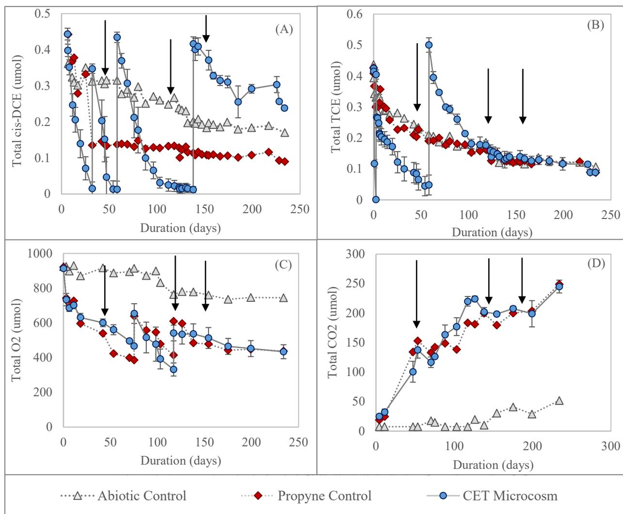
**Figure 4.21** Cometabolic transformation of (A) *cis*-DCE, (B) TCE, (C) O<sub>2</sub> utilization, and (D) CO<sub>2</sub> production in Fort Carson microcosms. (CET)—Co-encapsulated treatments with G4 and TPhOS at 1.9% (w/w) were in triplicate and abiotic and propyne controls were singlets. Arrows indicate nutrient additions.
