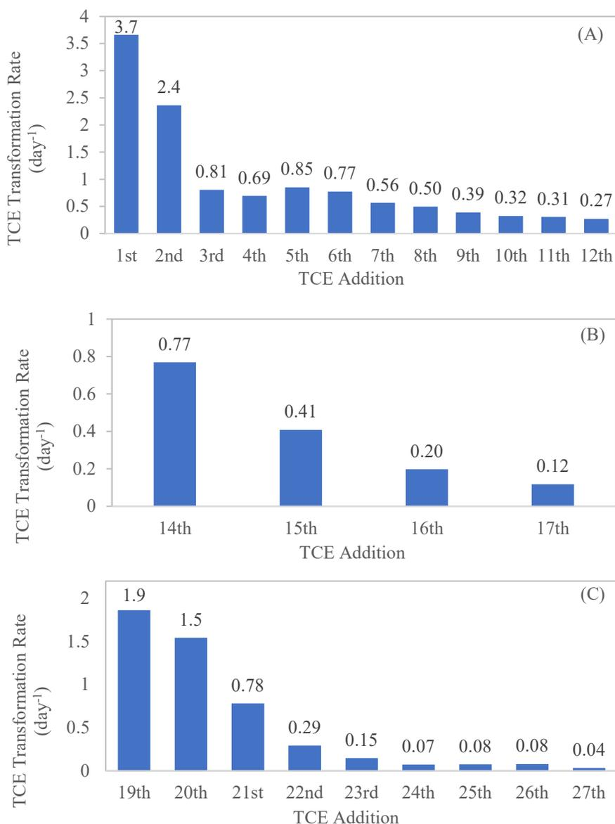
**Figure 4.5** Pseudo-first order TCE transformation rates for each addition of TCE by singlet encapsulated *B. vietnamiensis* G4 reactor (1  $\text{mg}_{\text{TSS}}/\text{g}_{\text{bead}}$ ) with an initial biomass of 2  $\text{mg}_{\text{TSS}}$ . (A) Rates for resting cells, (B) rates after first addition of toluene on day 99, (C) rates after second addition of toluene on day 160.
