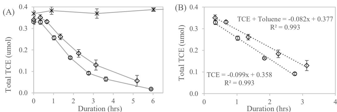
**Figure 3.5** TCE disappearance by resting *B. vietnamiensis* G4 (○), with toluene at 11.7 mg/L (◇), and with 2% (v/v) propyne as a monooxygenase inhibitor (×). Shown is (A) raw data and (B) zero-order rate regression. Treatments were done in triplicate with error bars representing SD for  $n = 3$ .
