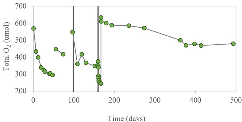
**Figure 4.6** Oxygen utilization by singlet reactor that diverged containing encapsulated G4 in gellan gum macrobeads. Toluene additions signified by lines at days 99 and 160.
