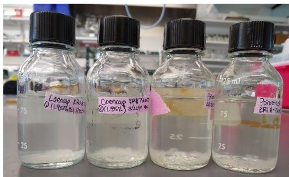
**Figure 4.20** From left to right: duplicates of active and poisoned treatments of co-encapsulated KR1 and 1.9% (w/w) TPhOS at day 112. Macro beads are at the bottom of the bottles. It is believed the majority of biomass is immobilized in the beads, as no visible growth in suspension is seen in the active treatments compared to the poisoned controls.
