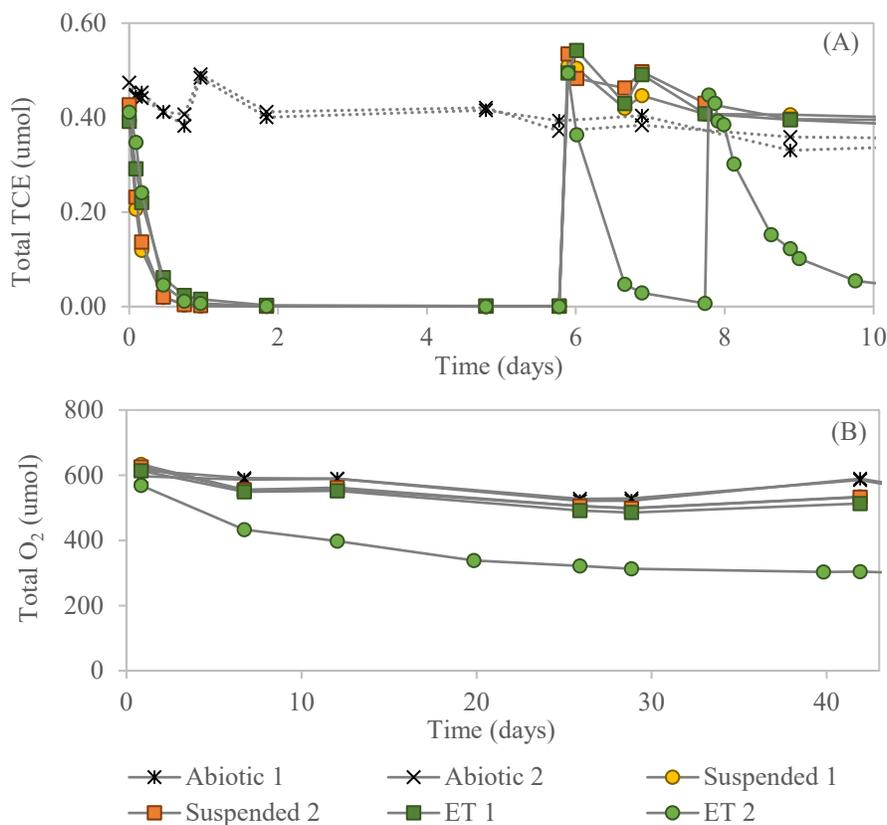
**Figure 4.3** Cometabolic transformation of (A) TCE and (B) O<sub>2</sub> utilization by immobilized G4 in gellan gum macrobeads ( $2 \text{ g beads}/\text{reactor}$ ) at a biomass loading of  $1 \text{ mg}_{\text{TSS}}/\text{g}_{\text{bead}}$ . One of the encapsulated reactors transforming TCE diverged on day 6. Data shown is for duplicates of each treatment. Encapsulated treatment—ET
