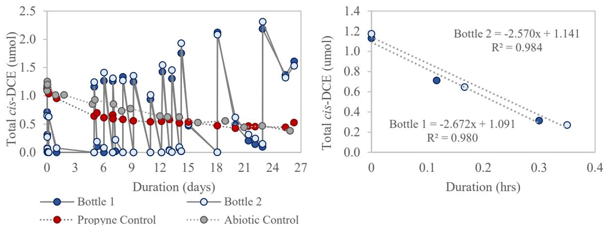
**Figure 3.10** Kinetic degradation results of *cis*-DCE by resting toluene-grown *B. vietnamiensis* G4 (5.5 mg<sub>TSS</sub>) showing (A) *cis*-DCE reinjections to determine total transformation capacity (umol/mg<sub>TSS</sub>) and (B) initial degradation of *cis*-DCE to determine initial zero order rate (umol/day/mg<sub>TSS</sub>).
