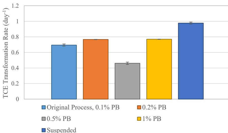
**Figure D-2** Comparison of pseudo-first order rates of TCE transformation for suspended and encapsulated *B. vietnamiensis* G4 in gellan gum macrobeads with 1.6 M phosphate buffer (PB) at 0.1%, 0.2%, 0.5%, and 1% (v/v). For 0.1, 0.2, 0.5, and 0.1% PB, error bars represent the range of duplicate reactors. Error bars for suspended treatment represent standard deviation with  $n=4$ .
