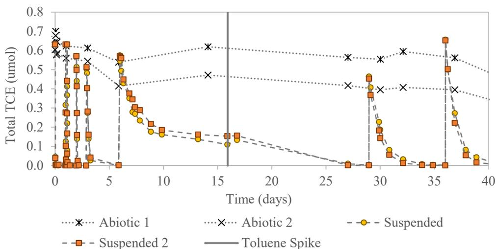
**Figure S-1** Cometabolic transformation of TCE over the course of 40 days by *B. vietnamiensis* G4. Treatments consisted of duplicate treatments of suspended cells of *B. vietnamiensis* G4 at 16 mg<sub>TSS</sub>/reactor, and duplicate abiotic control treatments. Toluene was added on day 16 to stimulate further cometabolic activity.
