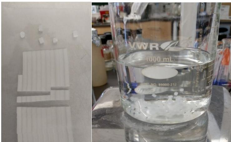
**Figure 2.1** (Left) Strands of gellan gum extruded from 2 mm diameter rubber tubing and cut into cylindrical pellets in a sterile laminar flow hood. (Right) After cutting, beads were transferred to a 0.25% CaCl<sub>2</sub> crosslinking solution.
