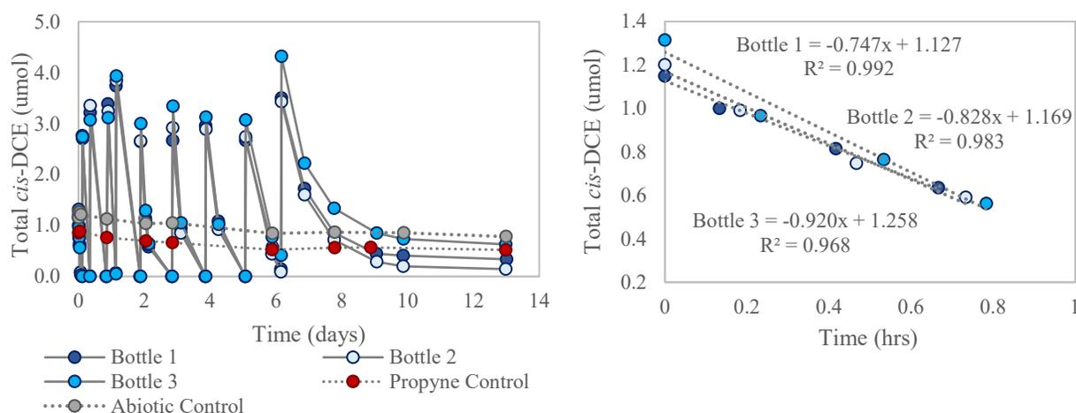
**Figure 3.11** Kinetic degradation results of *cis*-DCE by resting benzyl alcohol grown *B. vietnamiensis* G4 (4.8 mg<sub>TSS</sub>) showing (A) TCE reinjections to determine total transformation capacity (umol/mg<sub>TSS</sub>) and (B) initial degradation of TCE to determine initial zero order rate (umol/day/mg<sub>TSS</sub>).
