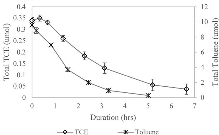
**Figure S-2** Results of concurrent TCE and Toluene disappearance by *B. vietnamiensis* G4 (1 mg<sub>TSS</sub>). Initial toluene liquid concentration was 11.7 mg/L. Treatment was done in triplicate with error bars representing SD for  $n = 3$ .
