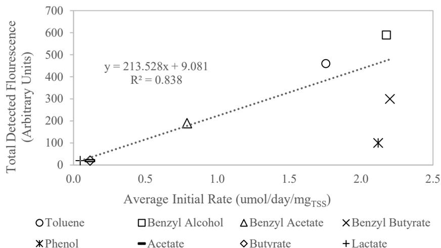
**Figure 3.4** Regression analysis of total detected fluorescence and the average initial rate for toluene, benzyl alcohol, benzyl acetate, benzyl butyrate, phenol, acetate, butyrate, and lactate grown *B. vietnamiensis* G4. Linear regression is shown for the data with the exception of phenol as an outlier.
