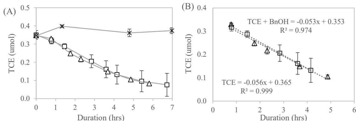
**Figure 3.7** TCE disappearance by resting *B. vietnamiensis* G4 alcohol ( $\square$ ) and with benzyl alcohol at 10 mg/L ( $\Delta$ ), and with 2% (v/v) propyne as a monooxygenase inhibitor ( $\times$ ). Shown is (A) raw data and (B) zero-order rate regression. Treatments were done in triplicate with error bars representing SD for  $n = 3$ .
