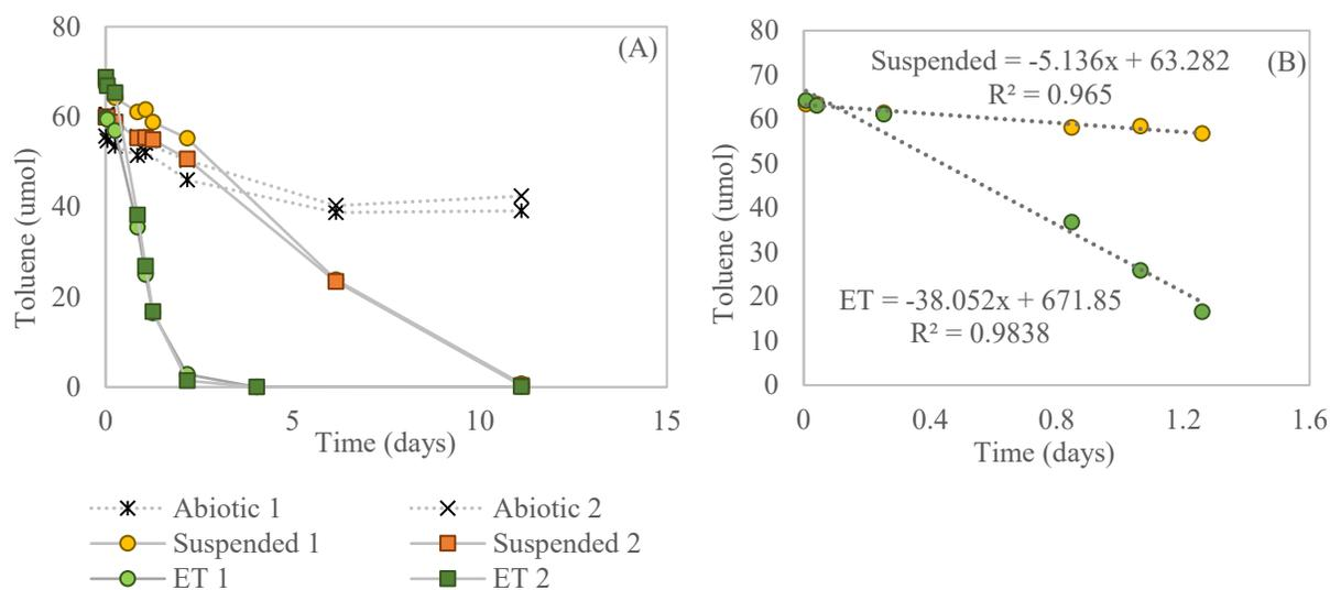
**Figure 4.10** (A) Toluene consumption after an addition made on day 16 in all treatments. Encapsulated treatments completely transformed toluene in four days, whereas suspended treatments transformed it in eleven days. (B) Average zero-order toluene uptake rates for suspended and encapsulated treatments of *B. vietnamiensis* G4 ( $16 \text{ mg}_{\text{TSS}}/\text{reactor}$ )
