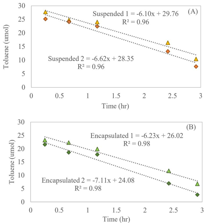
**Figure E-2** Initial zero-order substrate utilization rates for (A) suspended and (B) encapsulated *B. vietnamiensis* G4 at 4 mg<sub>TSS</sub>/reactor.
