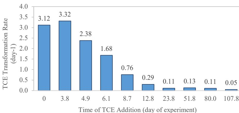
**Figure 4.16** Average psuedo-first order TCE transformation rates for each addition of TCE added to active treatments of co-encapsulated TPhOS (1.8%) and G4 (2 g of beads/reactor). Beads were made at a biomass loading of 1.45  $\text{mg}_{\text{TSS}}/\text{g}_{\text{bead}}$  and 1.8% (w/w) TPhOS. The rate of transformation decreased over time and was stable from day 23.8 to day 107.8 before decreasing on the next TCE addition.
