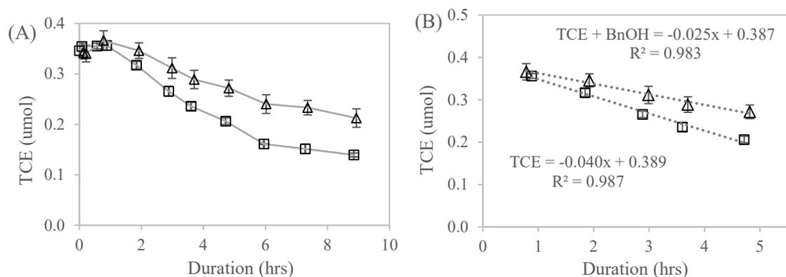
**Figure 3.8** TCE disappearance by resting *B. vietnamiensis* G4 ( $\square$ ) and with benzyl alcohol at 20 mg/L ( $\Delta$ ). Shown is (A) raw data and (B) zero-order rate fit. Treatments were done in triplicate with error bars representing SD for  $n = 3$ .
