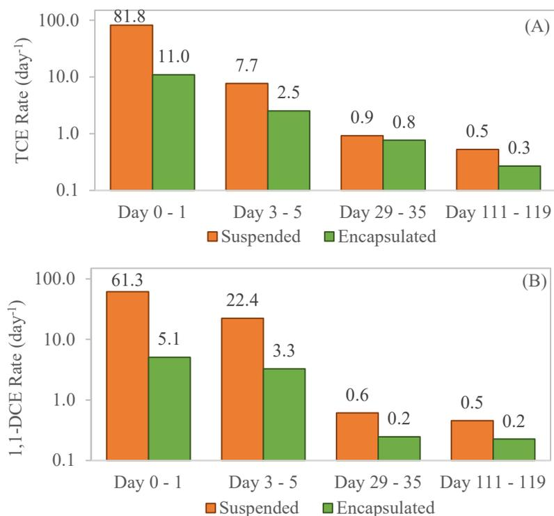
**Figure 4.9** Comparison of average pseudo-first order rates for (A) TCE and (B) 1,1-DCE in suspended and encapsulated treatments of *B. vietnamiensis* G4 (16 mg<sub>TSS</sub>/reactor) at various time intervals: initial rates (Day 0 - 1), before resting transformation capacity is reached (Day 3 - 5), after an addition of toluene (Day 29 - 35), and after a second addition of toluene (Day 111 - 119).
