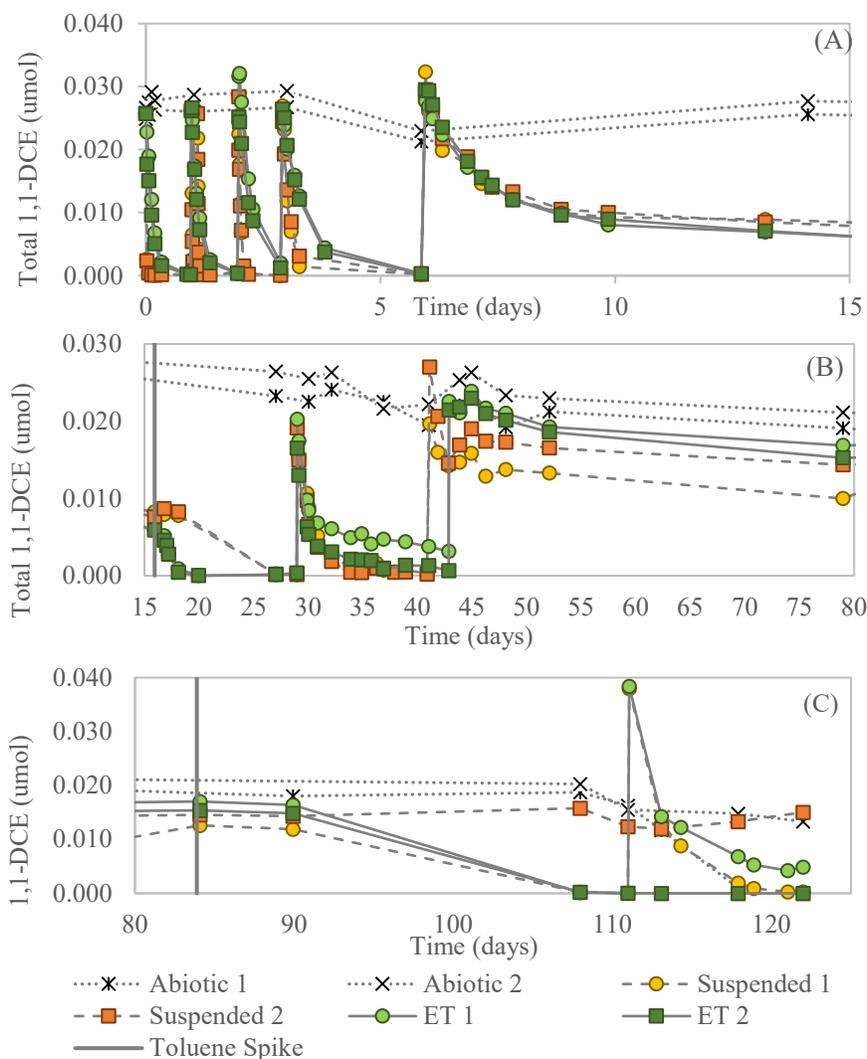
**Figure 4.8** Cometabolic transformation of 1,1-DCE by resting encapsulated and suspended immobilized *B. vietnamiensis* G4 at 16 mg<sub>TSS</sub>/reactor (A) resting cell transformation, (B) transformation after 1<sup>st</sup> toluene addition (day 16), (C) transformation after 2<sup>nd</sup> toluene addition (day 84). Treatment: duplicate encapsulated G4 (8 mg<sub>TSS</sub>/g<sub>bead</sub>), duplicate suspended G4, and duplicate abiotic controls.
