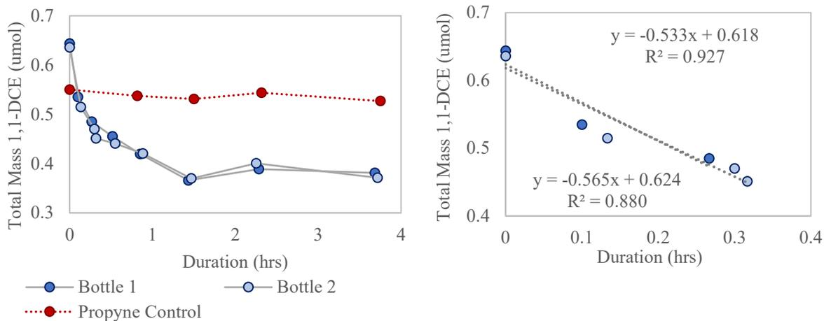
**Figure S- 5** Kinetic degradation results of 1,1-DCE by resting toluene grown *B. vietnamiensis* G4 (5.5 mg<sub>TSS</sub>) showing (A) 1,1-DCE reinjections to determine total transformation capacity (umol/ mg<sub>TSS</sub>) and (B) initial degradation of 1,1-DCE to determine initial zero order rate (umol/day/mg<sub>TSS</sub>).
