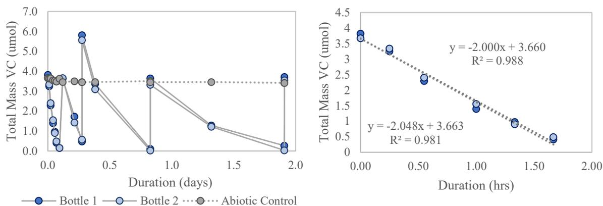
**Figure S- 3** Kinetic degradation results of VC by resting toluene grown *B. vietnamiensis* G4 (5.0 mg<sub>TSS</sub>) showing (A) VC reinjections to determine total transformation capacity (umol/ mg<sub>TSS</sub>) and (B) initial degradation of VC to determine initial zero order rate (umol/day/mg<sub>TSS</sub>).
