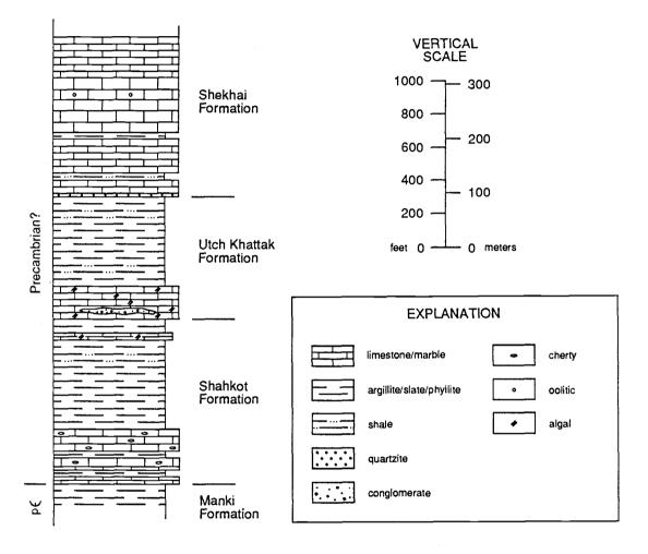
Figure 6. Schematic stratigraphic column for the southern Gandghar Range. Thickness of limestone "brick" pattern (not drawn to scale) indicates relative bedding thickness; e.g. thinnest "bricks" indicate thin-bedded limestone, thickest "bricks" indicate thick-bedded/massive limestone. Intraformational conglomerate in Utch Khattak Formation is exposed at the mouth of the canyon near Amgah. **KHERIMAR HILLS**
