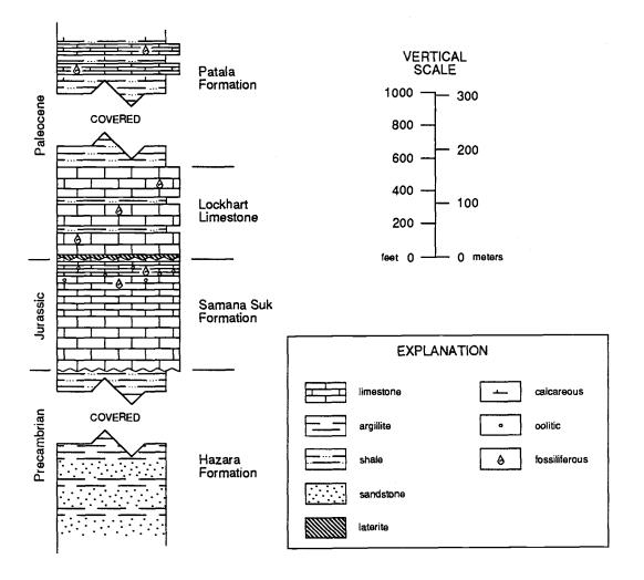
Figure 7. Schematic stratigraphic column for the Kherimar Hills. Thickness of limestone "brick" pattern (not drawn to scale) indicates relative bedding thickness as described in Figure 6.
