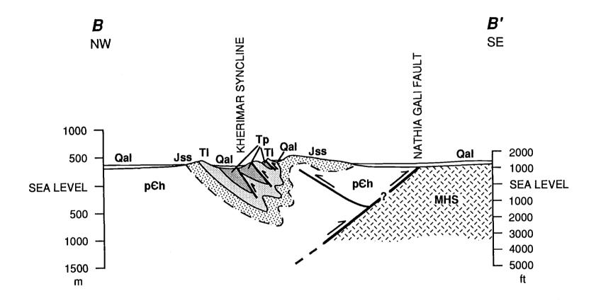
Figure 13. Structural cross section of the Kherimar Hills, showing overturned southern limb of the Kherimar syncline and postulated blind backthrust. No vertical exaggeration.  $p \in h$  = Hazara Formation; Jss = Samana Suk Formation; Tl = Lockhart Limestone; Tp = Patala Formation; Qal = alluvium. MHS = Margala Hills succession. See Figure 3 for location of cross section.
