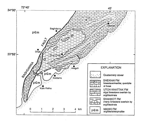
Figure 8. Lithologic map of the southern Gandghar Range in the vicinity of Dhar Chitti, showing basal Shekhai quartzite and distribution of limestone versus argillite and shale in Shahkot and Utch Khattak formations. Lithologic contacts represented by thin lines; formation contacts (dashed where approximately located) represented by medium lines; faults represented by thick lines.
