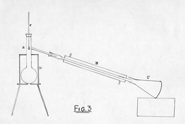
solution was filtered to remove fine charcoal powder which could have come into the condensate along with the vapors coming out of the retort. The tar was extracted successively with sodium bicarbonate (6%) solution and sodium hydroxide (6%) solution. The extractions were done with fresh solutions each time till the extract was fairly colorless. The substances not extracted by either of the above solutions were assumed to be the neutrals.
