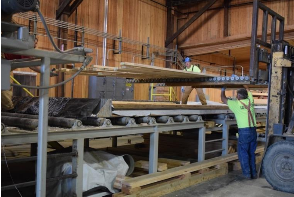
Figure 26: Layup of the major strength direction of the panels. One ply of lumber is laid-up on the forks of the forklift, which have wheels to roll the lumber off. The linemen simply need to ensure that the lumber is laid-up tightly.
