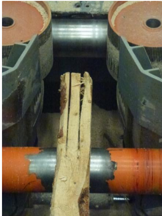
Figure 19: The HewSaw breakdown process began and was unable to continue through the saw, as the piece got jammed on the conveyor.
