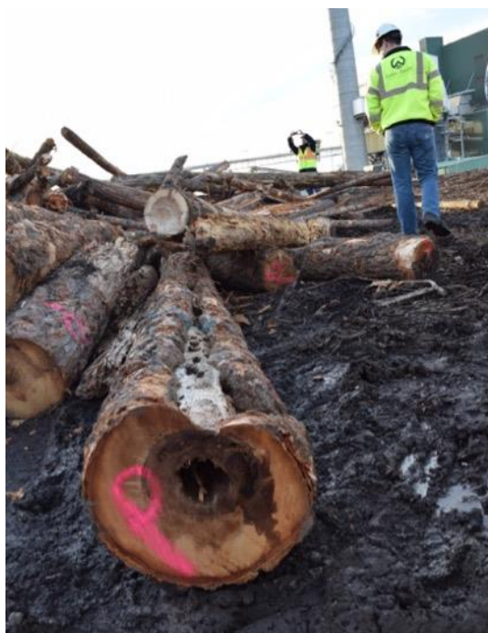
Figure 15: A delivered log to IFG that was rejected due to having too much sweep, or curvature to the log.
