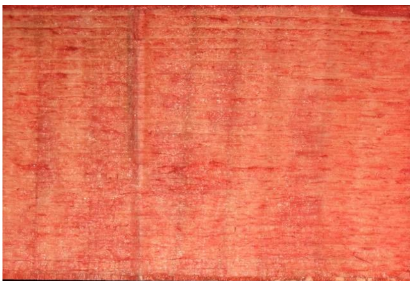
Figure 48: Example of some of the difficulty with safranin stain; where wood failure is present but minor, making it difficult to distinguish from the resin failure.
