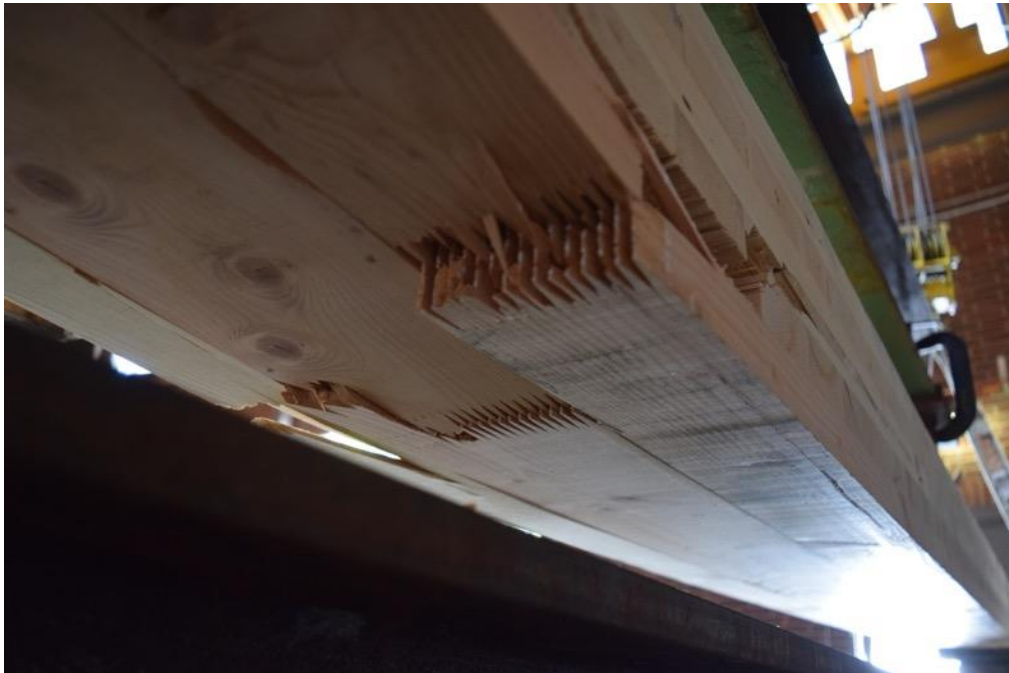
Figure 54: Failure of a 5-ply third-point test specimen at two finger joints, which were close together.
