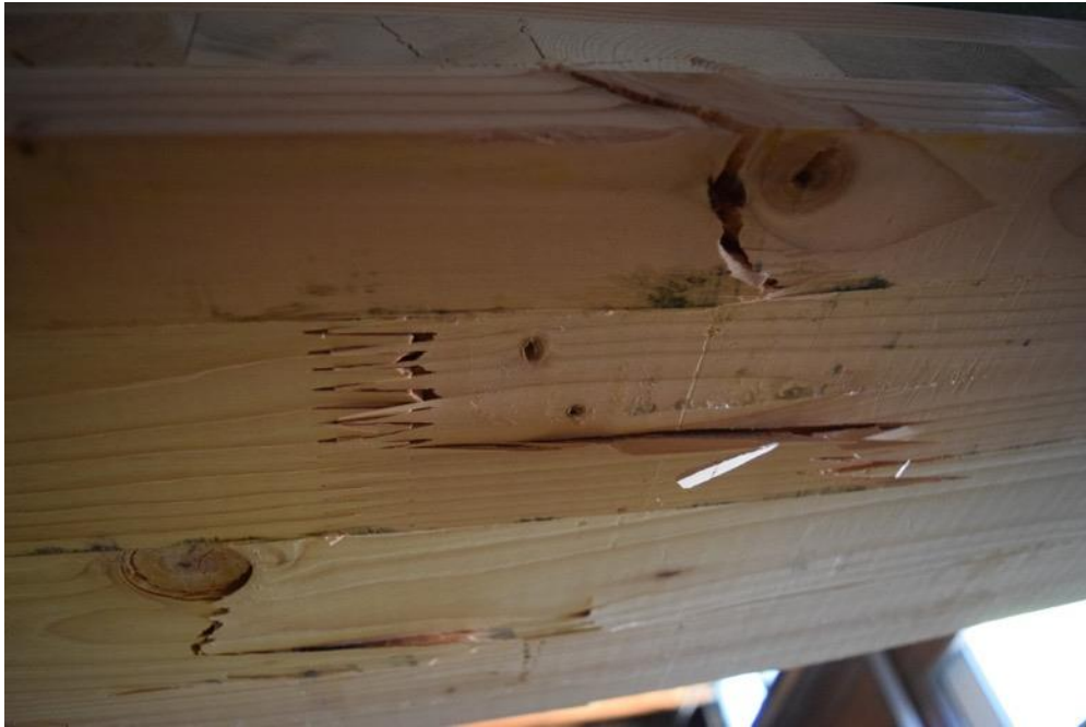
Figure 53: Failure of a 5-ply third-point test specimen at finger joints and knots.
