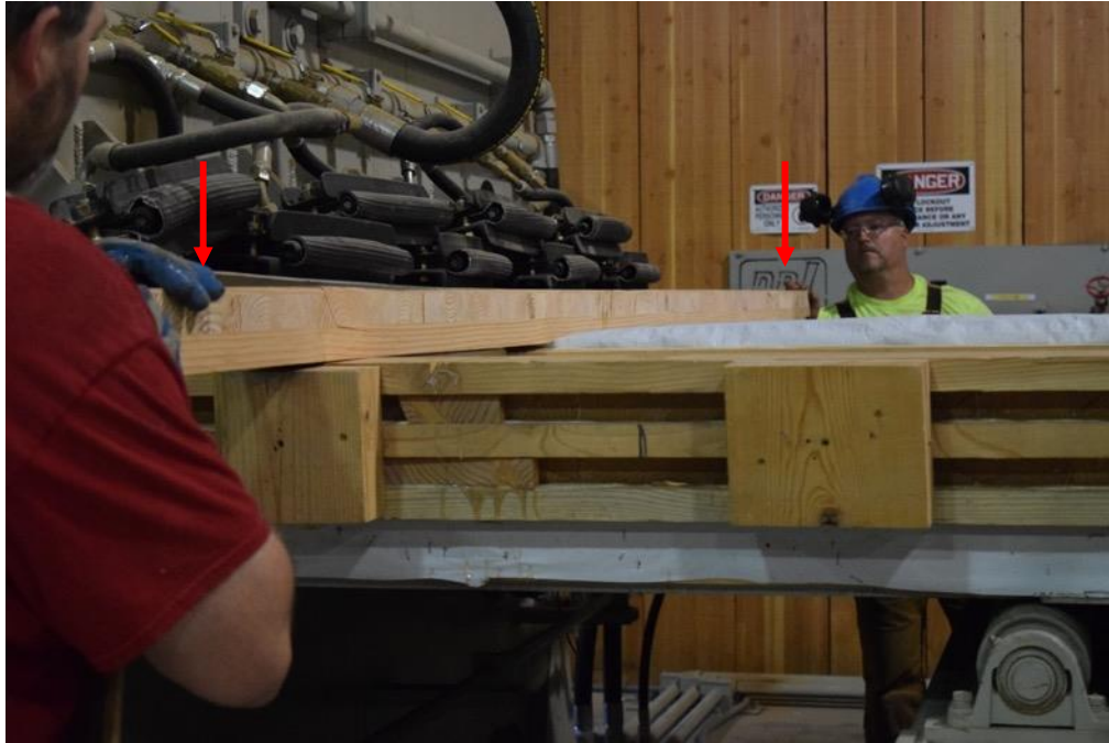
Figure 31: Because of warping, the panels had to be manually pressed down when loaded into the pneumatic press. The arrows indicating the pressure points on the board helping to squeeze the laid-up panel in the press.
