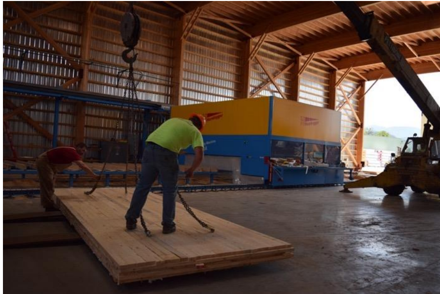
Figure 32: The labor-intensive method used by D.R. Johnson to move the produced panel from the press to their CNC. The panel must be rotated, screws inserted, and the chains adjusted for stability.
