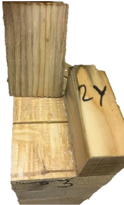
Figure 66: A mixed species sample that resulted in high delamination.
