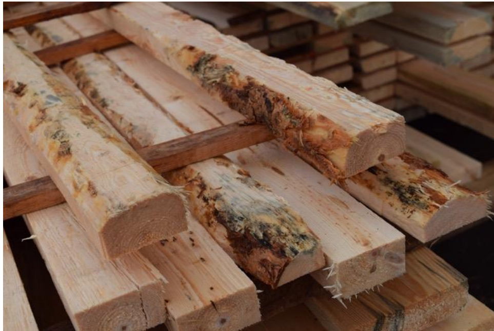
Figure 24: An example of the amount of wane that was present throughout the processed material; this was compatible with the No.2 visual grade.
