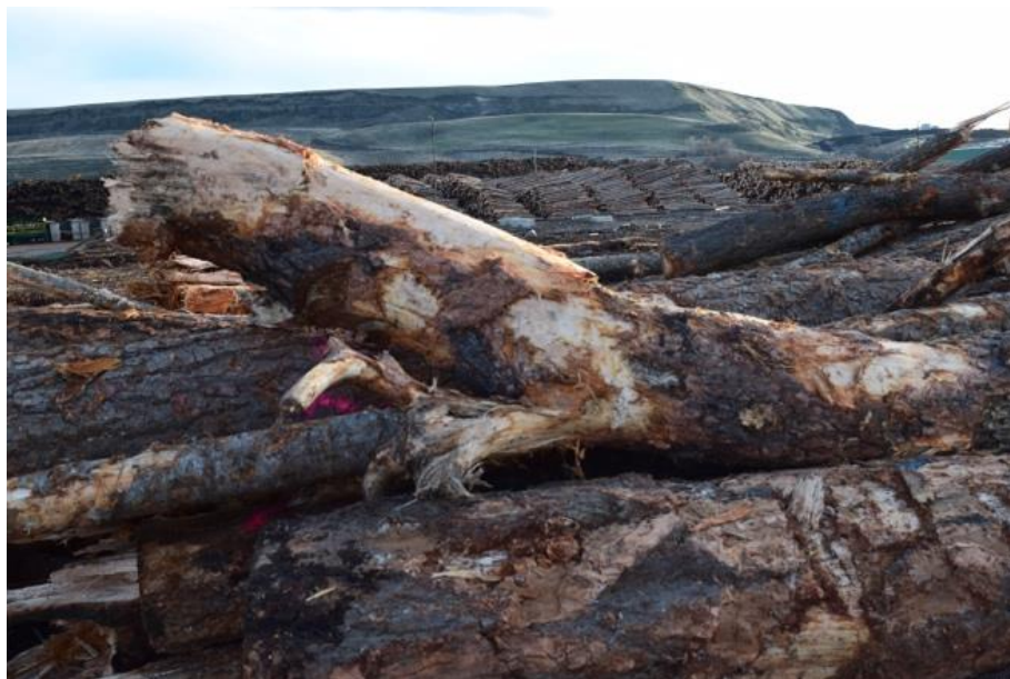
Figure 15: A delivered log to IFG that was rejected due to having too much sweep, or curvature to the log.
