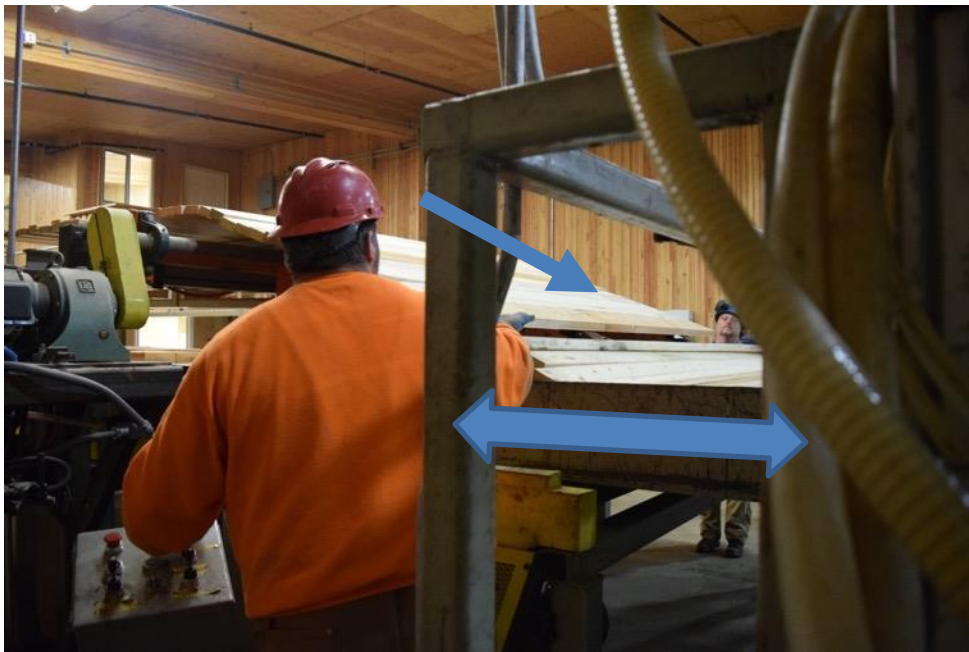
Figure 33: The additional machine that D.R. Johnson used for assistance in the minor direction. This allowed for the lumber to be rolled on top of the previous layer as the staging area for the panel moved back and forth for a quicker and easier layup to help reduce open times.
