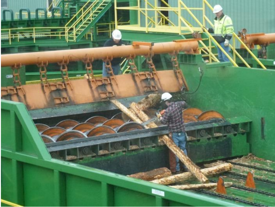
Figure 18: Difficulties during the breakdown process. During the processing the material was rotated, causing it to get caught in the machinery and needing it to be removed. This occurred multiple times.
