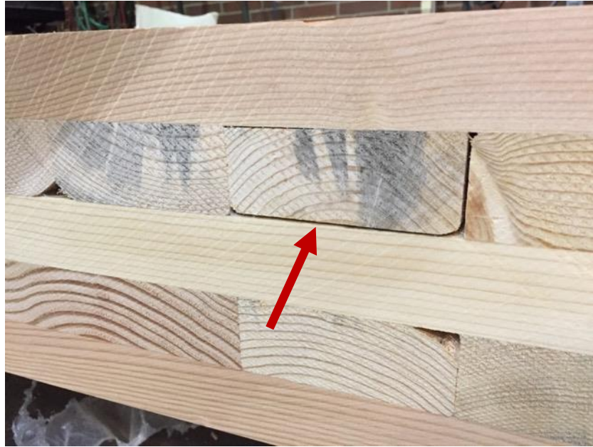
Figure 34: Due to bow and twist, when sent through the planer, the lumber becomes too thin for panel production and/or a sufficient bondline.
