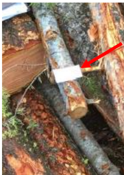
Figure 15: A delivered log to IFG that was rejected due to having too much sweep, or curvature to the log.
