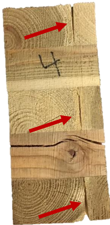
Figure 65: Cyclic delamination sample showing un-bonded edges that caused very little to no delamination on the bonded faces.
