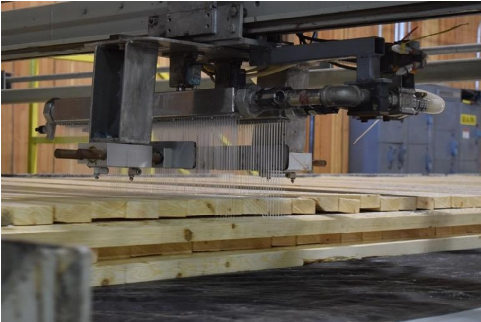
Figure 27: Panel glue spread setup. The glue head moves along the minor direction of the panels lay-up, while the table, on which the panels are laid-up, moves in the major direction. The hardener and MF glue are kept separately and roll together when placed under pressure in the press.
