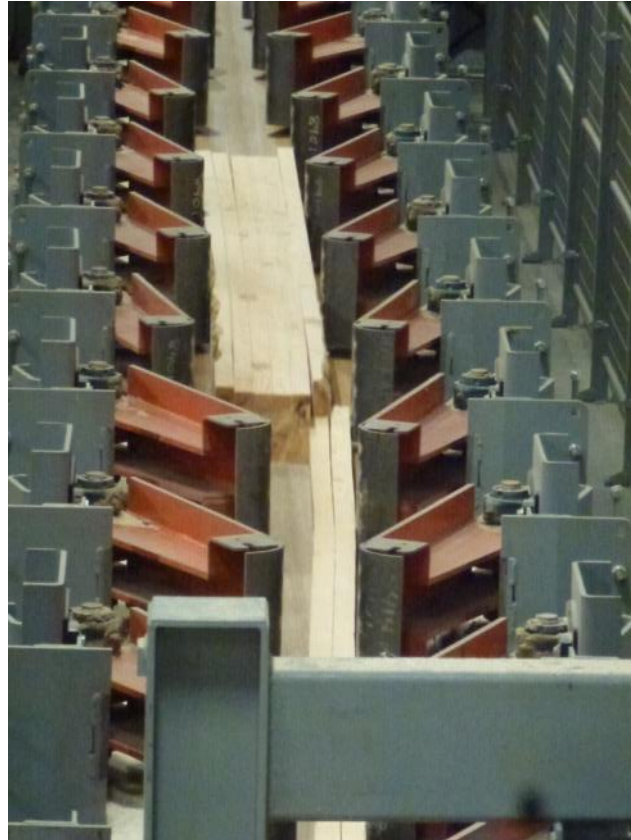
Figure 20: A sawn pieces still traveling together, past the first gang saw unit, got jammed on the conveyor.
