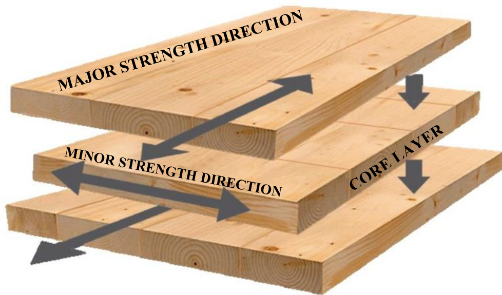
Figure 1: Example of the standard cross laminated timber lay-up. (Laguarda Mallo and Espinoza 2015)
