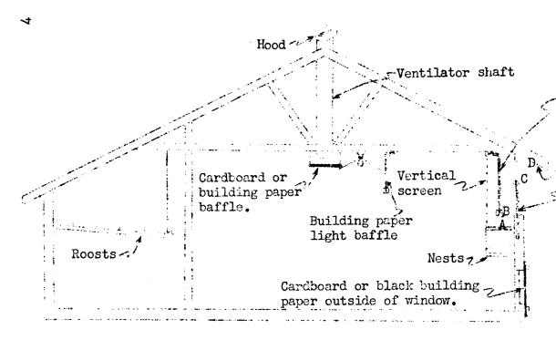
Figure 1 - Section of O. S. C. Type Laying House having vertical guard screen over the nests.
