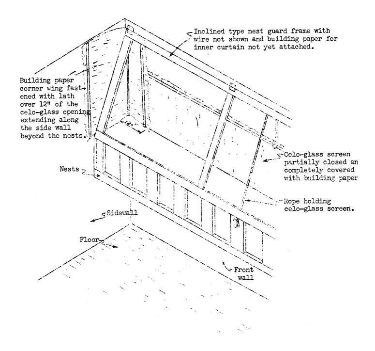
Figure 3 - Detail showing method of installing corner wing or baffle to prevent light leaks around ends of inner curtain.
