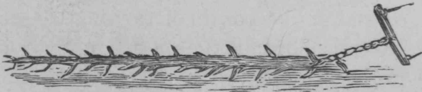
Fig. 142.—A STIRRER MADE OF A CEDAR STEM.
