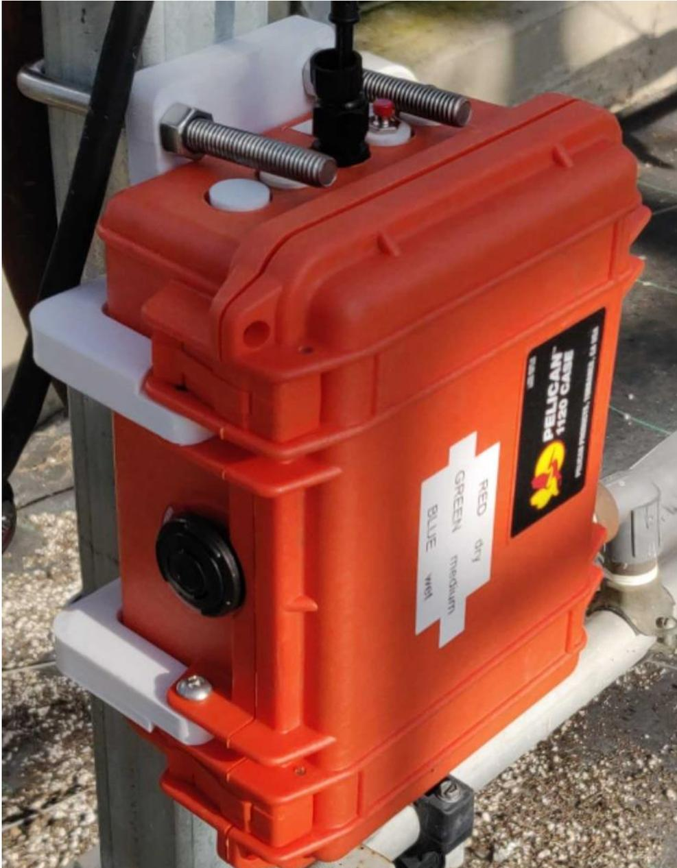
Figure 10. The water-resistance pelican case containing the onboard electronics and custom 3D printed irrigation mounting system (in white).
