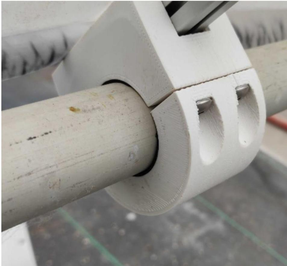
Figure 9. The irrigation boom 3D Printed mount implementation with rubber tape.
