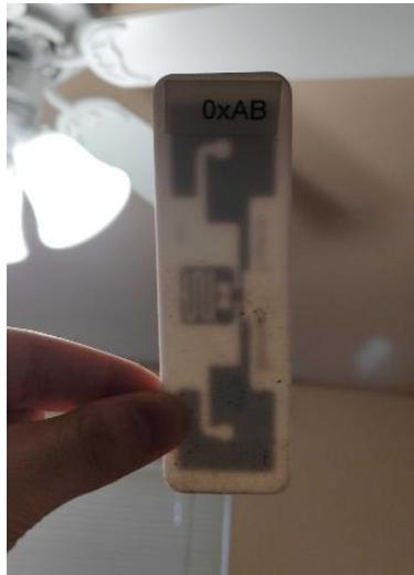
Figure 6. SmarTrac RFID Tag encased in the 3D Printed case.
