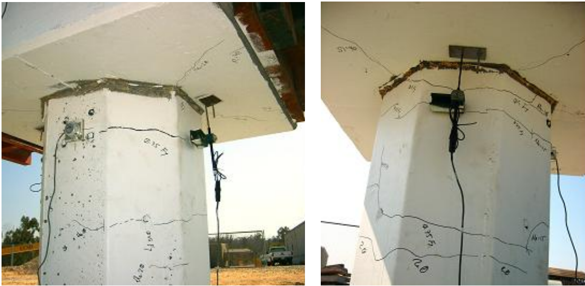
Figure 4-44 Cracks on P2 and P4 for loading Cycle 6 (System Test 2)
