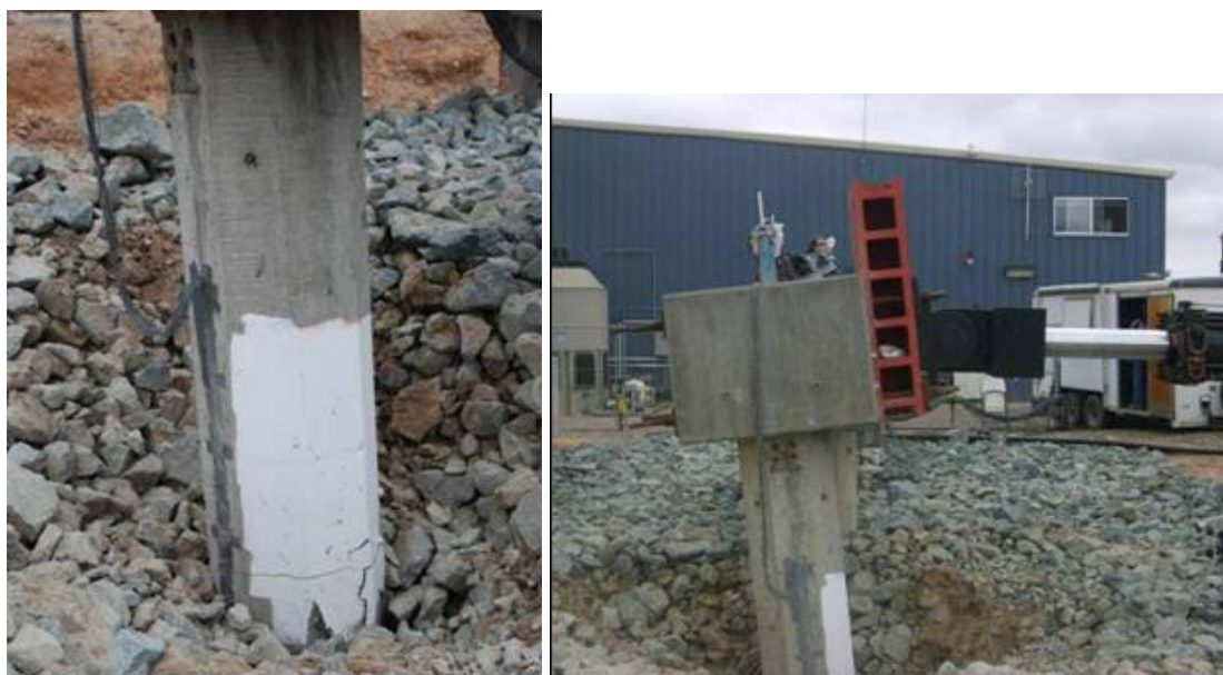
Figure 4-11 Deformed test pile after all the loading (Single Pile Test 2)
