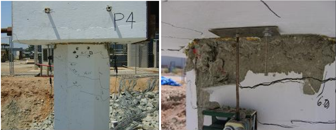
Figure 4-46 Spalling at connection of P4 at Cycle 10 (System Test 2)
