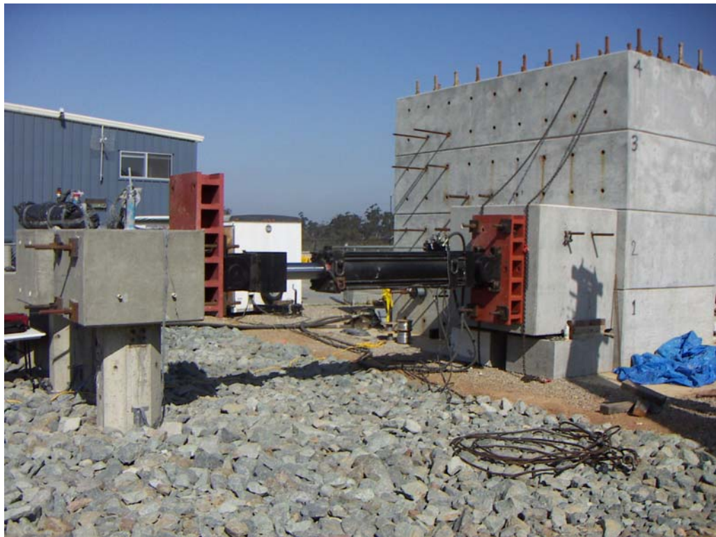
Figure 3-45 Aspect of test setup for Single Pile Test
