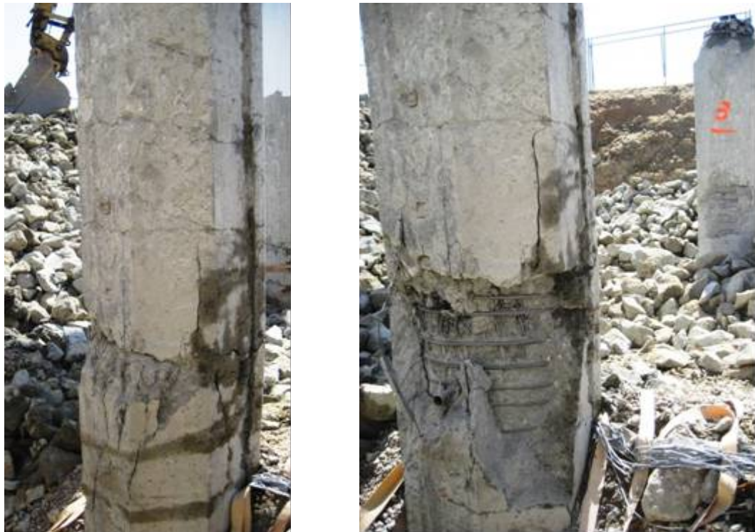
Figure 4-40 Plastic hinge (System Test 1, P3)
