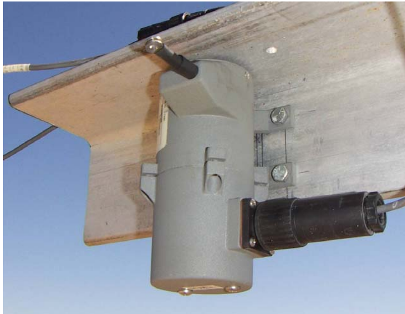
Figure 3-68 String-activated linear potentiometer
