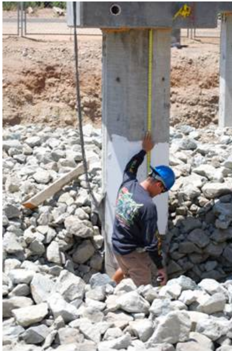
Figure 4-18 General view after excavation to 3ft below ground surface (Single Pile Test 2)
