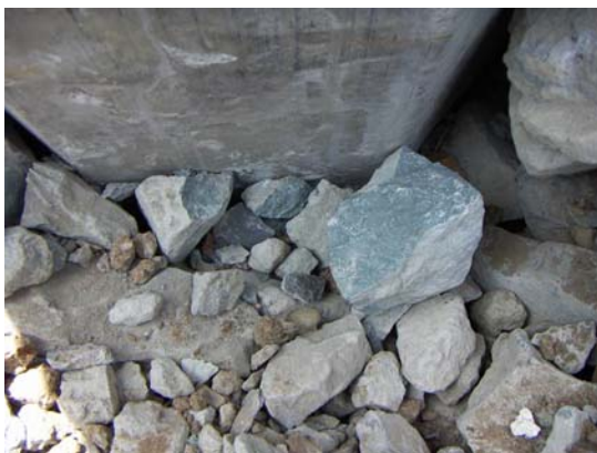
(a) Fractured rocks, shows interlocking
