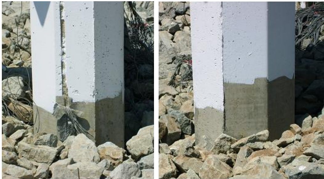
Figure 4-45 Settlement of rockfill around P2 and P4 after Cycle 8 (System Test 2)
