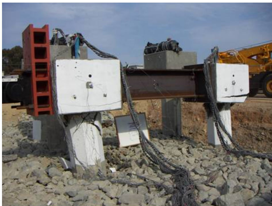
Figure 4-24 Deformed piles after the final loading (System Test 1)
