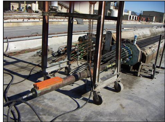
(b) Applying prestressing force on the strands
