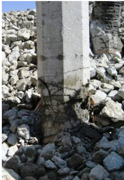
Figure 4-60 Plastic hinge on the north side (System Test 2, P2)
