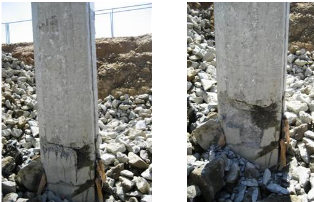
Figure 4-62 Plastic hinge on the north side (System Test 2, P4)
