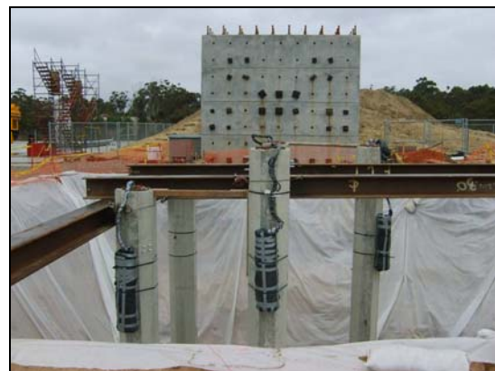
(j) Installed piles fixed to the beam
