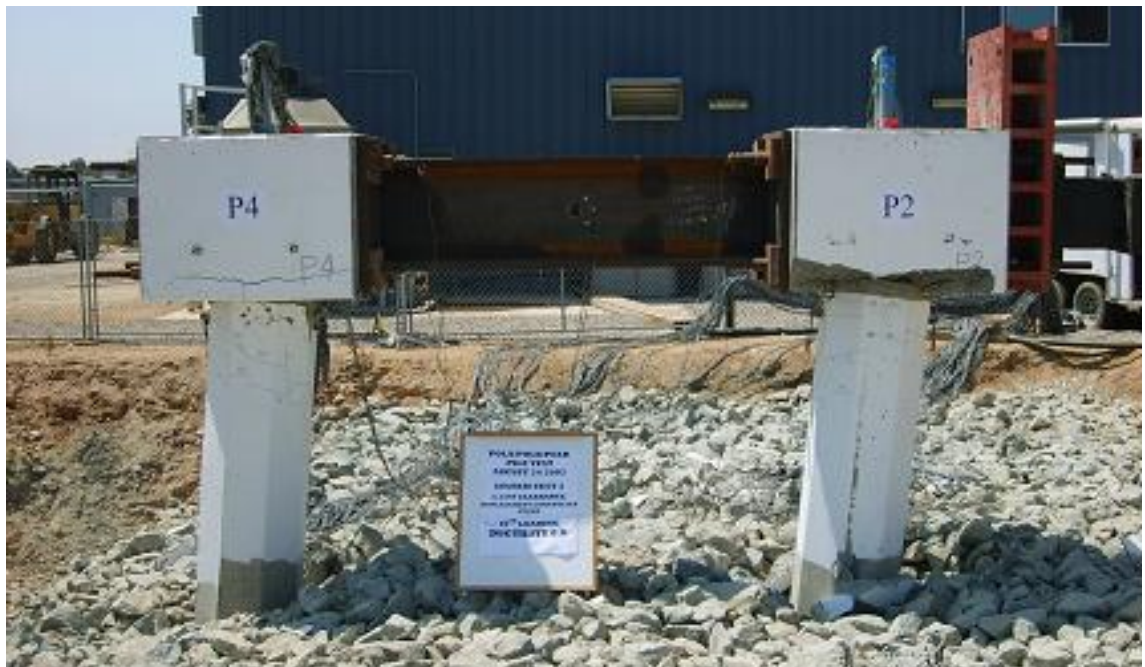
Figure 4-47 Deformed test piles after the final loading Cycle 11 (System Test 2)
