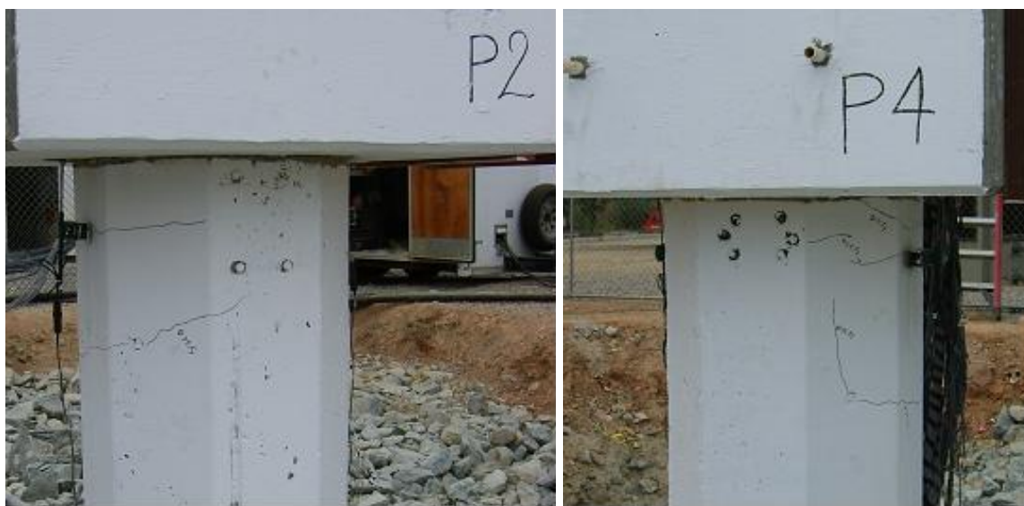
Figure 4-43 Cracks on P2 and P4 for loading Cycles 1 to 3 (System Test 2)
