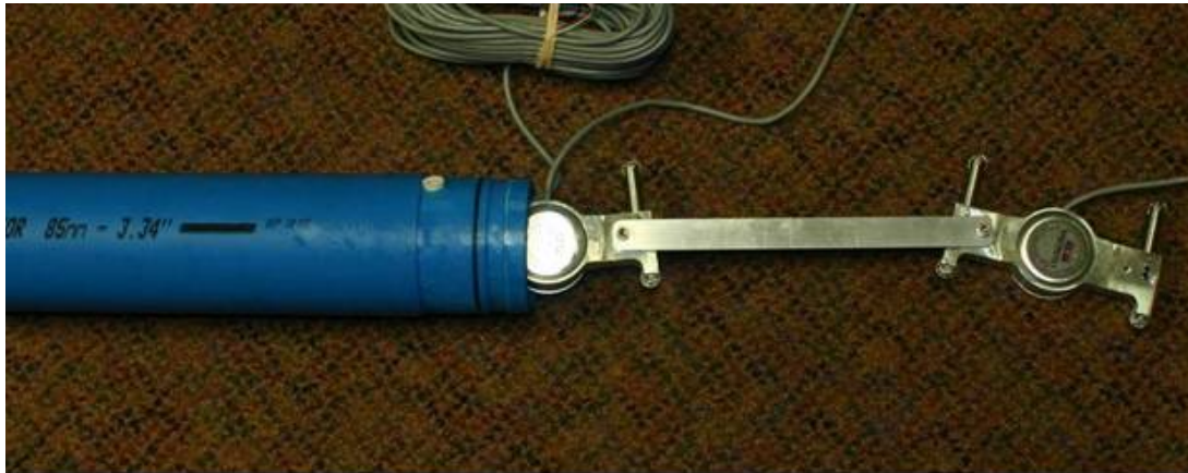
Figure 3-60 Installation of a series of tiltmeters through inclinometer casing
