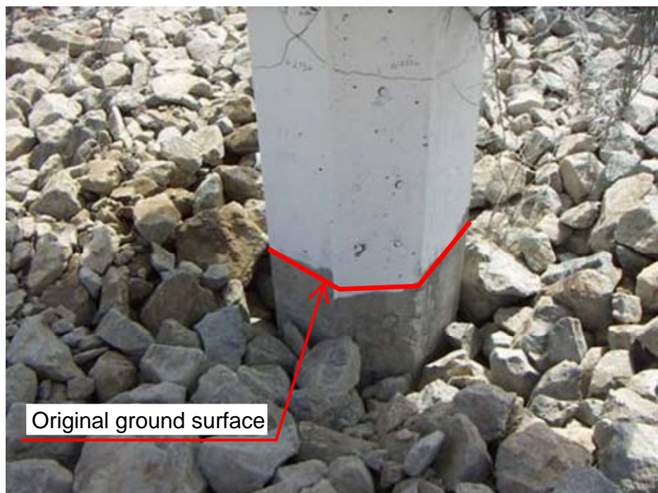
Figure 4-23 Settlement around the test pile (System Test 1)
