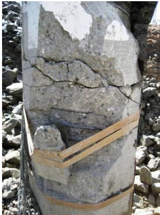
Figure 4-19 Exposed in-ground plastic hinge on the north side of the pile (Single Pile Test 2)
