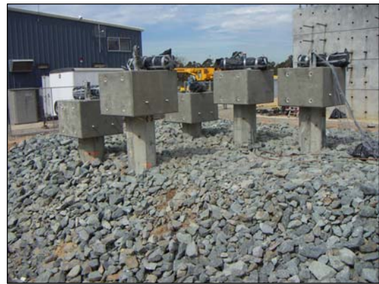
(j) Completed making load stubs
