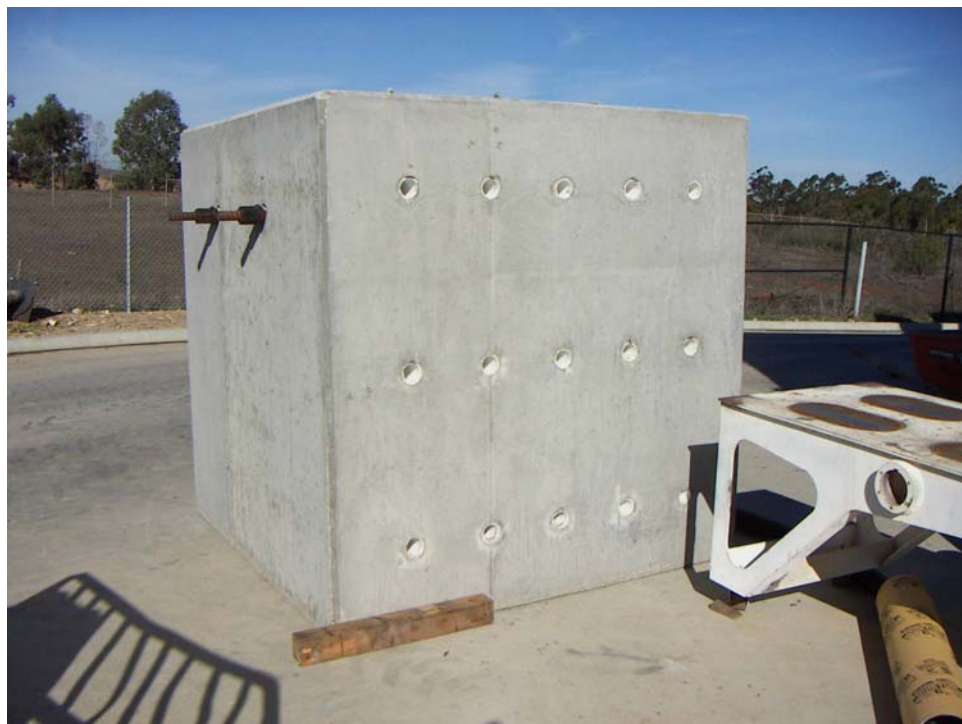
Figure 3-41 Concrete spacer block
