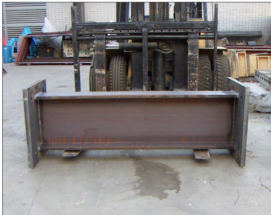
Figure 3-43 Steel beam connecting test piles (before instrumentation)
