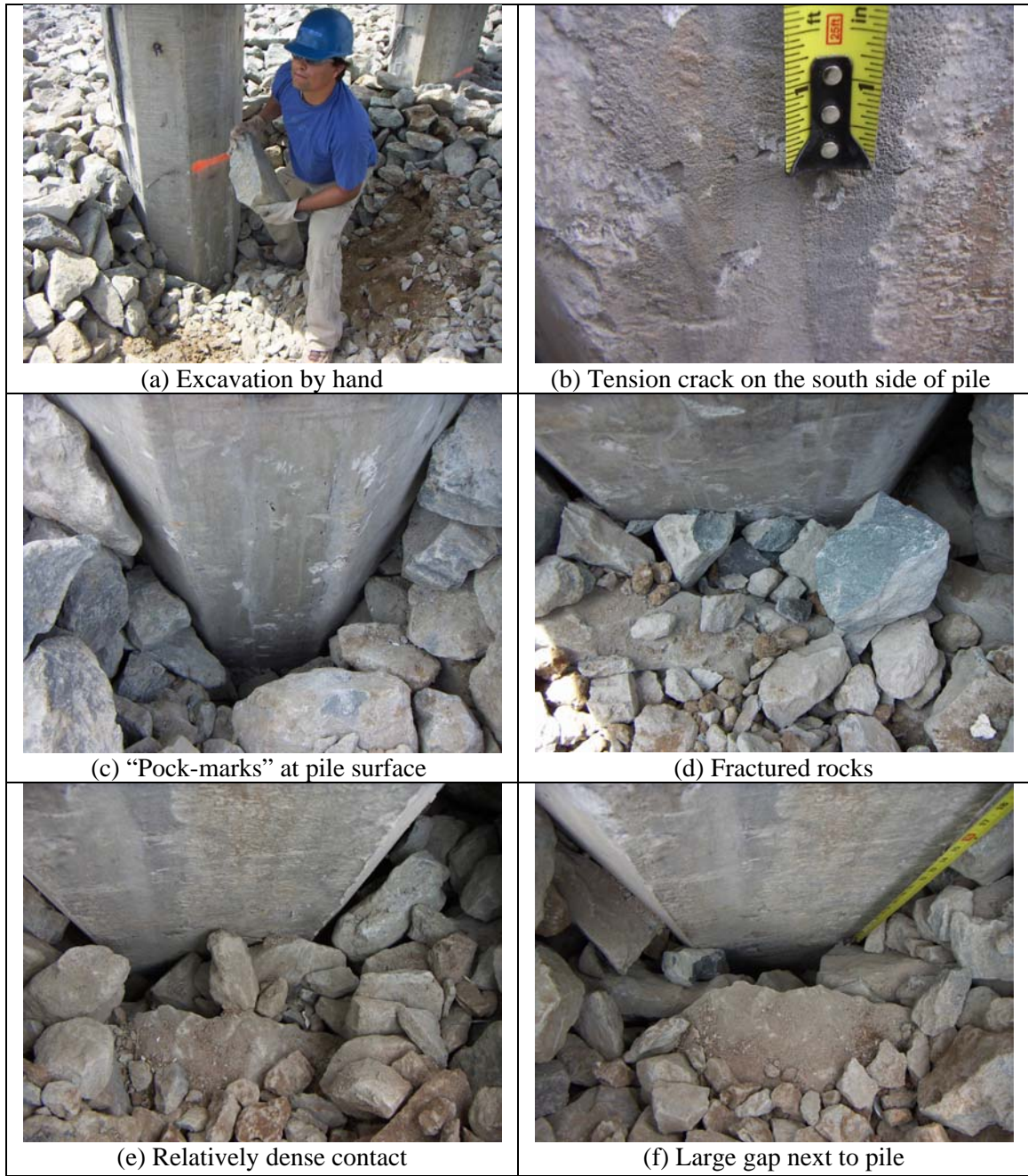
Figure 4-8 Visual inspection of in-ground parts of test pile (Single Pile Test 1)
