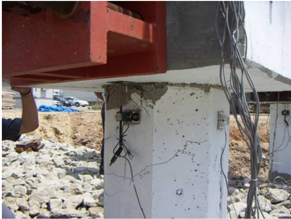
Figure 4-22 Concrete crushing during Cycle 8 at P3 (System Test 1)
