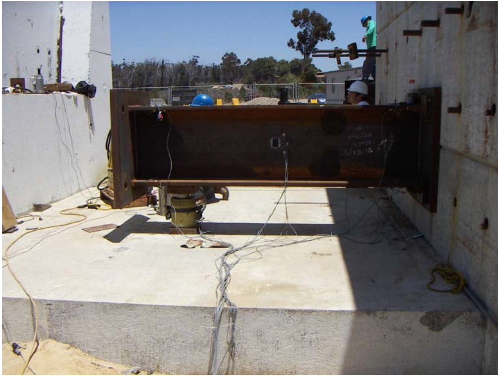
Figure 3-74 Aspect of test setup for calibration of the steel beam
