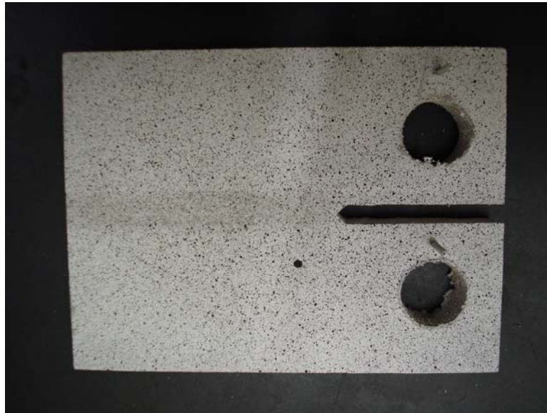
Figure 15. Specimen with random speckle pattern
