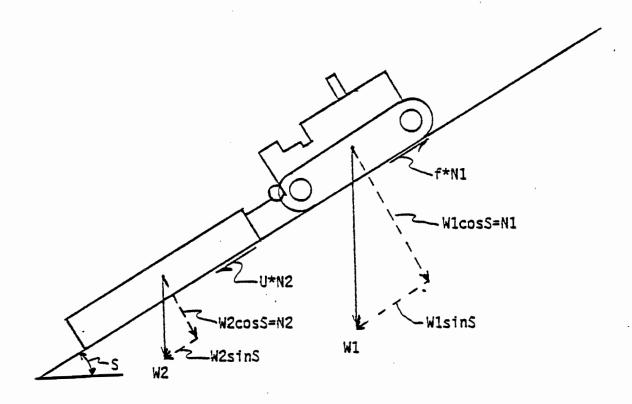
Figure B3. Diagram of the forces acting on the conventional tracked skidder.
