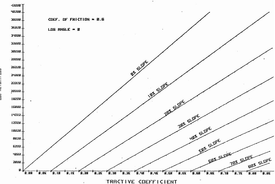
Figure 25. Graph of tractive coefficient and log weight for various slopes(conventional skidder, D-7 Cat
