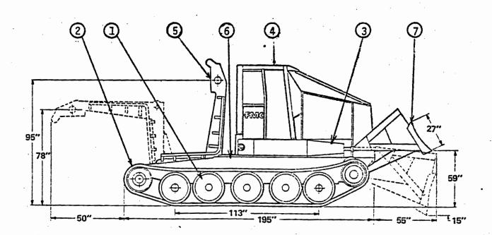
The general arrangement consists of a running gear with forged steel track and torsion bar suspension, with the suspension mounted to a steel unitized lower chassis structure. The suspension consists of ten sets of dual road-wheels, five per side, mounted on rear facing roadarms. Each roadwheel and arm assembly is free to flex or move up and down using a torsion bar.
