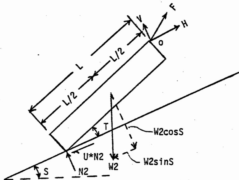
Figure B2. Free-body diagram of the forces acting on the log.
