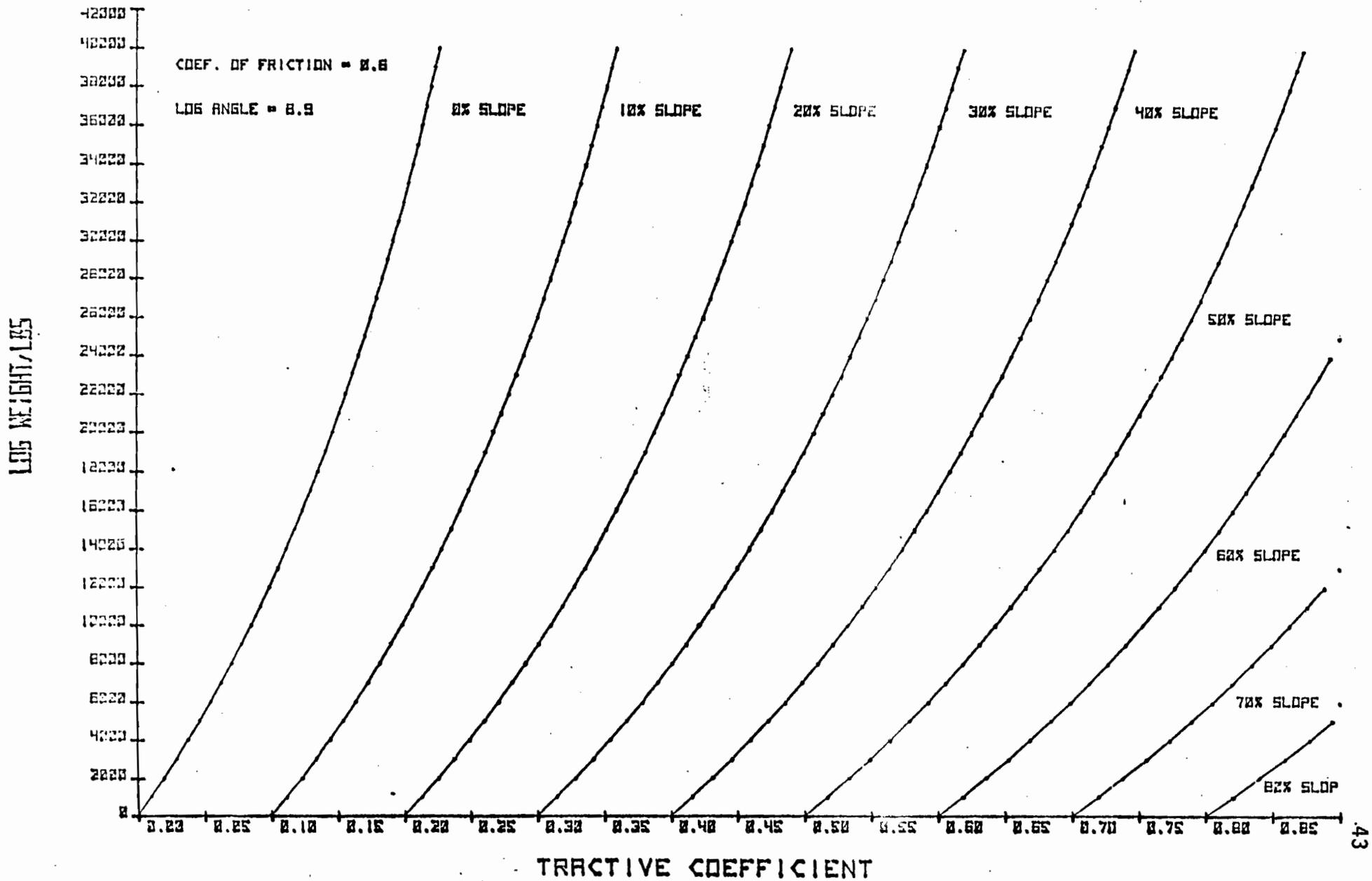
Figure 24. Graph of tractive coefficient and log weight for various slopes(FMC skidder).
