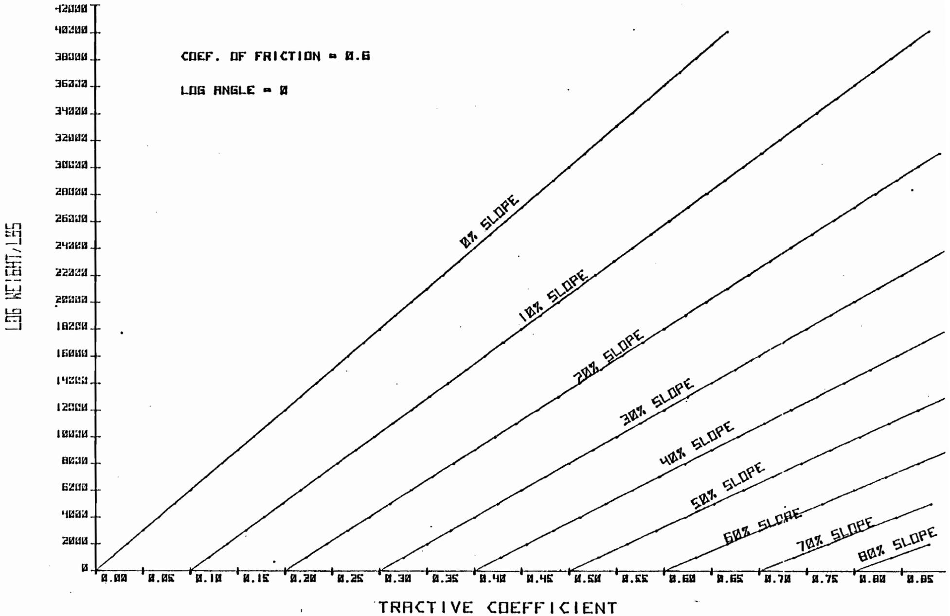
Figure 25. Graph of tractive coefficient and log weight for various slopes (conventional skidder, D-7 Cat)
