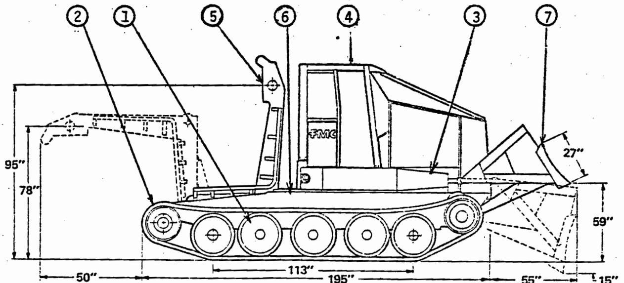
The general arrangement consists of a running gear with forged steel track and torsion bar suspension, with the suspension mounted to a steel unitized lower chassis structure. The suspension consists of ten sets of dual road-wheels, five per side, mounted on rear facing roadarms. Each roadwheel and arm assembly is free to flex or move up and down using a torsion bar.
