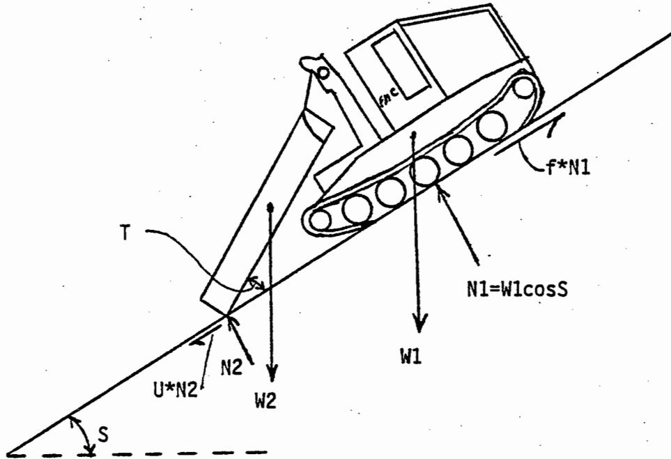
Figure B1. Diagram of the forces acting on the FMC skidder.
