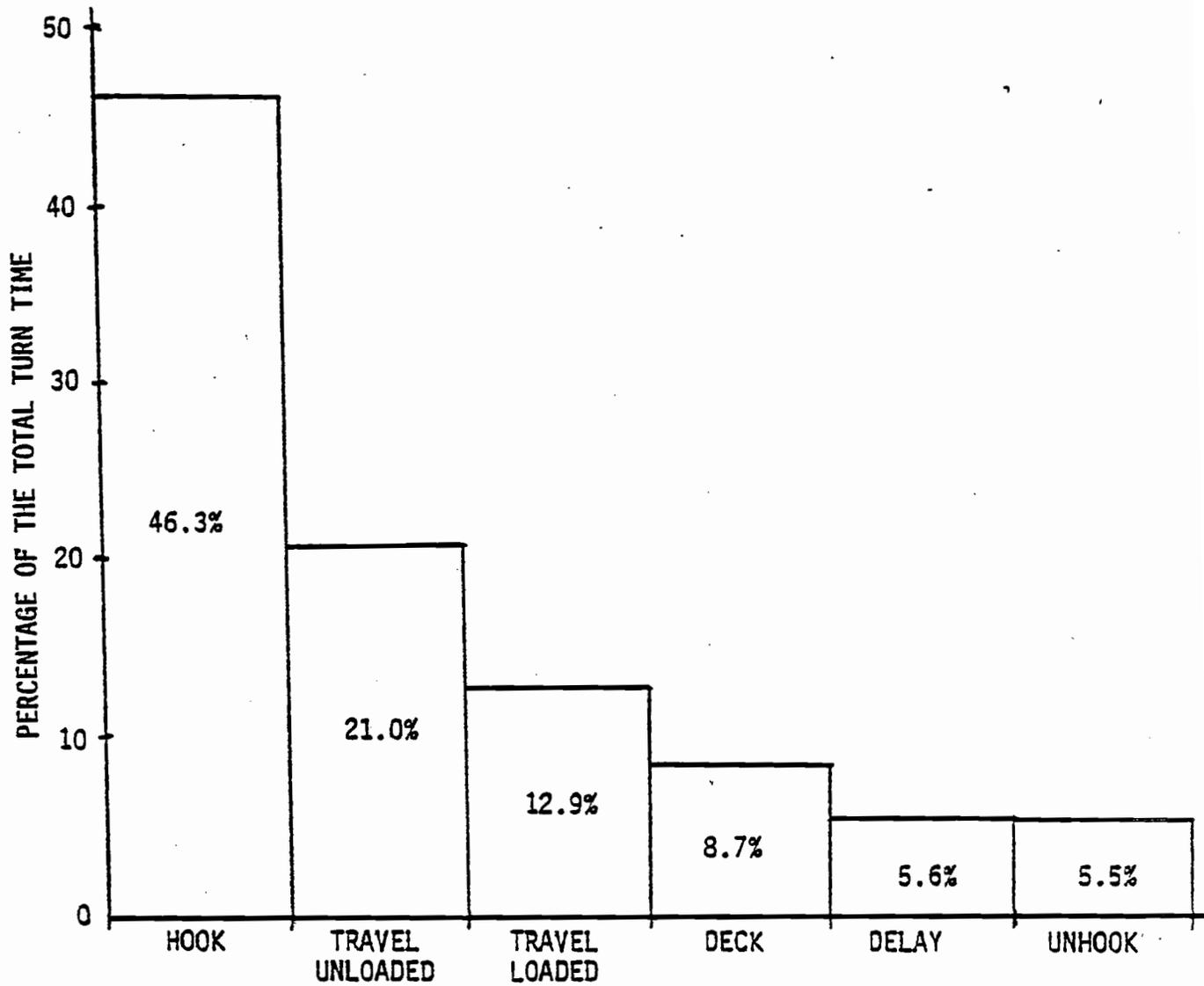
Figure 5. Bar graph of the individual elements of the turn shown as a percentage of the total turn time. (combined units)
