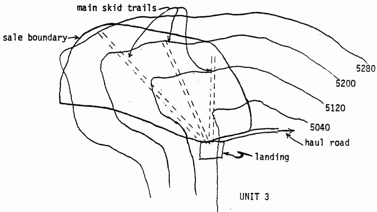
Figure 2. Map of units 3 and 4 of the sale area showing skid trail layout. (not to scale)
