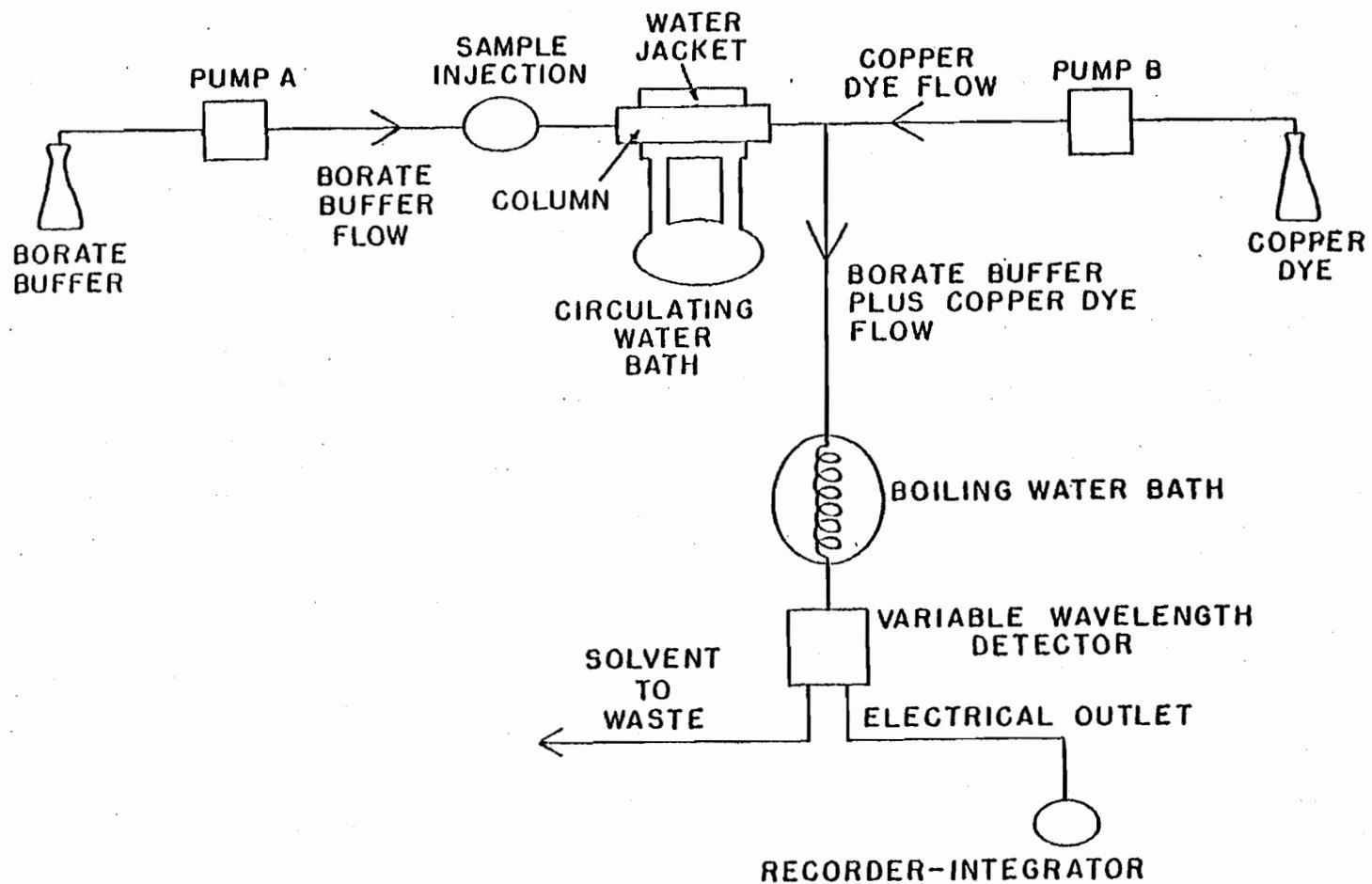
Figure 8. Schematic diagram of the apparatus used for carbohydrate analyses.
