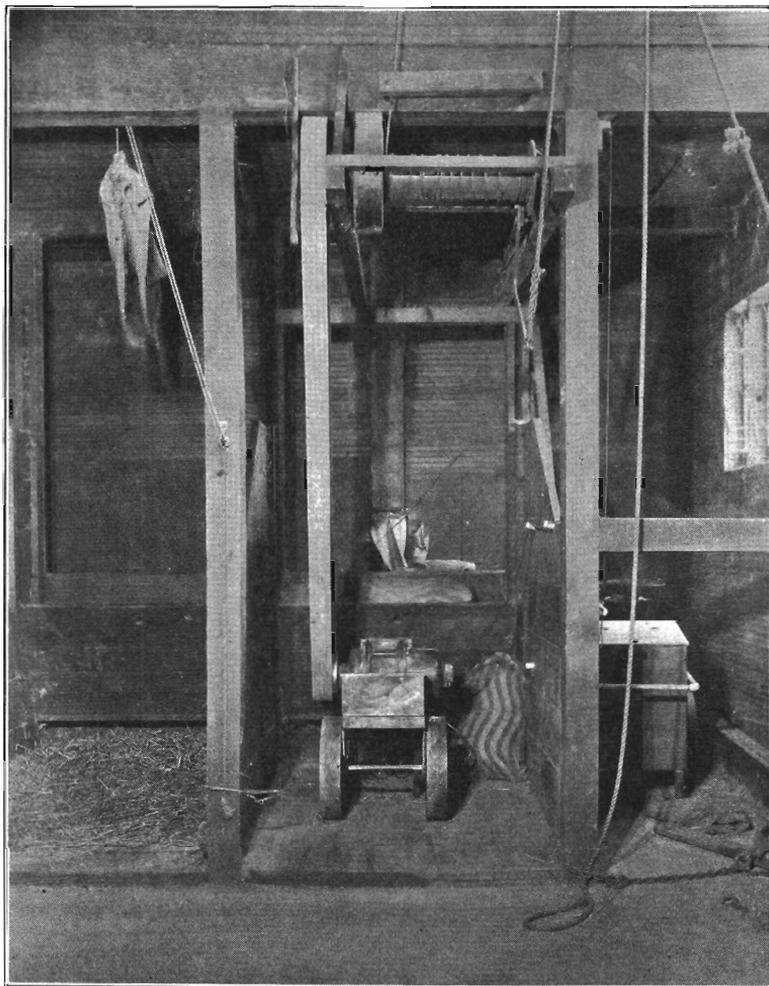
Fig. 5. The internal gear hoist showing single lever control attached to a rope which runs through a pulley near the top of the barn and returns to the operator on the wagon which is located in the driveway in front of the hoist.
