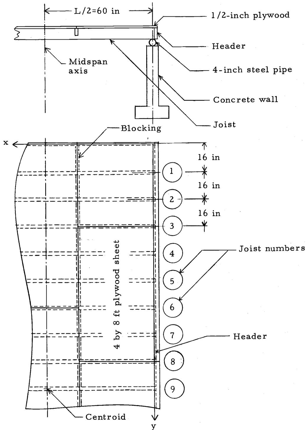
Figure 4.5. Arrangement of experimental wood-joist floor.
