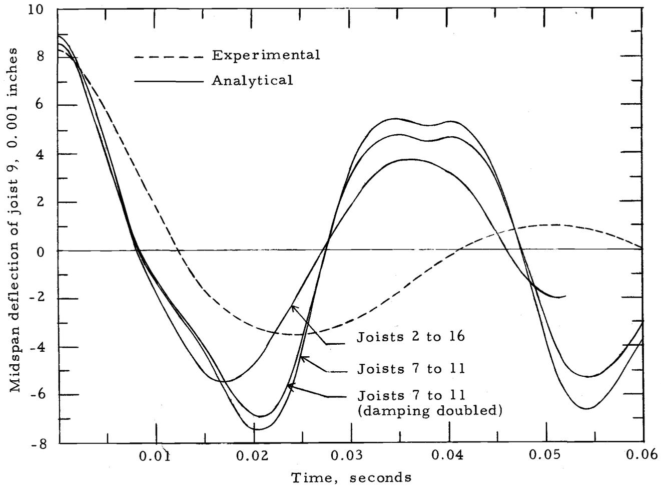
Figure 4.8. Dynamic response of a floor to initial displacements.
