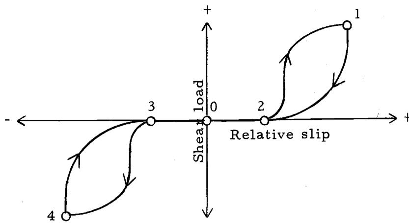
Figure 4.9. Cyclic load-slip curve of nailed plywood-joist connection.
