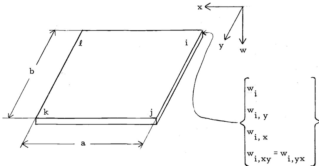
(a) Finite element and nodal displacements.
