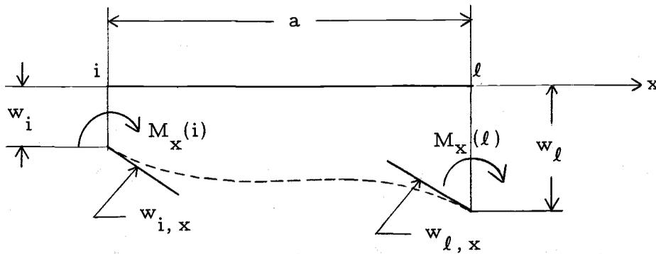
Figure 2.5. Composite T-beam bending element.
