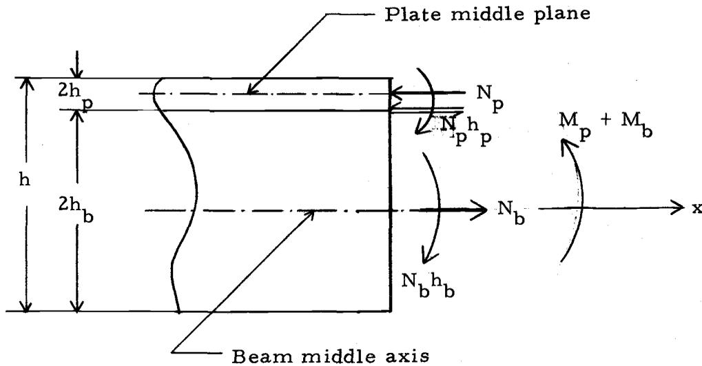
Figure 2.3. Forces on the composite beam element.
