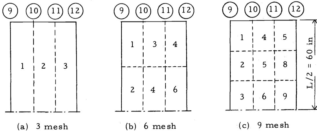
Figure 4.10. Finite element mesh of a floor with four joists.
