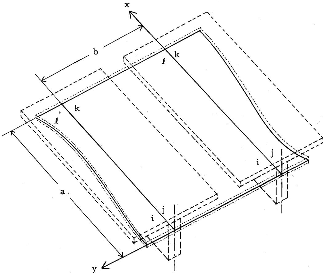
Figure 3.1. The floor model and the assembly of the plate and beam elements.
