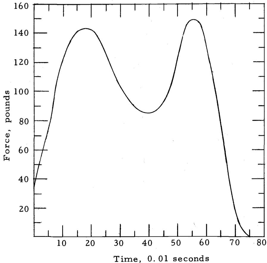
Figure 3.2. Forcing function for the human foot during walking.
