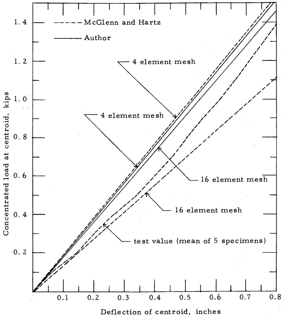
Figure 4.2. Deflection of a square orthotropic plate clamped along four edges.
