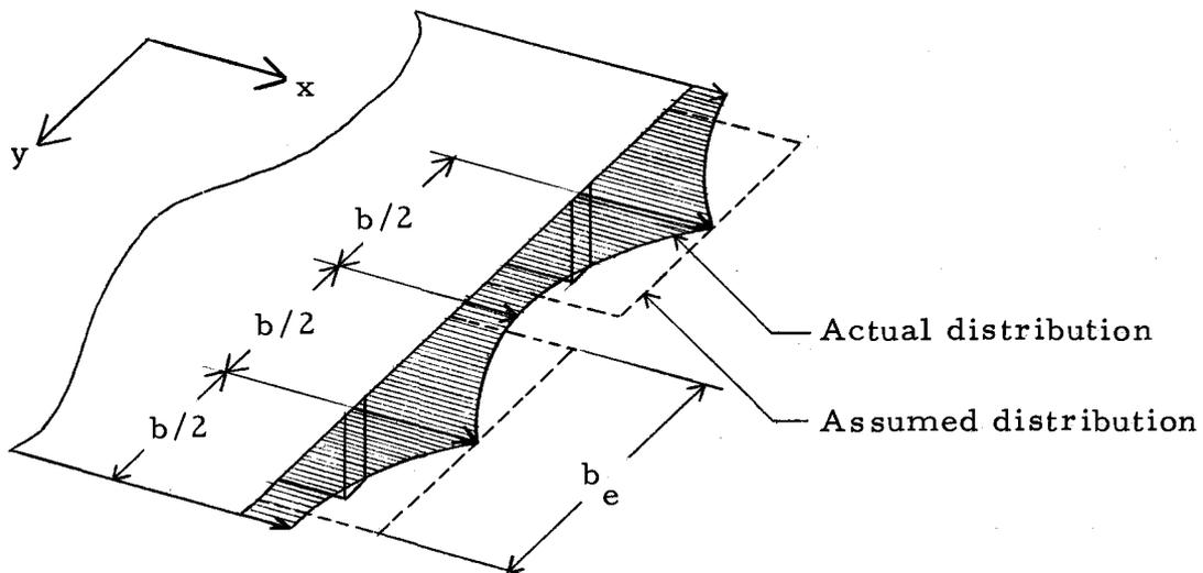
Figure 2.4. Distribution of membrane forces in the floor covering.
