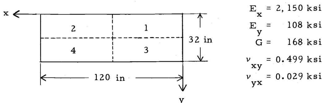
Figure 4.4. Rectangular plywood plate simply supported along all four edges.
