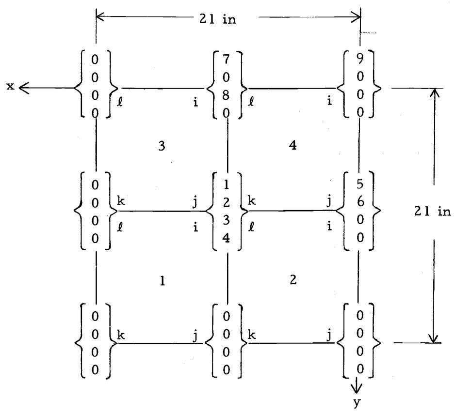
(b) Nodal displacement numbers for 4 element mesh.
