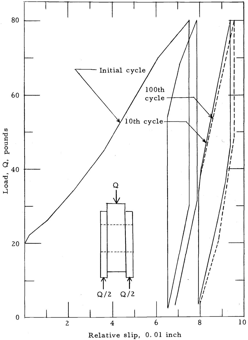
Figure 2.2. Cyclic load diagram of nailed shear specimen.
