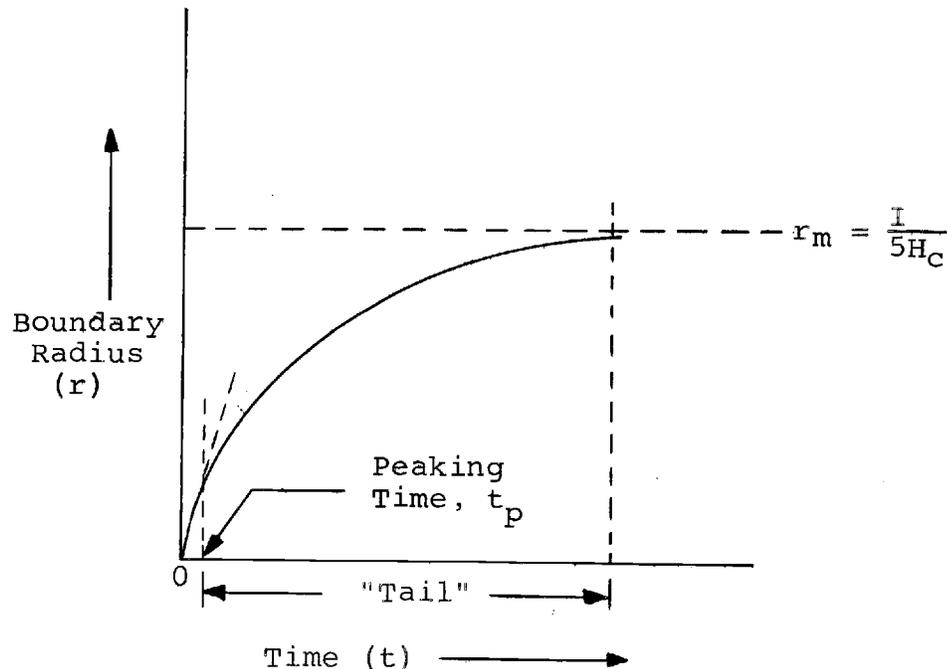
Figure 7. Penetration of flux reversal in term of boundary radius ( $r$ ), as function of time ( $t$ ).
