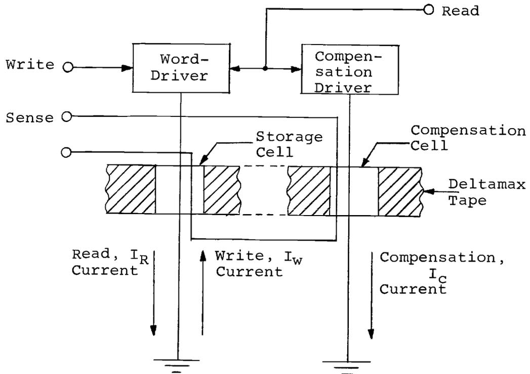
Figure 9. System diagram of the compensated, apertured Deltamax memory cell.
