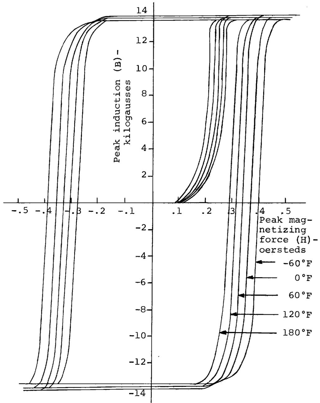
Figure 32. Effect of temperature on the dynamic magnetization loop of Deltamax at 60 cycles A.C.
