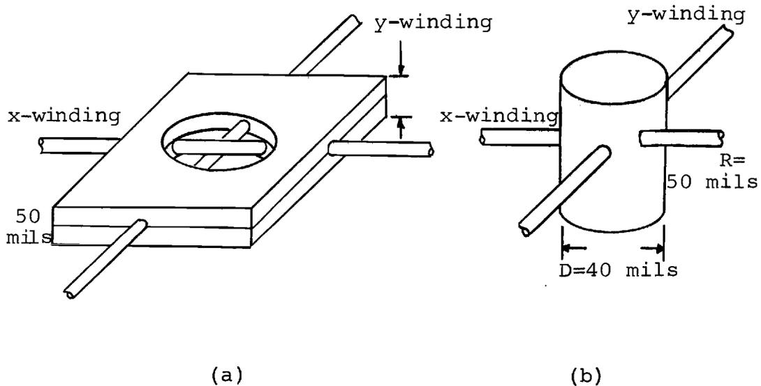
Figure 24. Structure of type III element.
