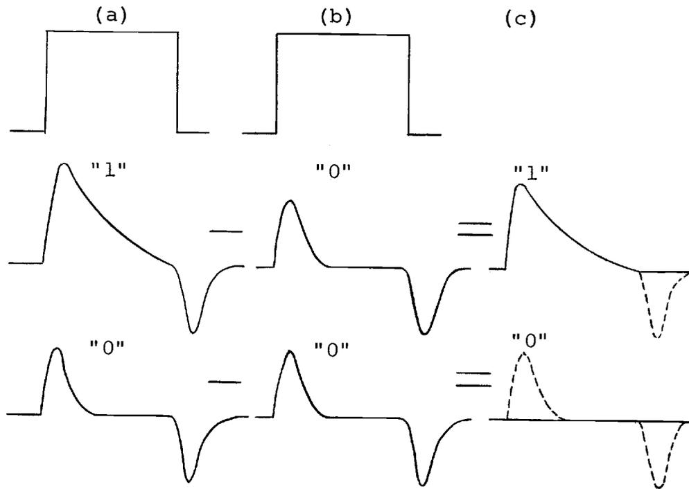
Figure 10. Principle of ideal compensation.
