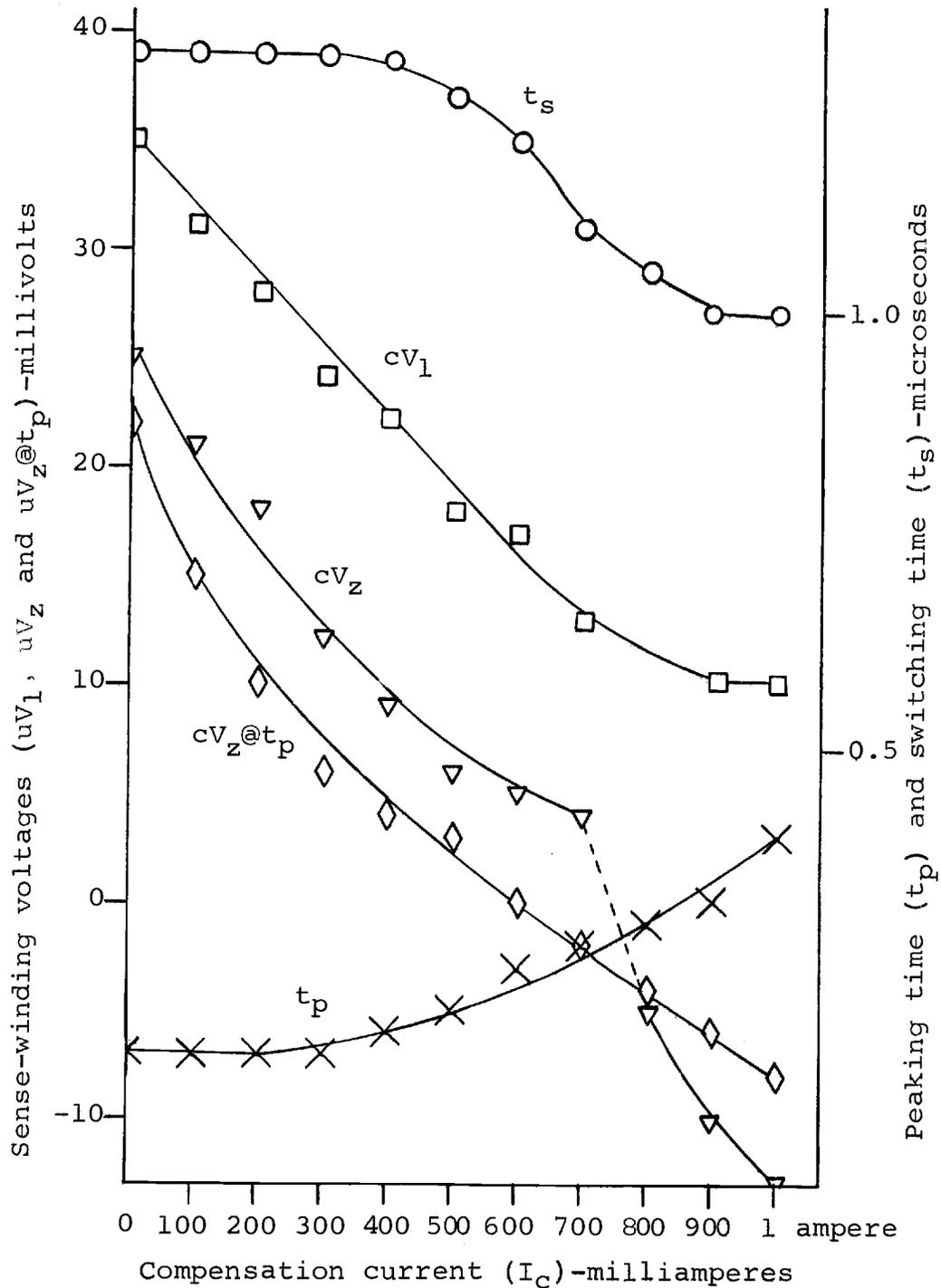
Figure 16. Typical characteristics for the compensated, apertured Deltamax memory cell with a read current pulse of 800 milliamperes. (See Table IV, Appendix VI, for test conditions)
