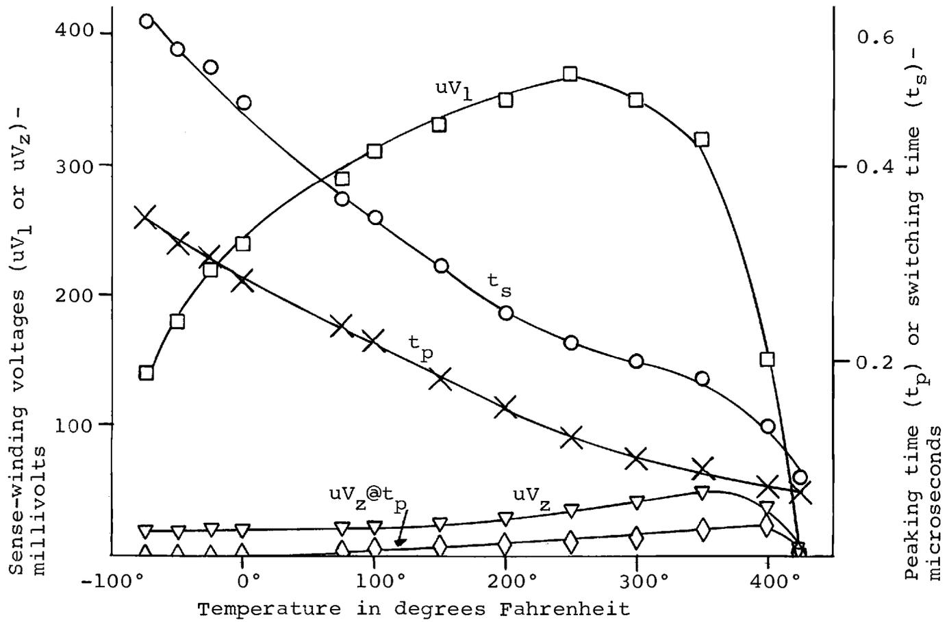
Figure 21. Temperature effect on the RCA Type 226M1 ferrite core.
