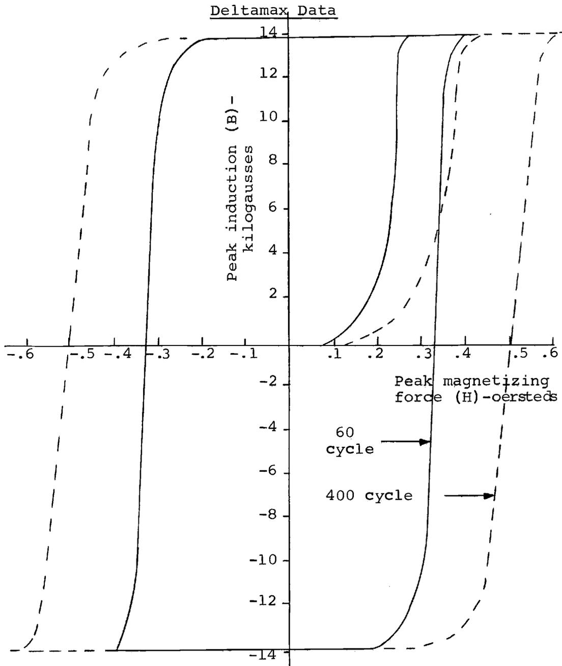
Figure 31. Dynamic magnetization loops of Deltamax.
