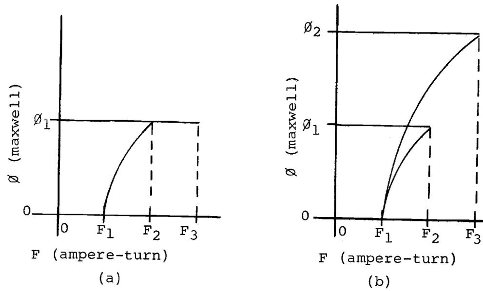
Figure 2. Initial magnetizing characteristic.
