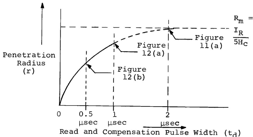
Figure 13. Principle of speed improvement.
