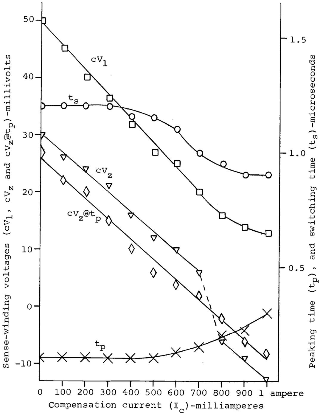
Figure 15. Typical characteristics of compensated, apertured Deltamax memory cell with a read current pulse of one ampere. (See Table III, Appendix VI for test conditions)
