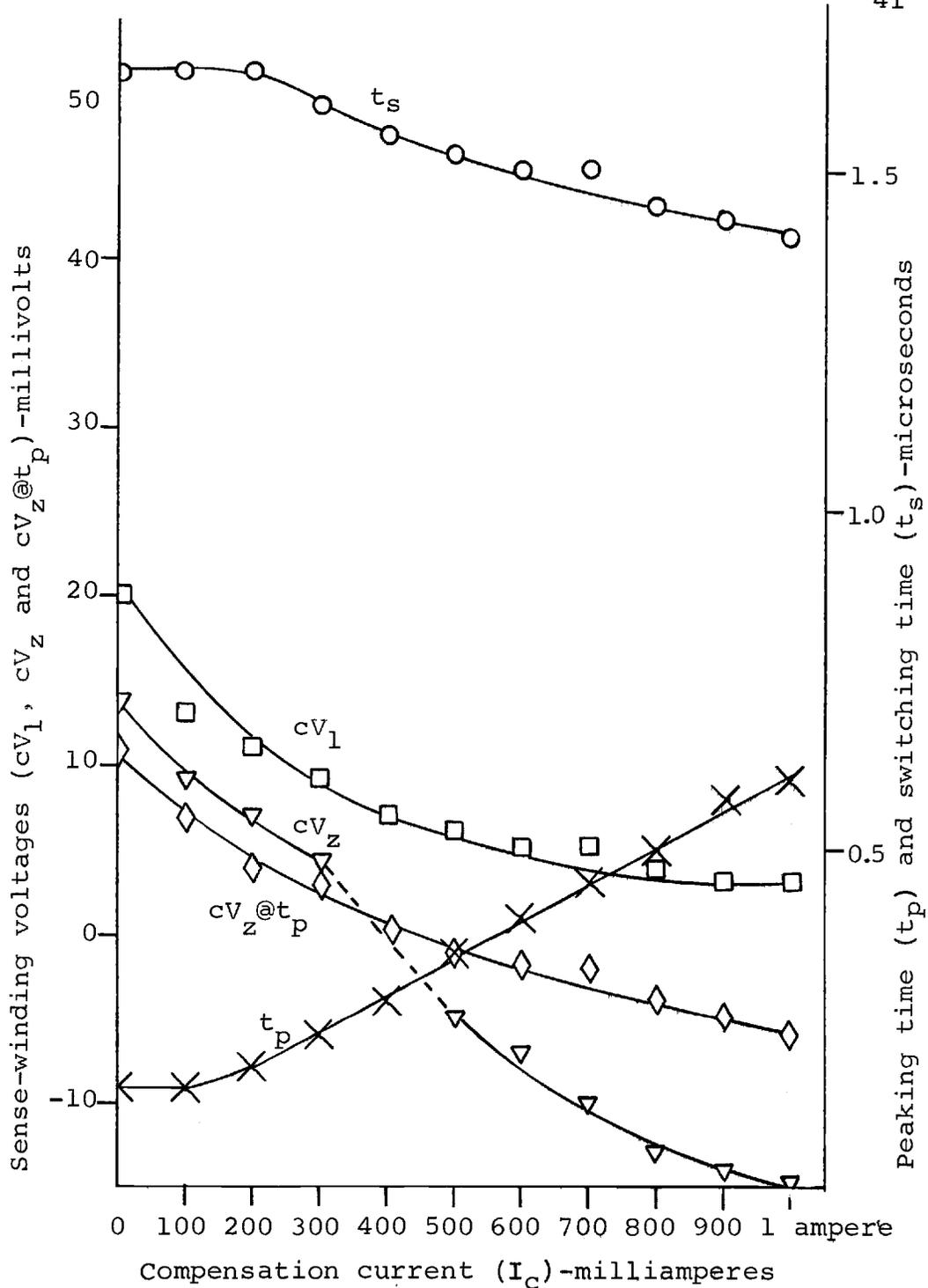
Figure 17. Typical characteristics of compensated, apertured Deltamax memory cell with a read current pulse of 500 milliamperes. (See Table V, Appendix VI for test conditions)
