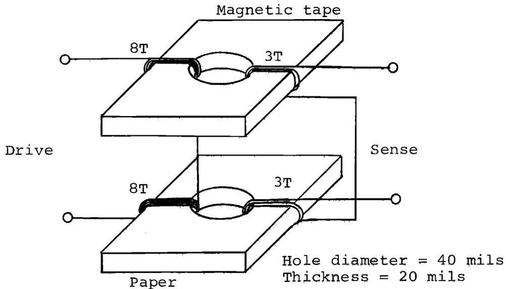
Figure 22. Type II element system diagram.
