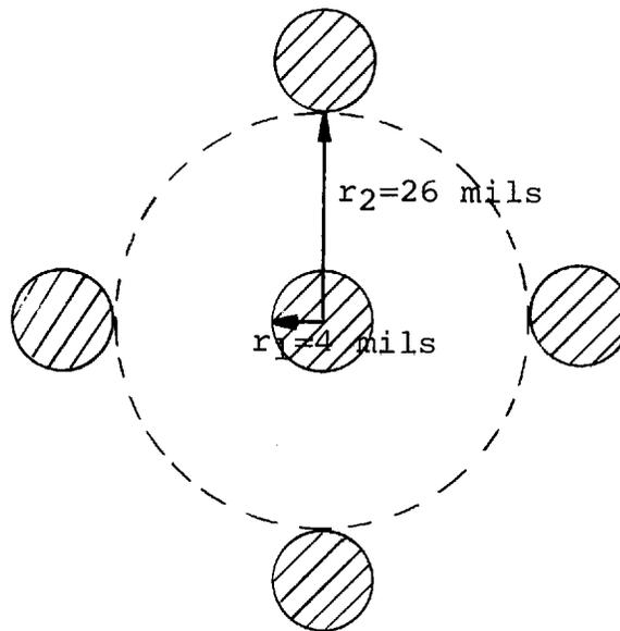
Figure 4. Geometry of type I element (apertured Deltamax memory cell).
