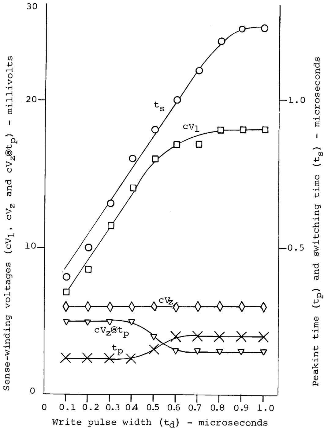
Figure 19. Variation of the typical characteristics for the compensated, apertured Deltamax memory cell with write pulse width ( $t_d$ ).
