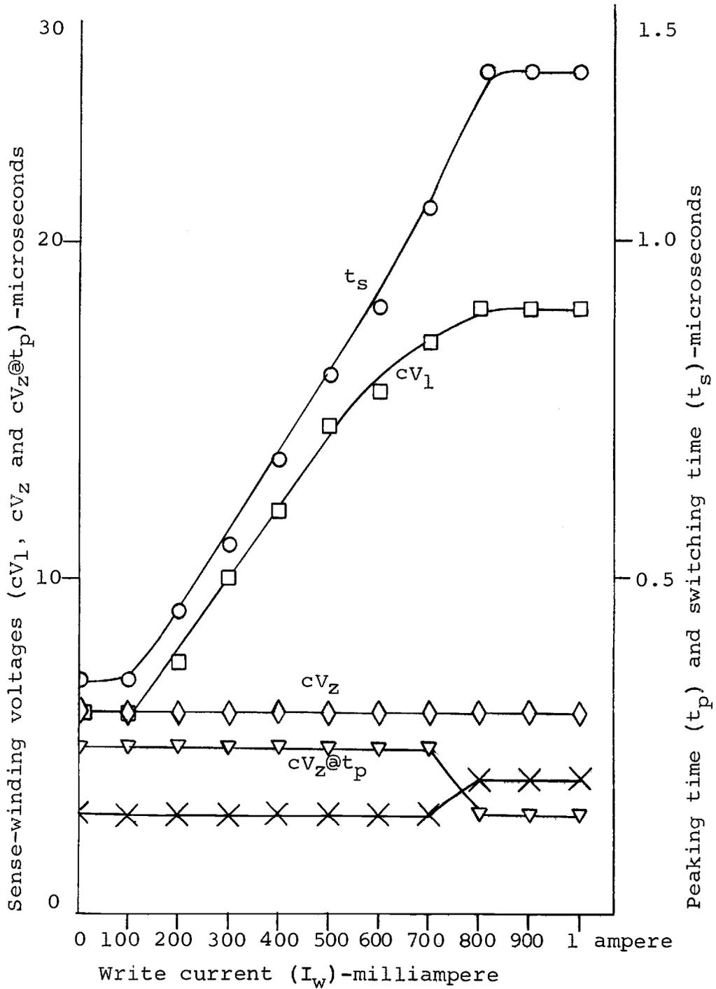
Figure 18. Variation of typical characteristics for the compensated, apertured Deltamax memory cell with write current, ( $I_w$ ). (See Table VI, Appendix VI, for test conditions)
