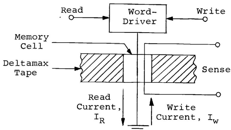
Figure 5. System diagram of the uncompensated, apertured Deltamax memory cell.
