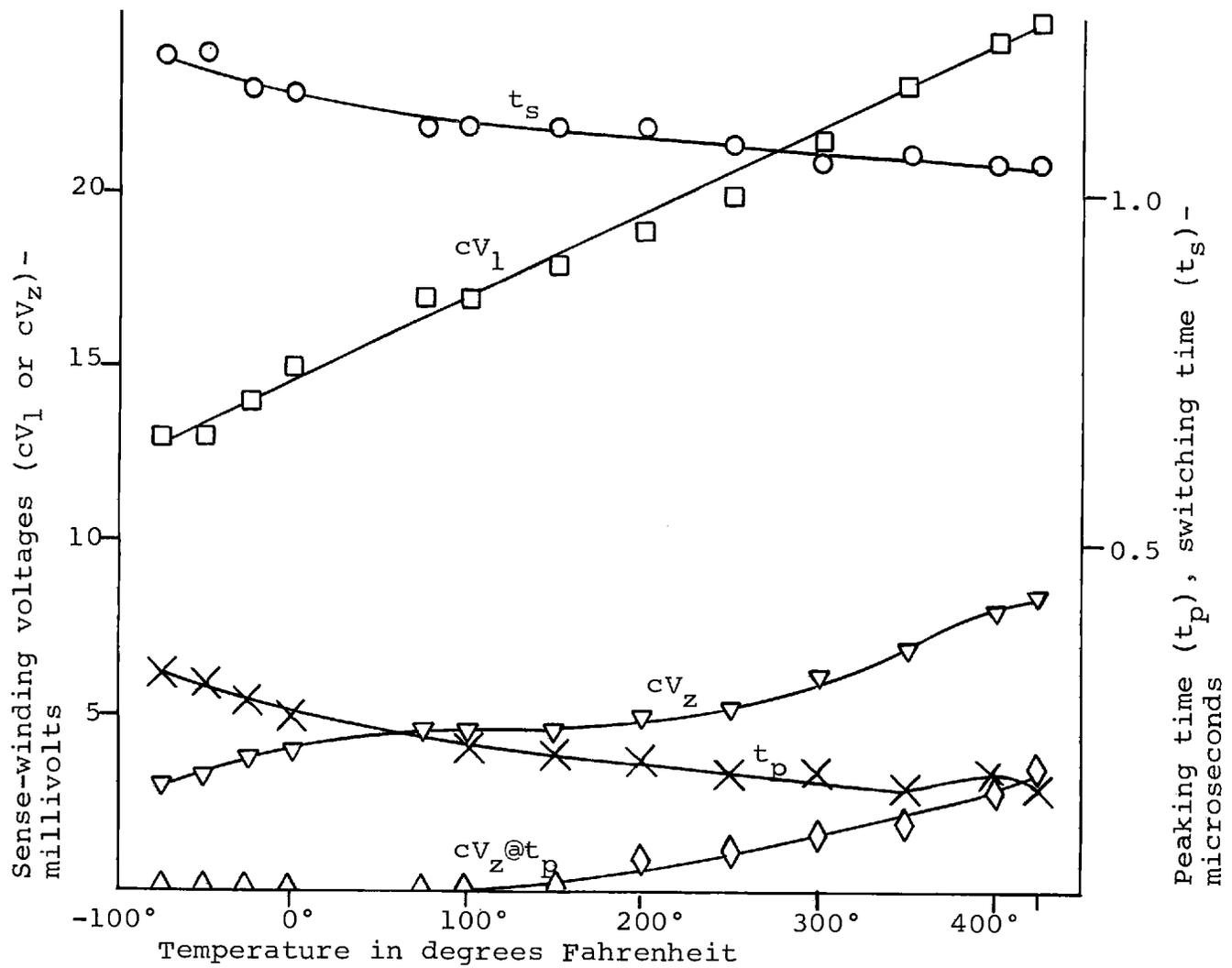
Figure 20. Temperature effect on the response of the compensated, apertured Deltamax memory cell. (See Table VIII, Appendix VI)
