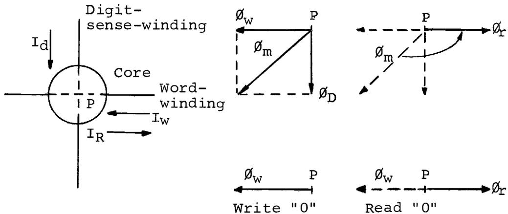
Figure 25. Flux vector diagram of type III element.
