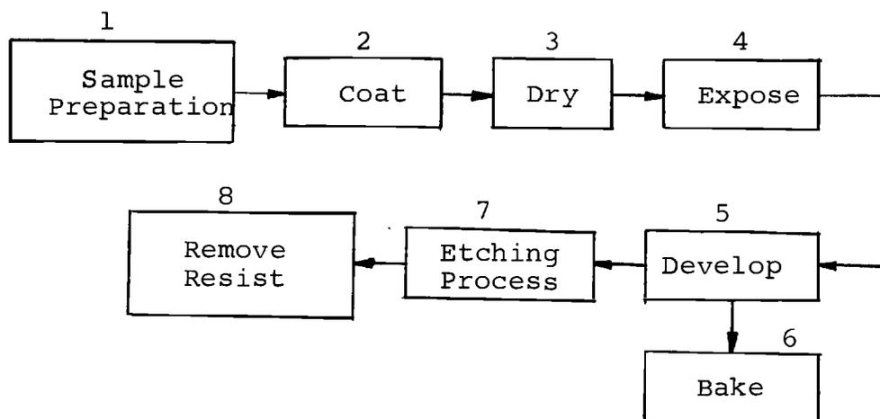
Figure 33. Flow diagram of the basic procedures of photolithographic techniques.
