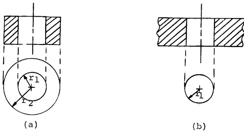
Figure 1. Geometry of (a) toroidal core, (b) memory cell.
