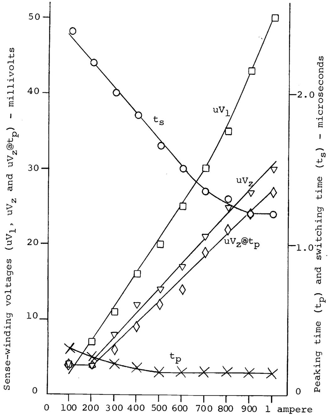
Figure 8. Typical characteristics for the uncompensated, apertured Deltamax memory cell.
