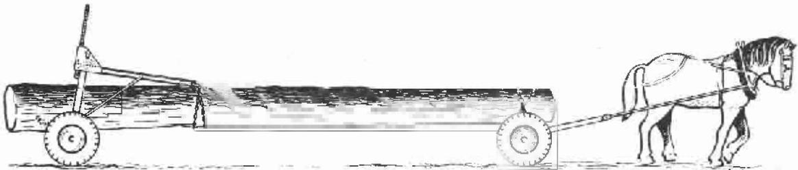
Figure 2.--Transporting logs with a sulky and bumper.
