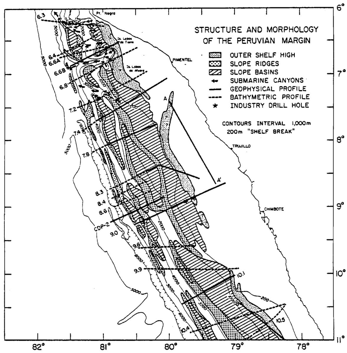
Figure 2A. Structural ridges, sedimentary basins, and submarine canyons of the Peru continental margin. Bathymetric and seismic control is plotted: profiles are referred to by latitudinal degree of intersection with the 200 m contour.
