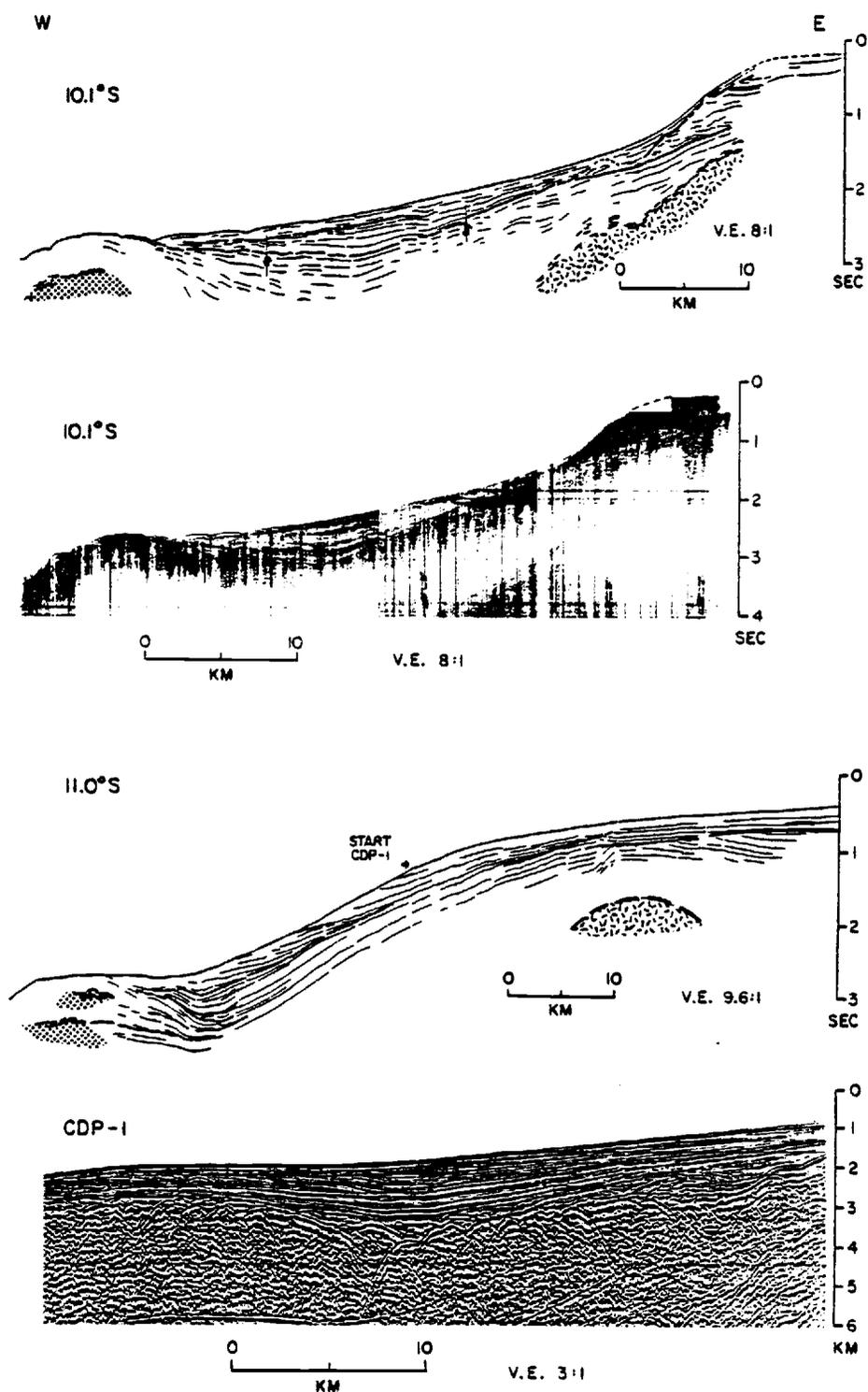
Figure 4C. Seismic reflection line interpretations and actual records across the Lima Basin. Note the good correlation between the single channel record SP-11.0 and the nearly coincident multi-channel record CDP-1 below. See page 16 for caption.
