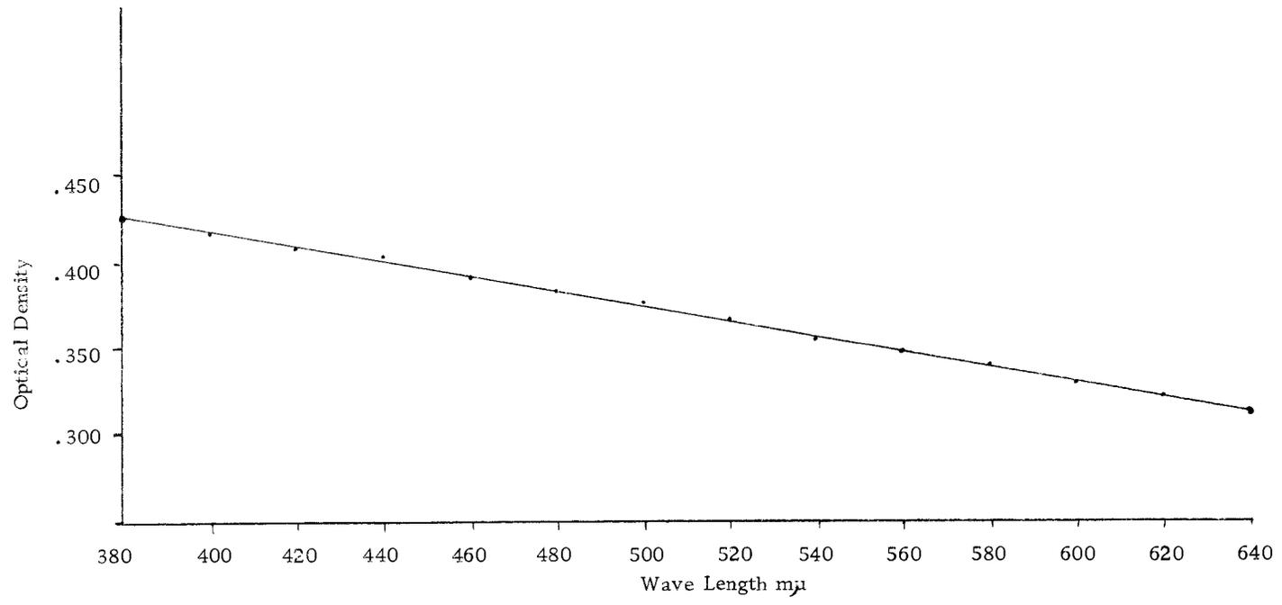
Figure 2. Optical density values of a melanin granule suspension as influenced by wave length setting - Trial 1A. (Zeiss PMQ2 Spectrophotometer)
