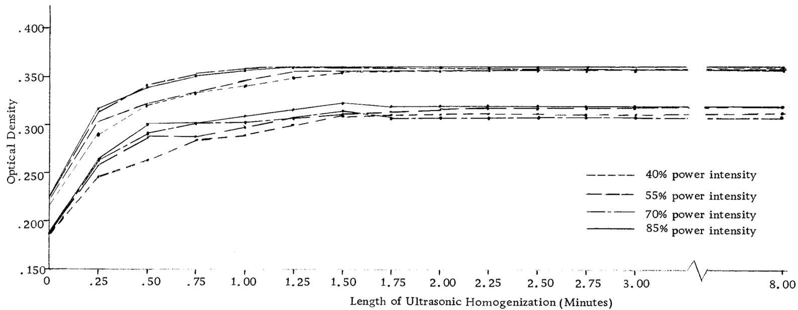
Figure 4. Effect of ultrasonic homogenization on optical density of two melanin granule suspensions of different concentrations run at power intensities ranging from 40 to 85 percent - Trial 2A.
