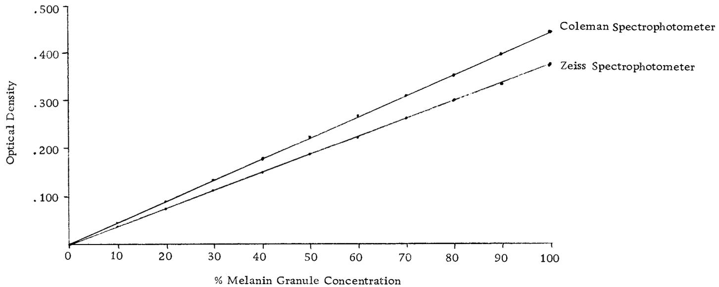
Figure 3. Optical density of a Melanin granule suspension at concentrations ranging from 0 to 100% as determined on two makes of spectrophotometers - Trial 1B.
