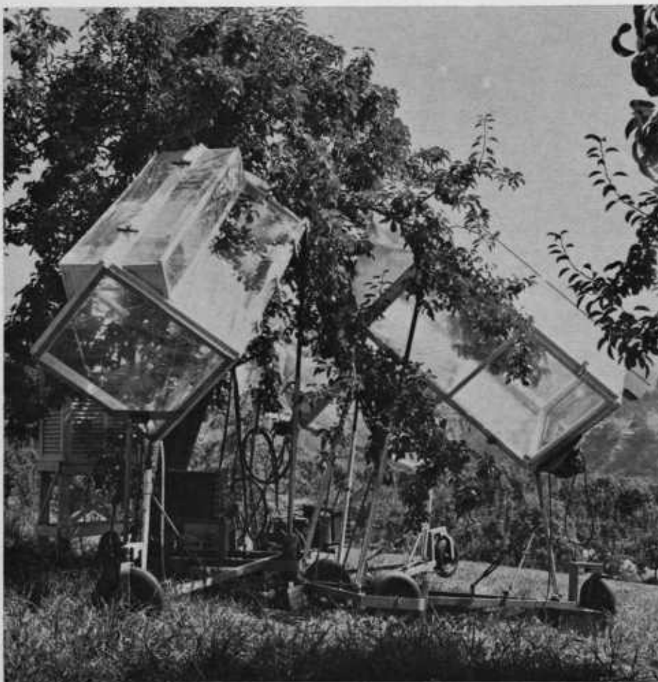
Using these temperature-controlled plastic limb cages, OSU researchers have successfully induced premature ripening condition in growing Bartlett pears.
