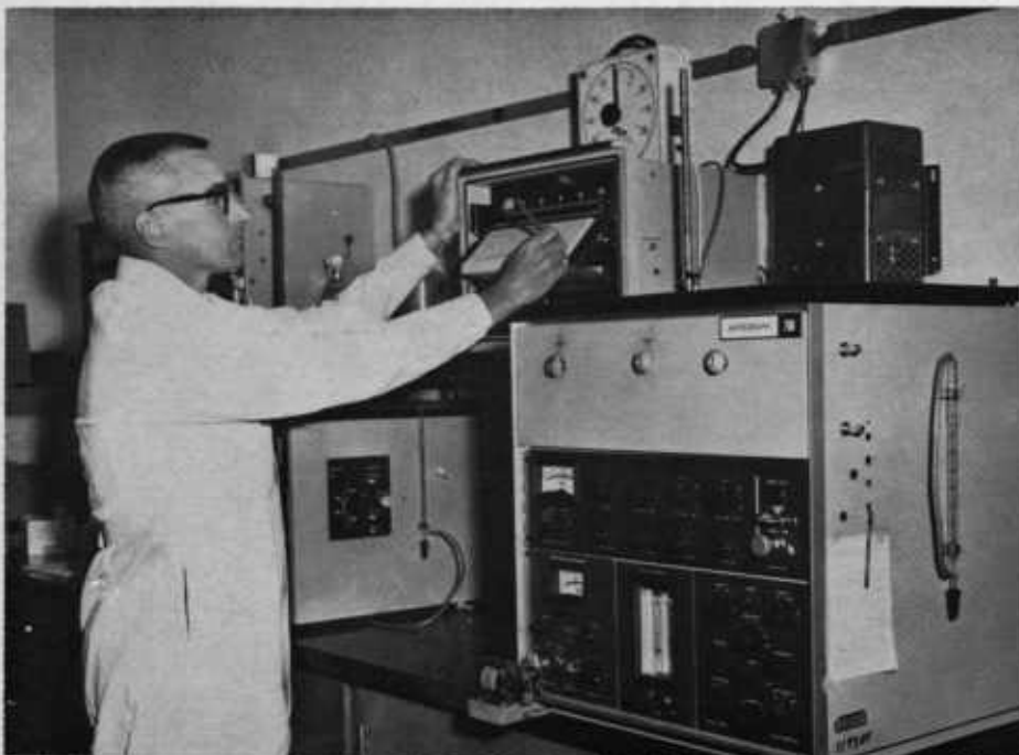
Bills examines the pattern of specially equipped gas chromatograph's reactions to test material previously treated with precise amount of ultraviolet light.
