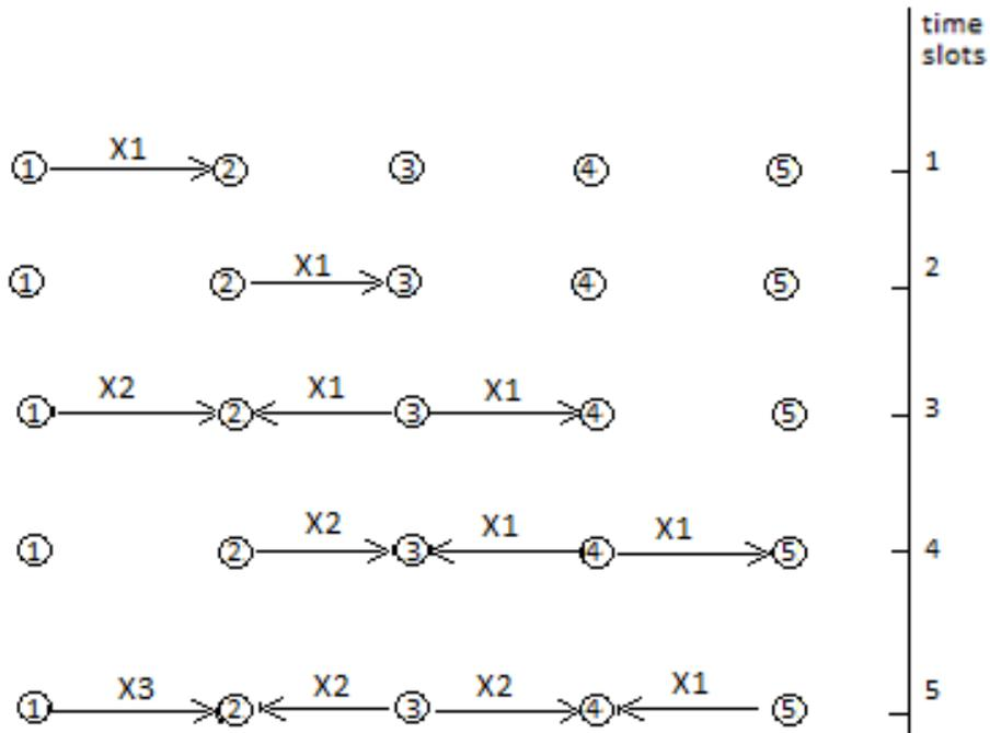
Figure 4.2: Unidirectional PNC transmission in a linear network
