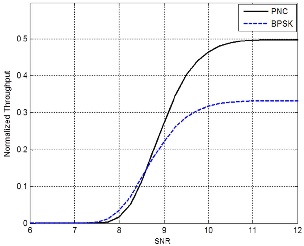
Figure 4.3: Normalized throughput of PNC and traditional transmission techniques for various SNR values
