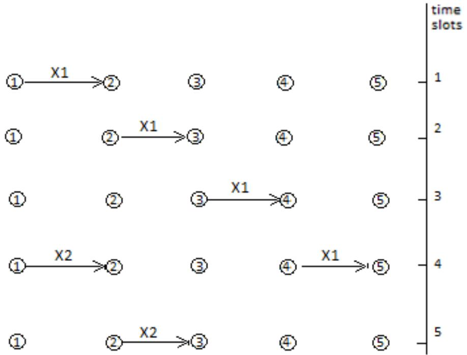
Figure 4.1: Unidirectional traditional transmission in a linear network
