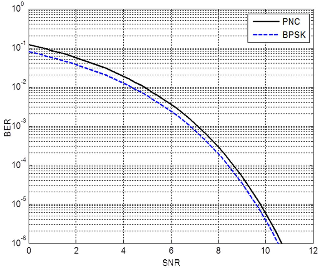
Figure 3.1: Derived BER of PNC and traditional transmission techniques
