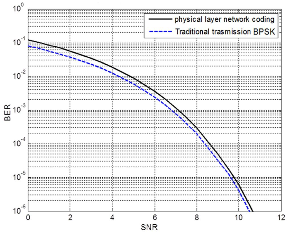
Figure 3.2: Simulated BER of PNC and traditional transmission techniques
