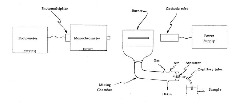
Figure 1. Schematic diagram of the atomic absorption spectrophotometer.
