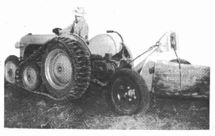
Figure 1.--Crawler track attachment for wheel tractor showing idler wheel and flexibility of tracks.
