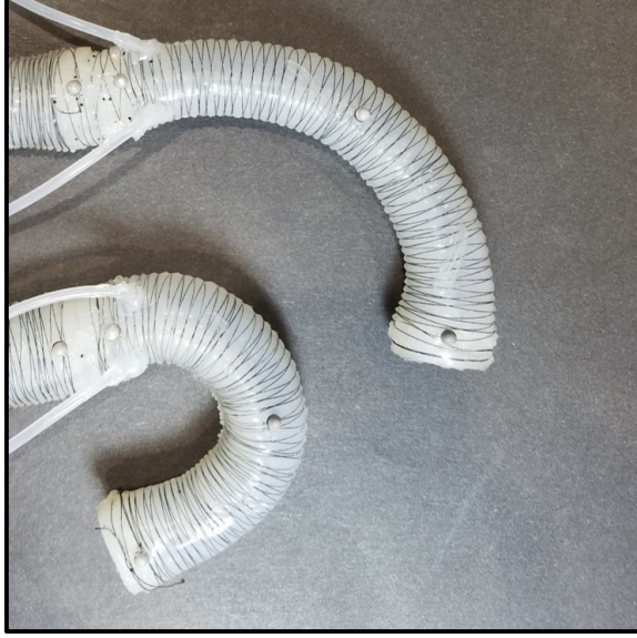
Figure 3.7: Extension in the original actuator (top), and an actuator manufactured later whose extension is restricted with an embedded rigid backbone. Both actuators are inflated with the same pressure.
