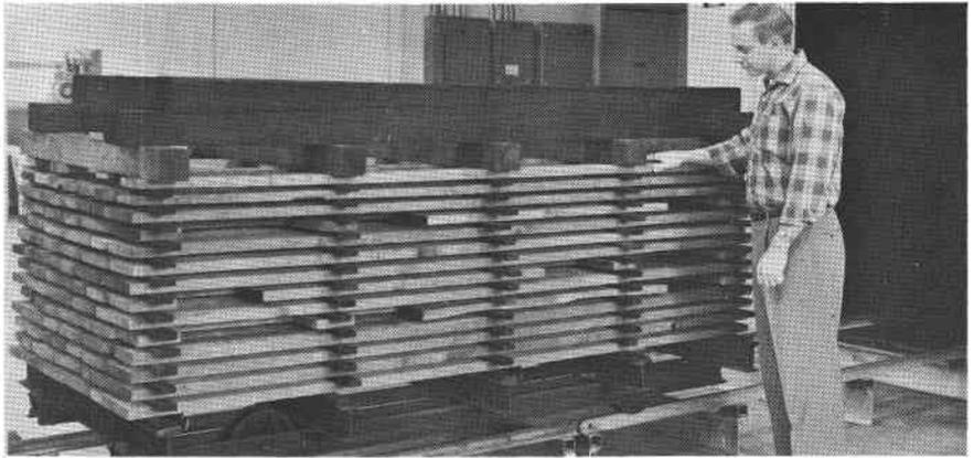
Figure 1. A charge of kiln-dried four-quarter red alder lumber with weights.
