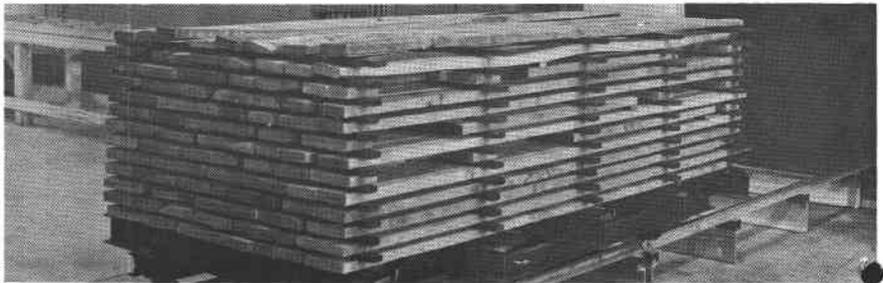
Figure 3. A charge dried at the same conditions as the charge in Figure 1, but without weights.
