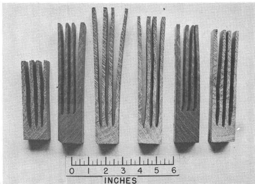
Figure 5. Casehardening stress samples from properly conditioned six-quarter red alder lumber.
