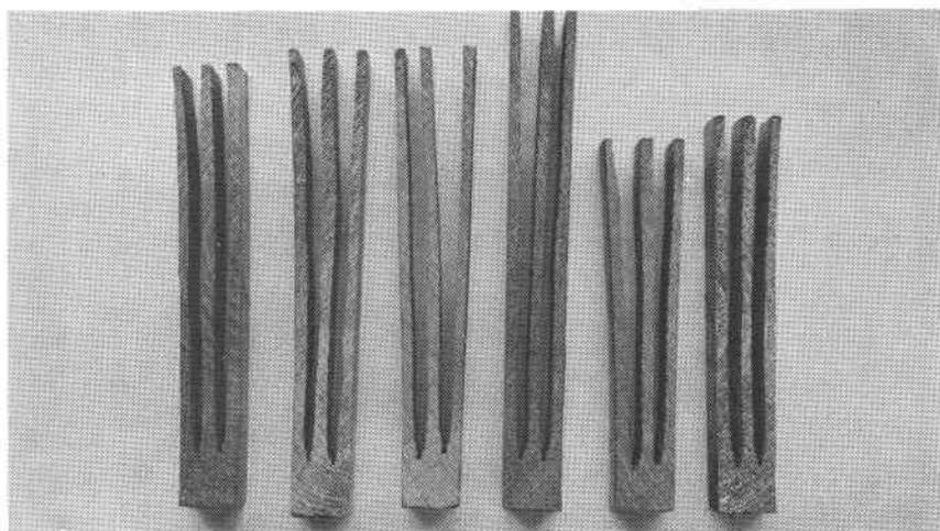
Figure 4. Casehardening stress samples from properly conditioned four-quarter red alder lumber.
