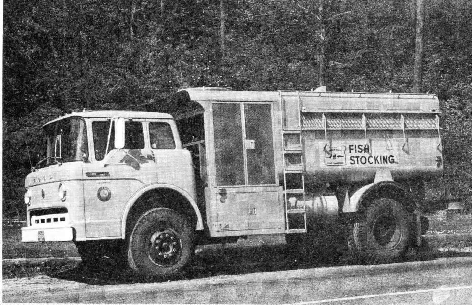
One of the newest of the Game Commission's fish liberation trucks. The 1,300-gallon refrigerated truck can haul up to 10,000 legal-sized fish for several hundred miles.
