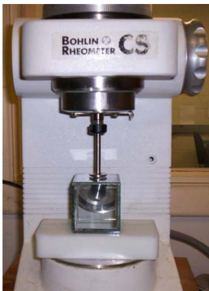
Figure 12. Device used for determination of photopolymerization time. The bottom plate was replaced by a glass plate with a mirror attached at a 45° angle underneath.
