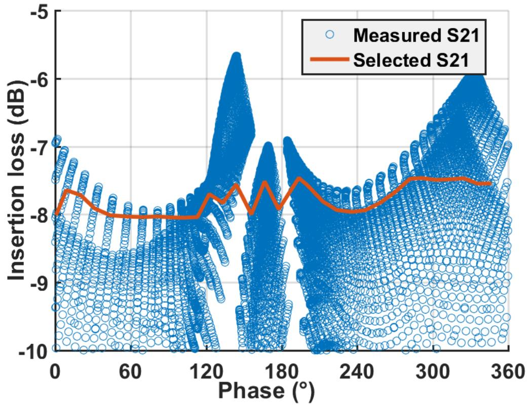
Figure 5.2: Measured stand-alone RTPS insertion loss and phase shift across load settings at 28 GHz.
