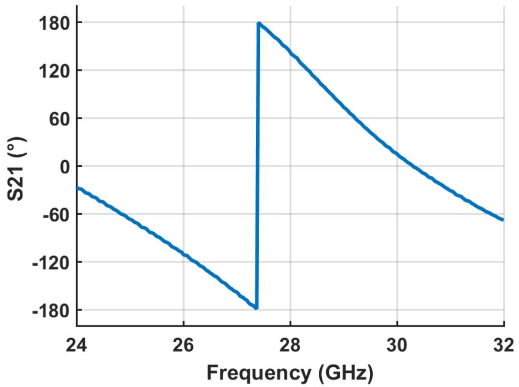
Figure 5.8: Measured  $S_{21}$  phase across frequency for  $[C_{1,max}, C_{2,max}]$
