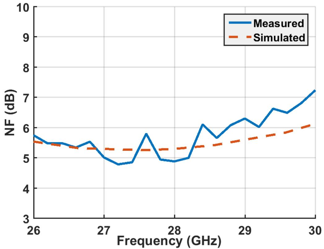
Figure 5.9: Comparison of measured and simulated noise figure for the frontend for  $[C_{1,max}, C_{2,max}]$
