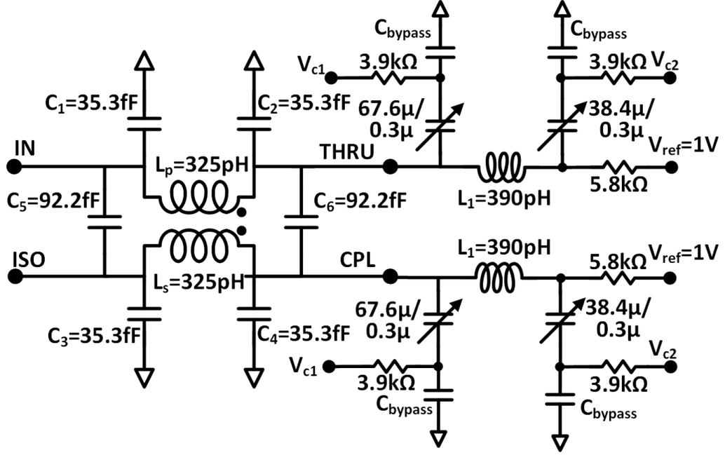
Figure 4.1: Implementation of RTPS in 65 nm TSMC
