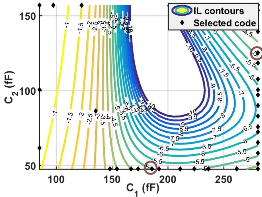
Figure 3.5: Insertion loss contours for different values of  $C_1$  and  $C_2$  and the selected code for minimum loss across phase shift range
