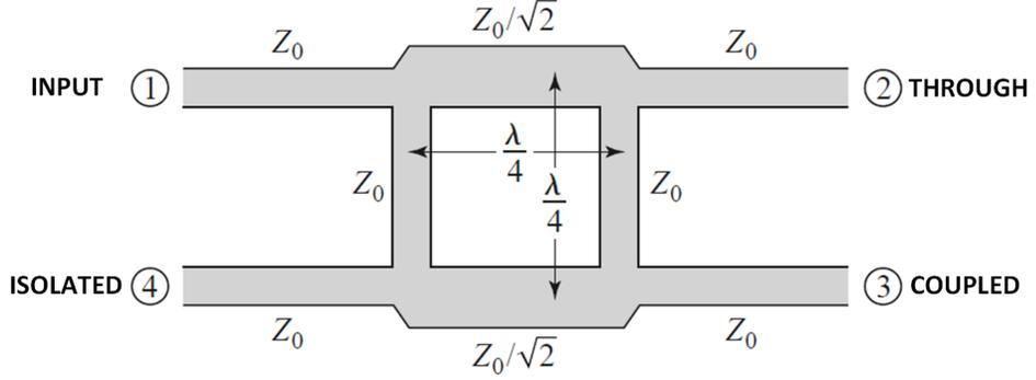
Figure 2.3: Schematic of branch-line hybrid coupler
