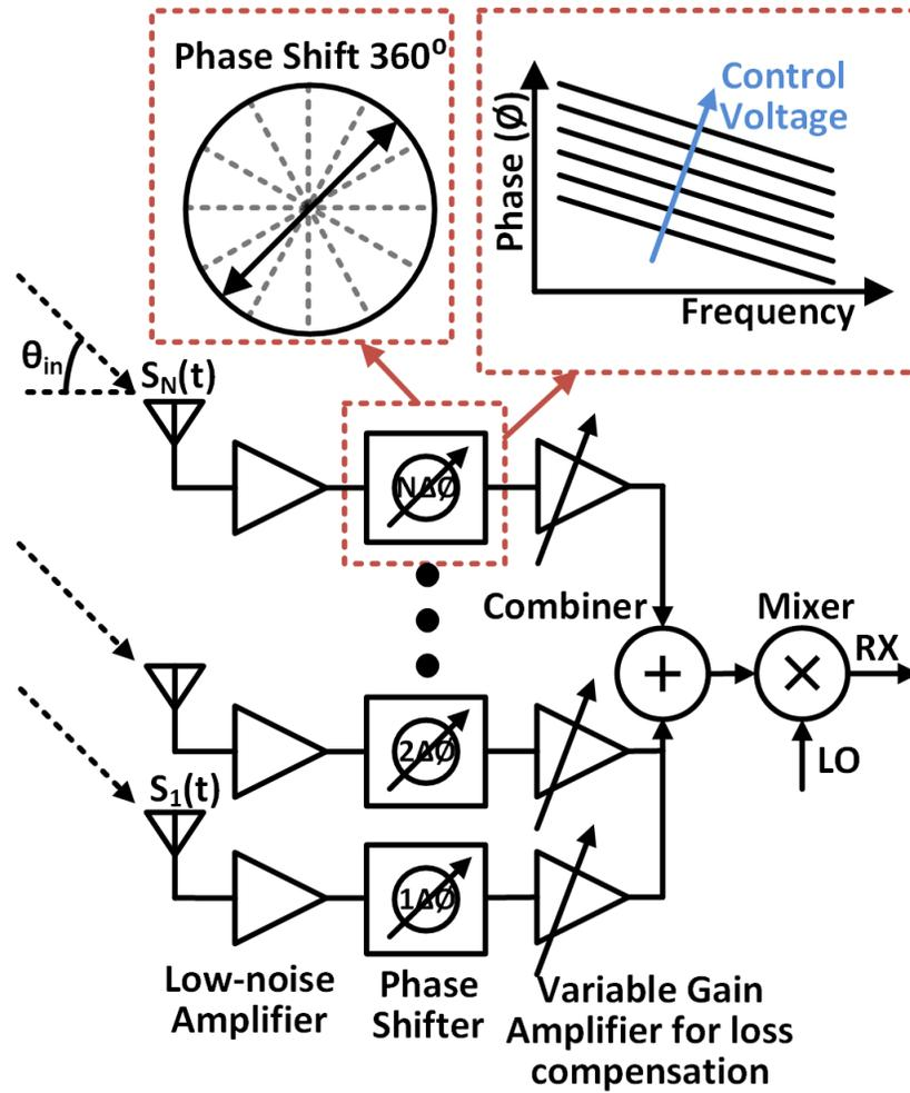
Figure 1.1: Phased-array receiver architecture and desired phase shifter characteristics
