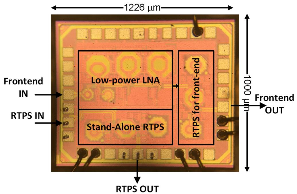
Figure 5.1: Micro-photograph of wire-bonded die - Stand-alone RTPS case
