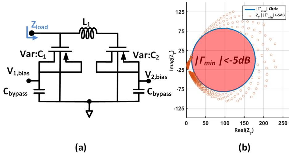
Figure 3.2: (a) Variable  $\Pi$  load based on varactors (b) Impedance circles corresponding to  $|\Gamma_T|=-5$  dB
