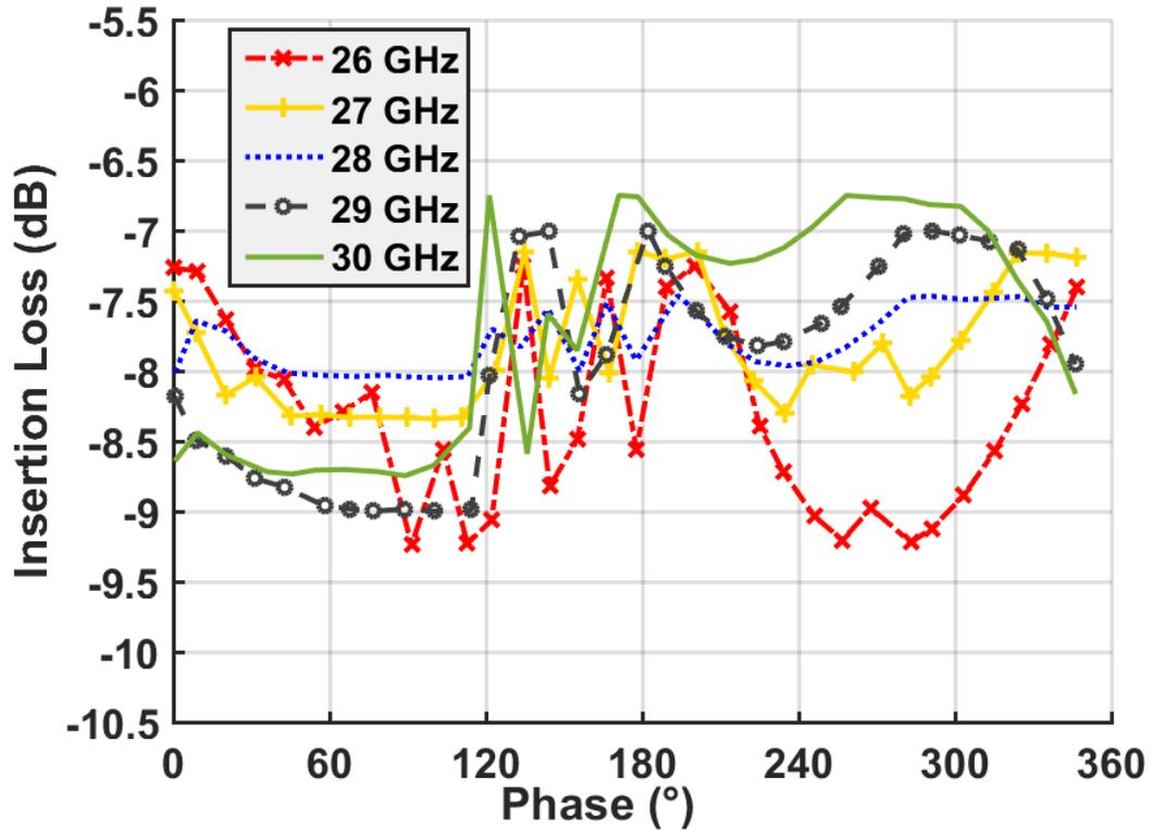
Figure 5.5: Measured RTPS insertion loss with phase shift across frequency
