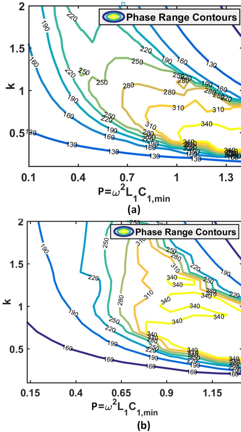
Figure 3.6: Phase range contours for different values of  $K$  and  $P$  and (a)  $C_{1,\min} = 45$  fF (b)  $C_{1,\min} = 85$  fF
