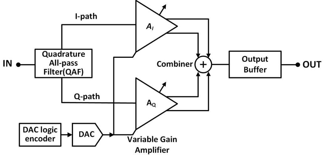
Figure 2.1: Architecture of vector modulator based active phase shifter
