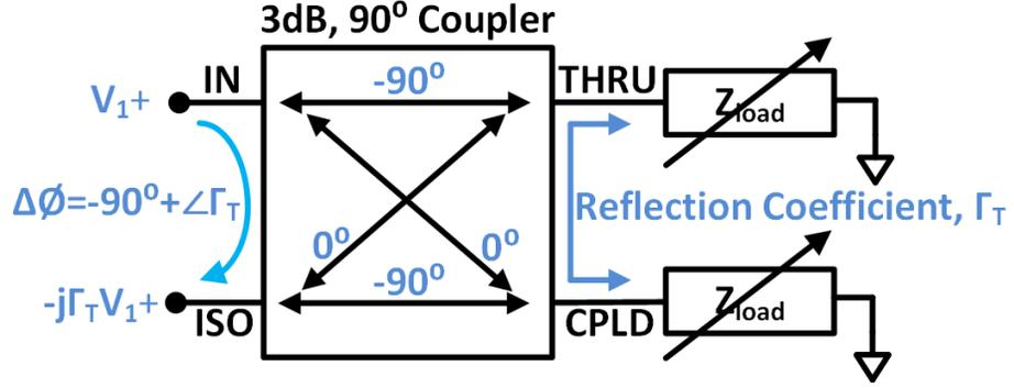
Figure 2.4: Architecture of reflection-type phase shifter
