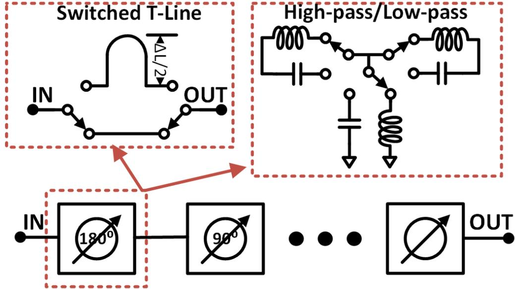
Figure 2.2: Architecture of switched t-line based N-bit phase shifter
