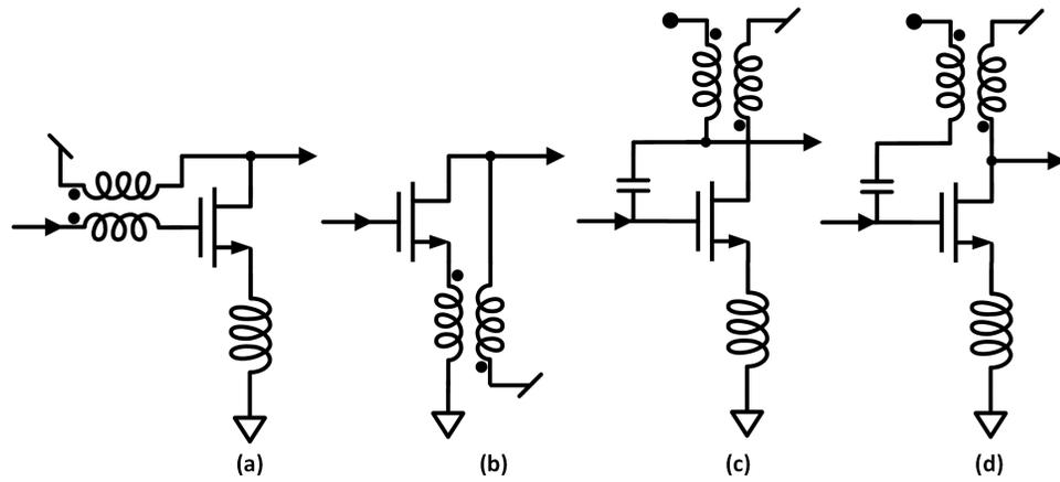
Figure 3.7: (a,b) Gain boosting through transformer feedback from drain to gate/-source (c,d) Neutralization with  $C_{GD}$  cancellation through transformer feedback
