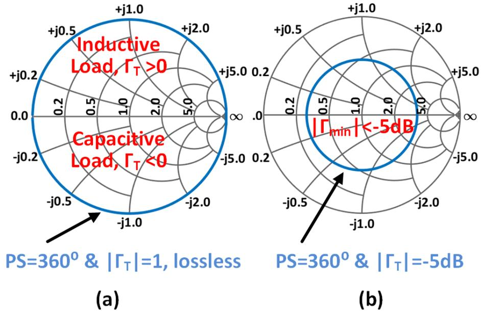
Figure 3.1: Representation of desired & practical  $\Gamma$  on Smith chart (a) Ideal  $|\Gamma_T|=0$  dB circle (b)  $|\Gamma_T|=-5$  dB circle
