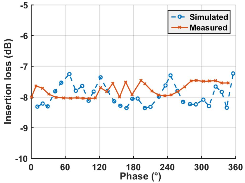
Figure 5.3: Measured vs. simulated performance for stand-alone RTPS at 28 GHz
