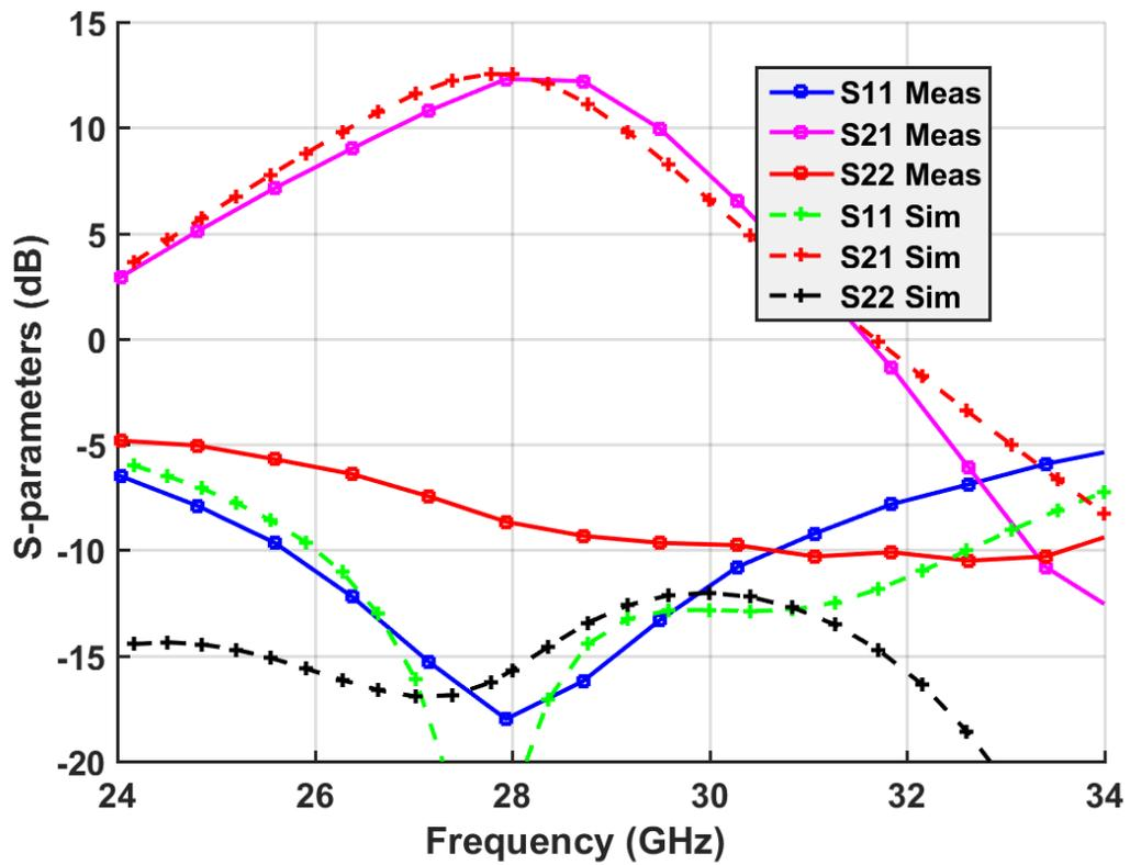
Figure 5.6: Comparison of measured and simulated S-parameters for the frontend for  $[C_{1,max}, C_{2,max}]$
