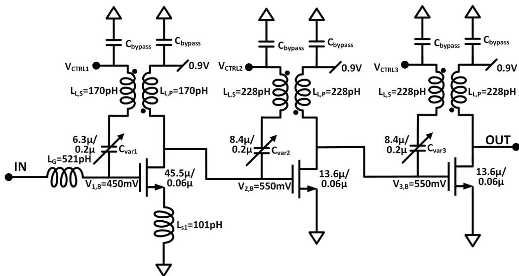
Figure 4.2: 3-stage neutralization LNA
