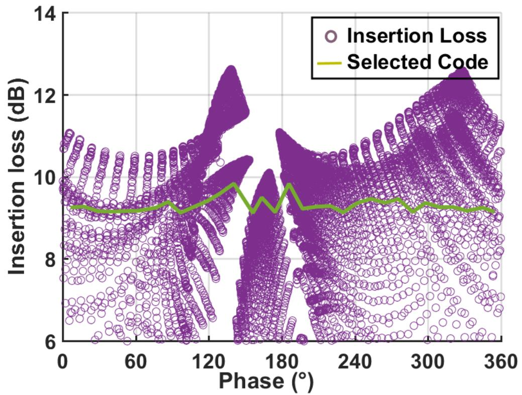
Figure 5.7: Frontend measured loss across  $[C_1, C_2]$  corners and the selected output
