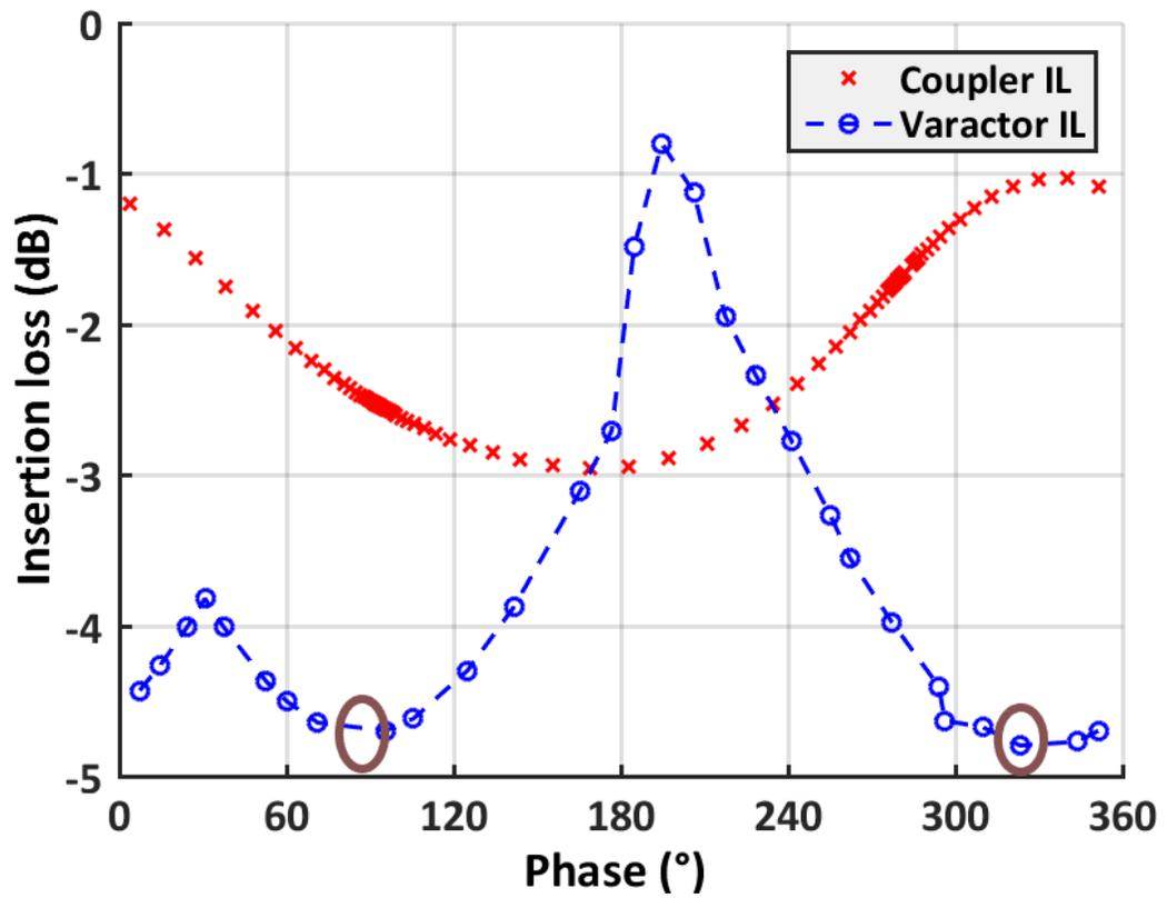
Figure 3.4: Coupler and  $\Pi$  load insertion losses with phase shift for selected varactor code
