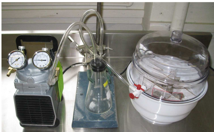
Figure 4.15: Vacuum desiccator to dry and store samples for XRD analysis
