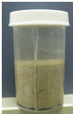
Figure 4.18: Cracked vial due to expansion of GCX inside, at 38 °C.
