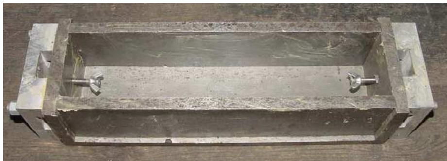
Figure 2.14: Modified ASTM C157 Prism Mold (Ramniceanu et al. 2010)
