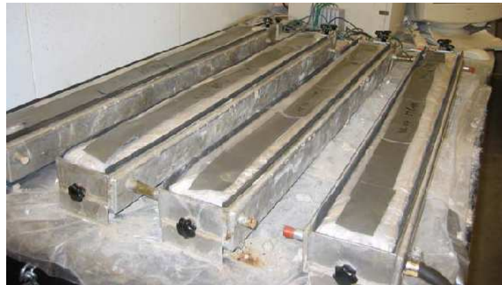
Figure 2.17: Linear measurement of autogenous shrinkage (Schleibinger Shrinkage Drain)
