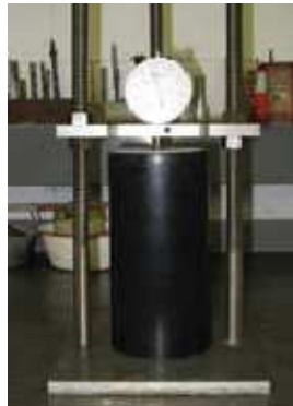
Figure 2.18: Cylindrical mold method ( Bentz et al. 2009 )
