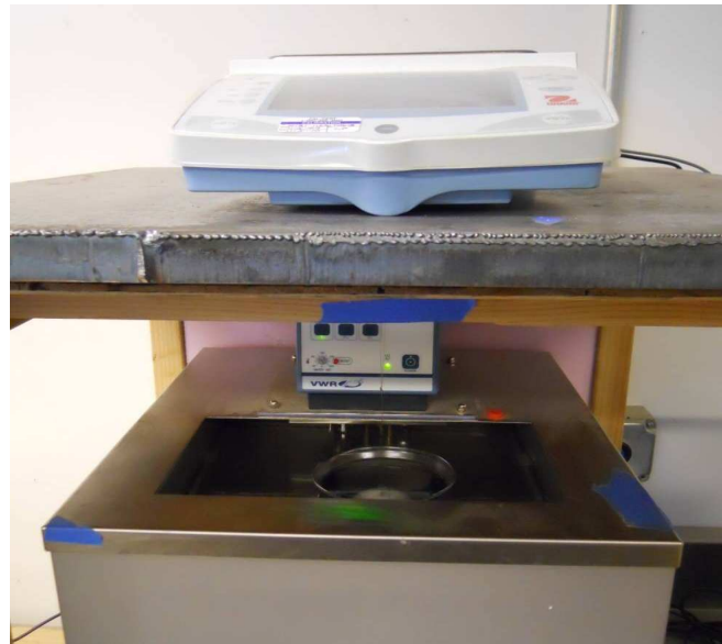
Figure 2.8: Experimental set-up for membrane method to test autogenous strain for cement paste
