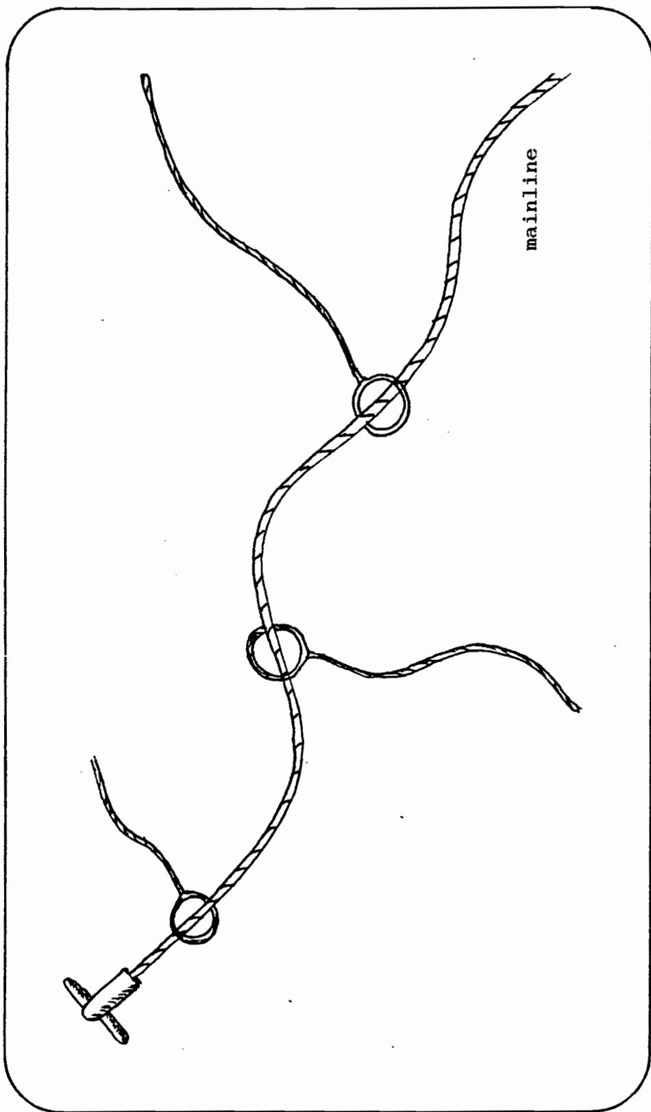
Figure 5. Ring and toggle choker system.
