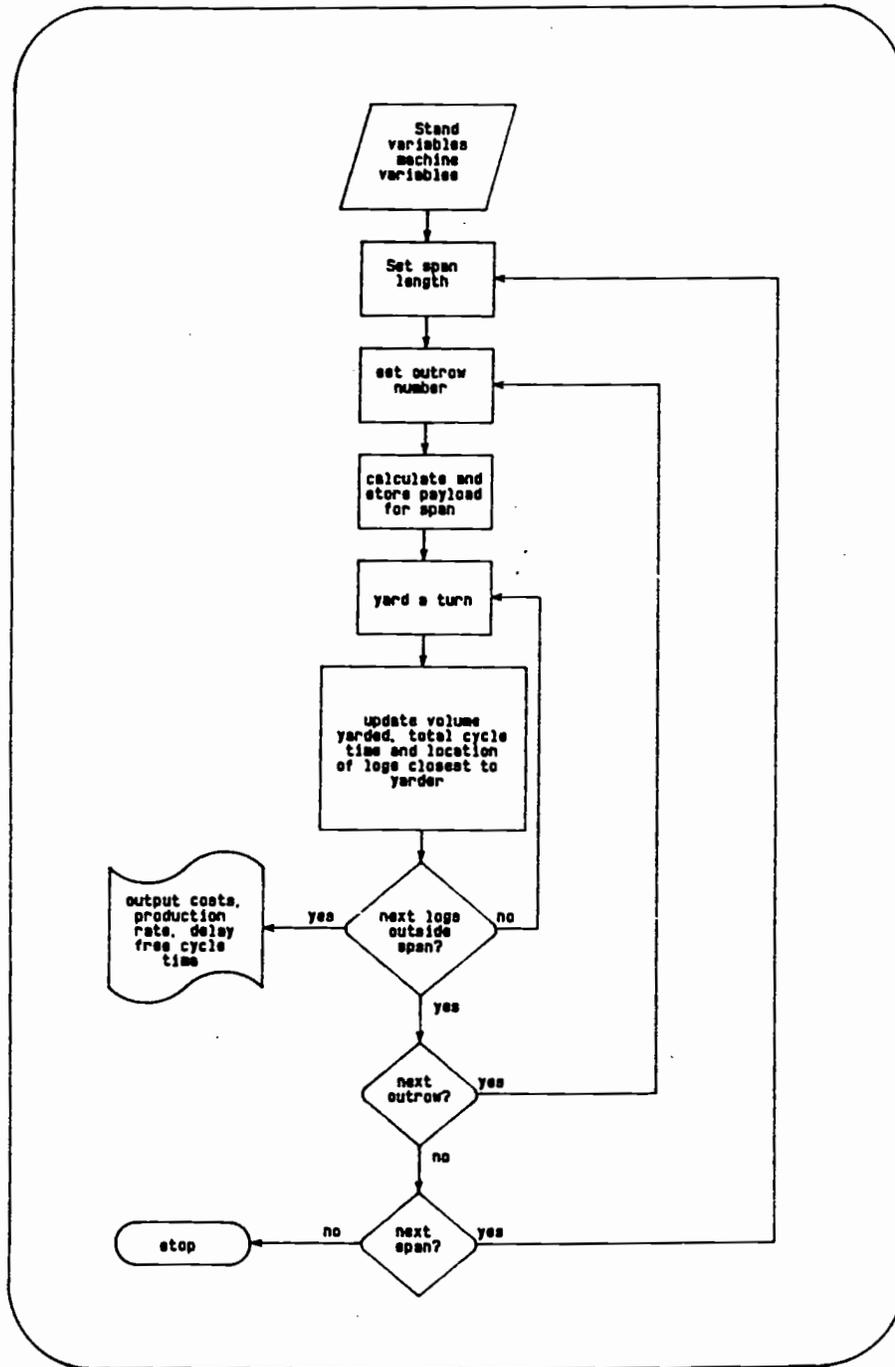
Figure 3. Flow chart of the simulation sequence.
