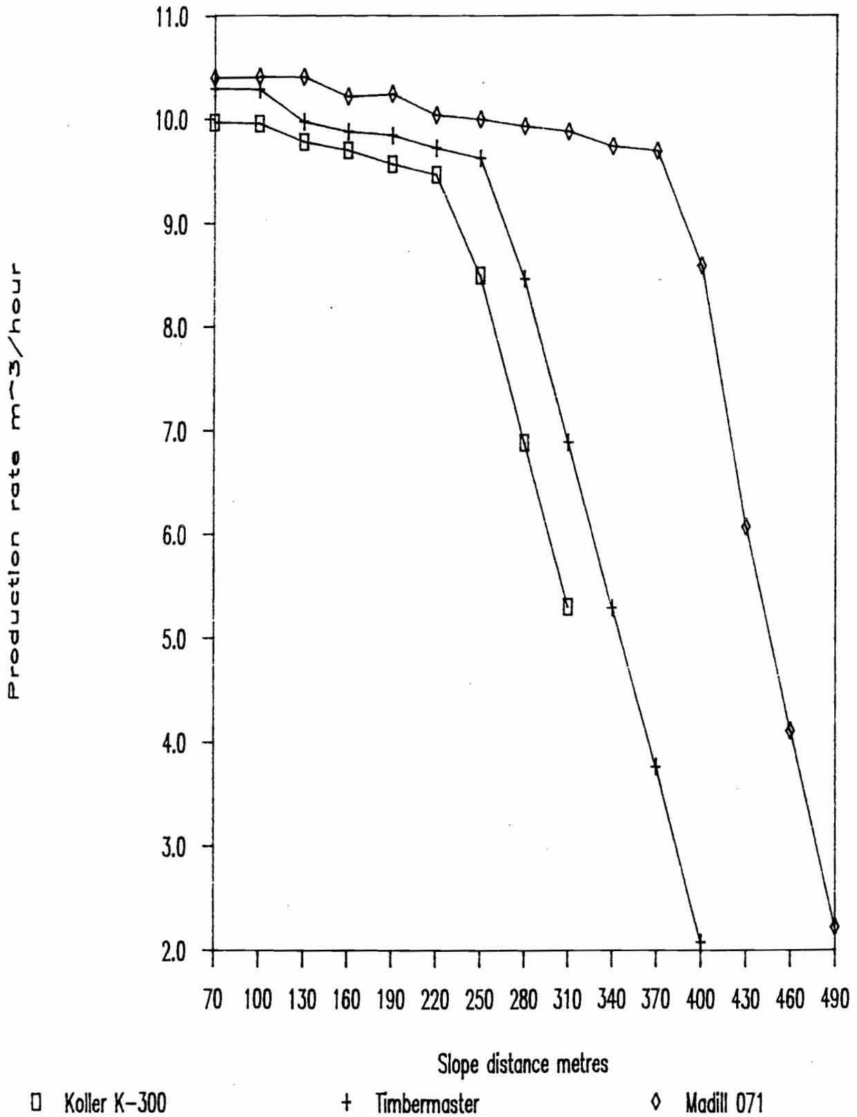
Figure 10. Production Rate, 0.20 cubic metre tree size.
