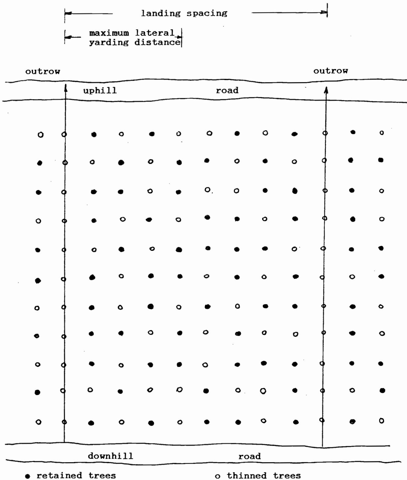
Figure 8. Relationship between outrow spacing, maximum lateral outhaul distance and the stems removed per hectare.
