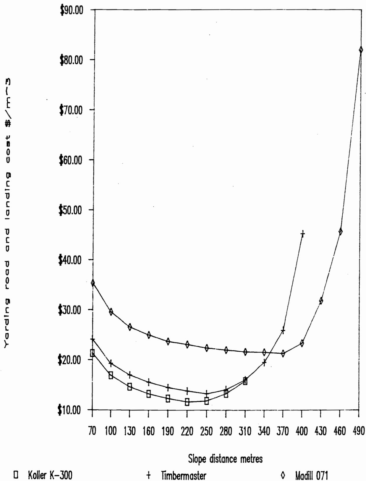
Figure 14. Yarding, Road, and Landing Cost, 0.20 cubic metre tree size.
