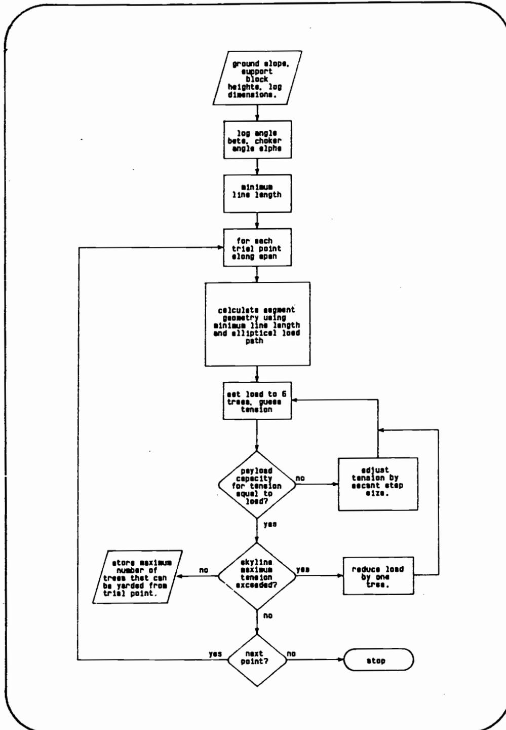
Figure 6. Flow chart for payload calculation.
