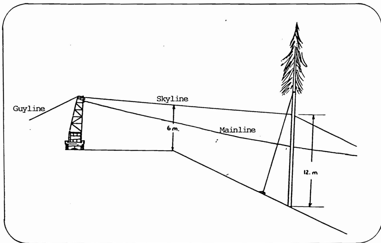
Figure 2. Intermediate support block location.
