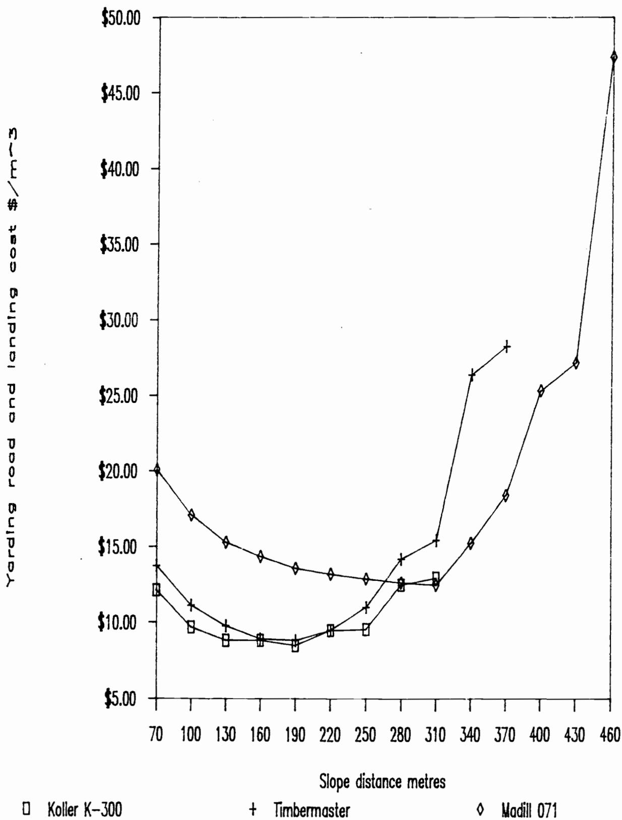
Figure 17. Yarding, Road, and Landing Cost, 0.35 cubic metre tree size.
