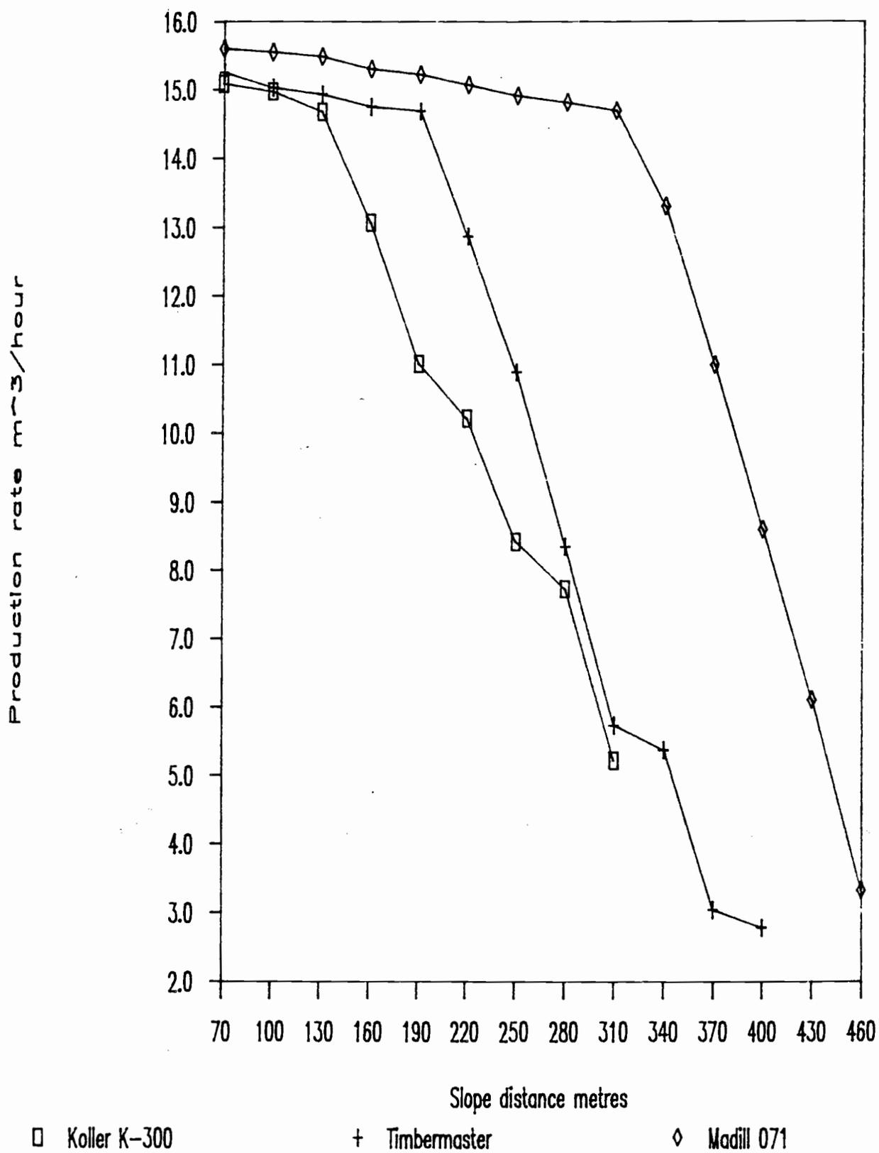
Figure 12. Production Rate, 0.30 cubic metre tree size.
