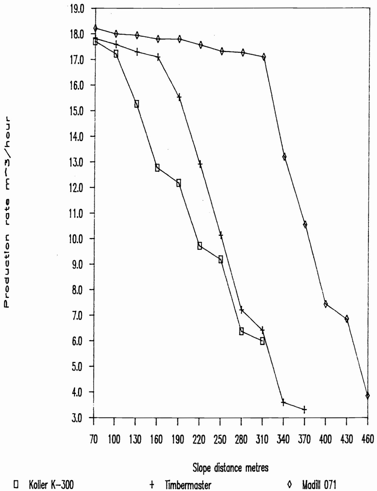
Figure 13. Production Rate, 0.35 cubic metre tree size.
