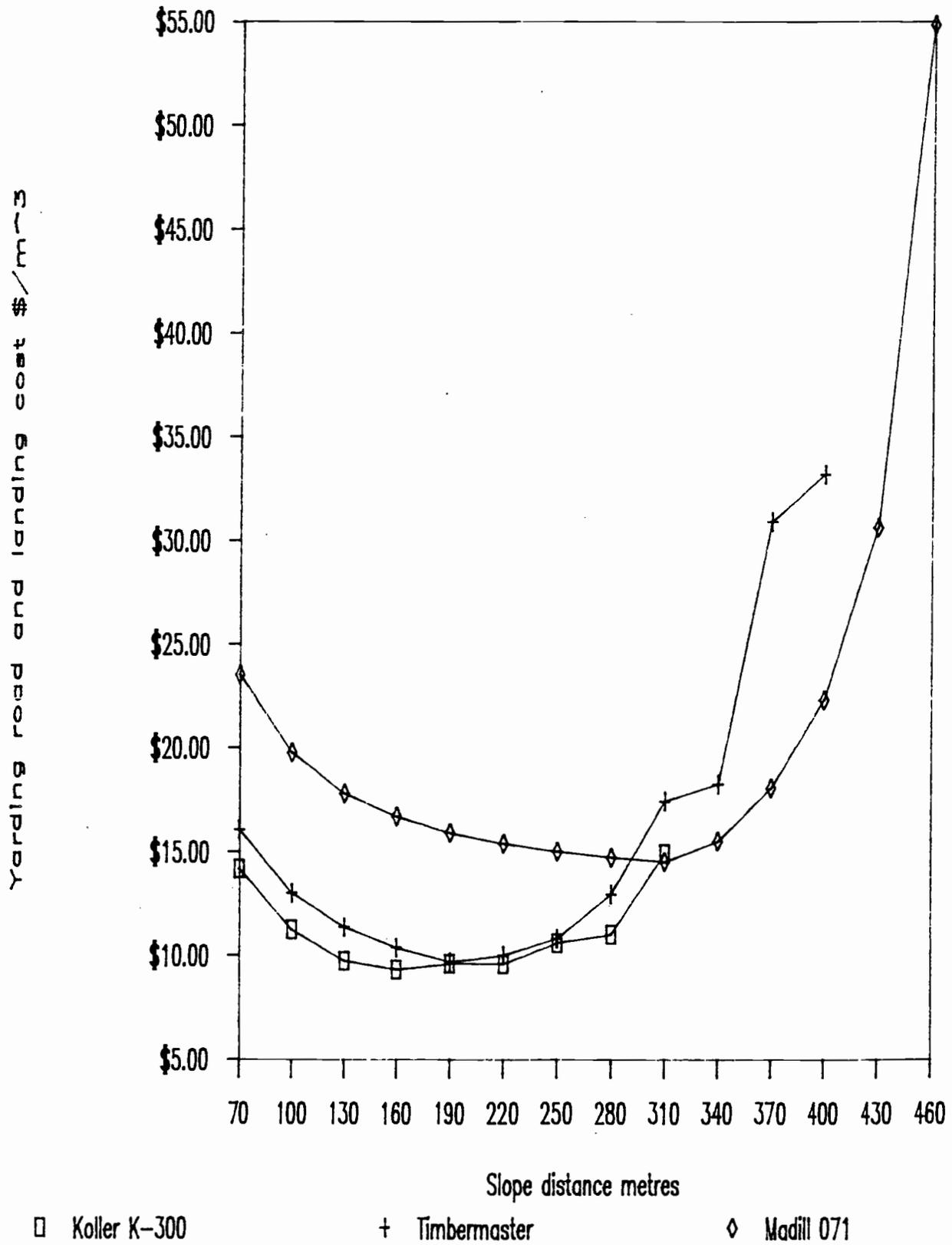
Figure 16. Yarding, Road, and Landing Cost, 0.30 cubic metre tree size.
