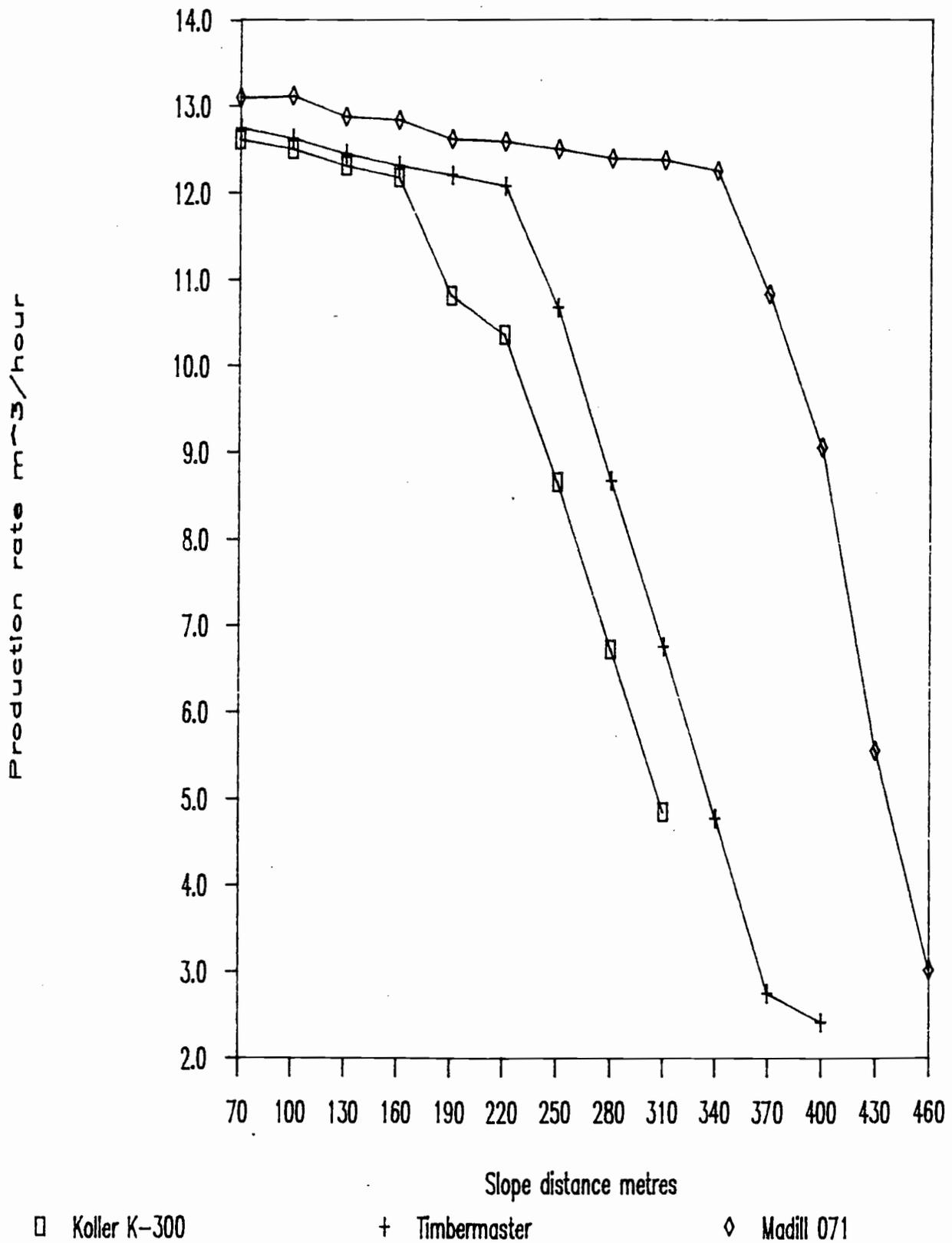
Figure 11. Production Rate, 0.25 cubic metre tree size
