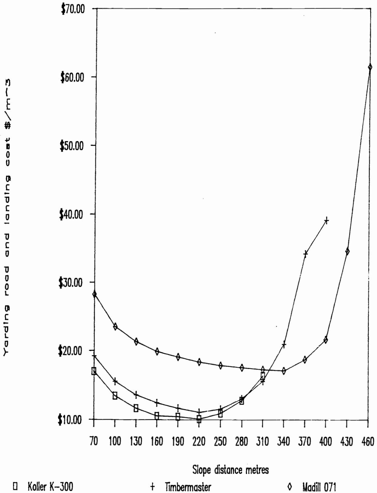
Figure 15. Yarding, Road, and Landing Cost, 0.25 cubic metre tree size.
