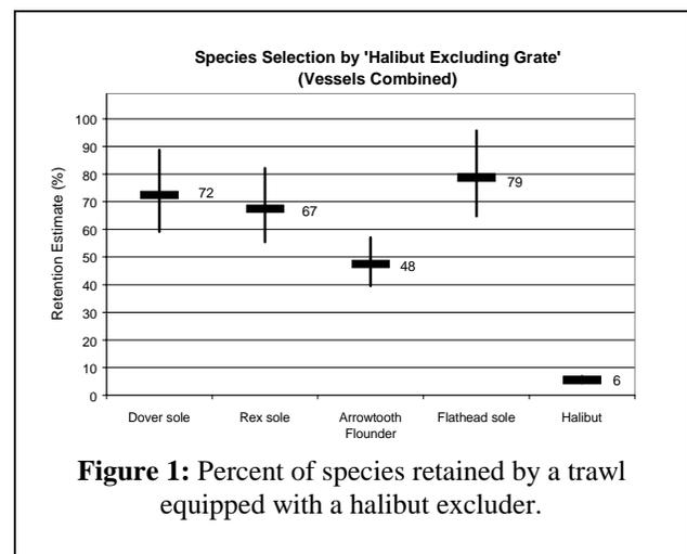
Figure 1: Percent of species retained by a trawl equipped with a halibut excluder.
