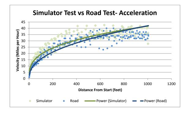
Figure 19. Comparison of Simulator and Road Test Acceleration Curves
