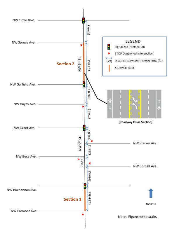
Figure 3. NW 9<sup>th</sup> Street Corridor and Test Sections
