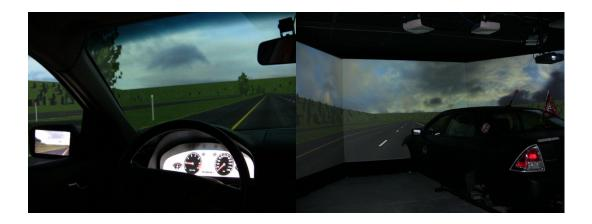
Figure 10. OSU Driving Simulator Vehicle and Projection System
