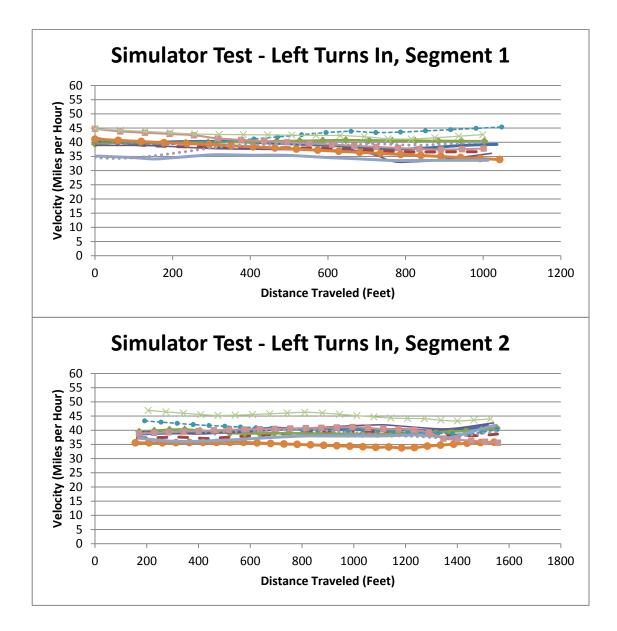
Figure 15. Simulator Test Speed Profile, Left Turns In Section, Segment 1 and 2
