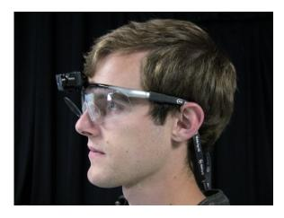
Figure 8. Mobile Eye XG Eye Tracking Equipment
