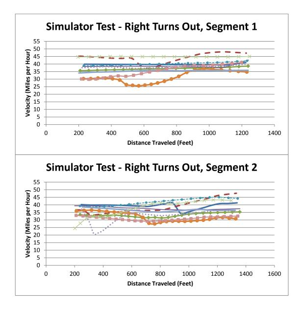
Figure 14. Simulator Test Speed Profile, Right Turns Out Section, Segment 1 and 2
