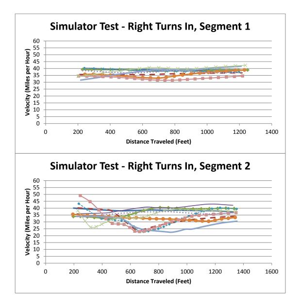
Figure 16. Simulator Test Speed Profile, Right Turns In Section, Segment 1 and 2
