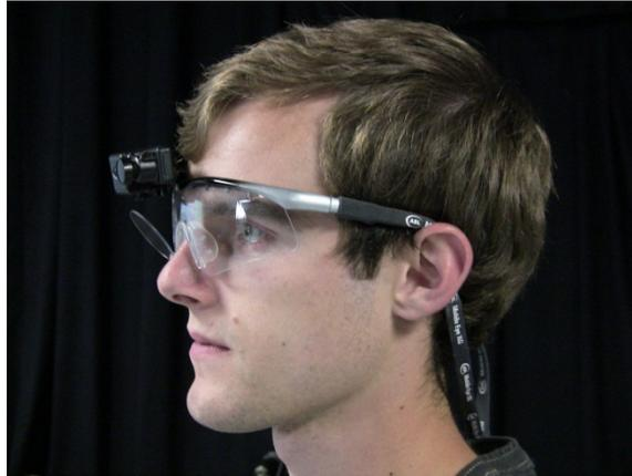
Figure 8. Mobile Eye XG Eye Tracking Equipment
