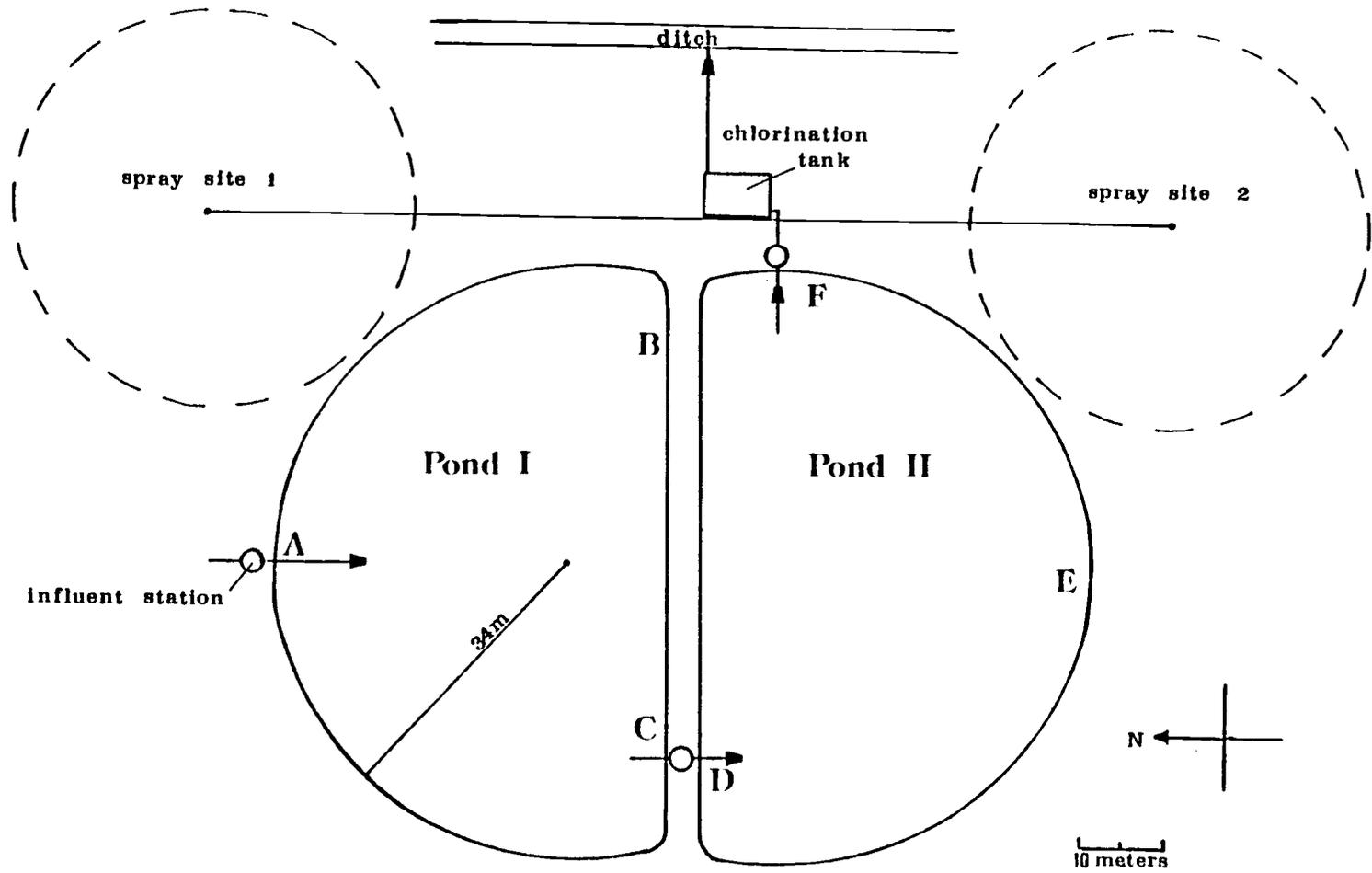
Figure 1. The Corvallis Airport Sewage Lagoon. The locations of stations A through F and the positions of the influent (at A) and the effluent (at F) are shown.
