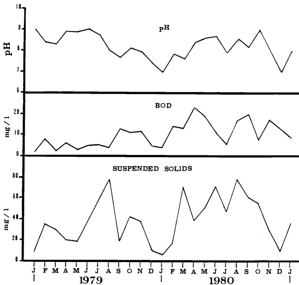
Figure 4. Effluent from Pond II. Monthly values of the pH, BOD, and suspended solids during 1979 and 1980.
