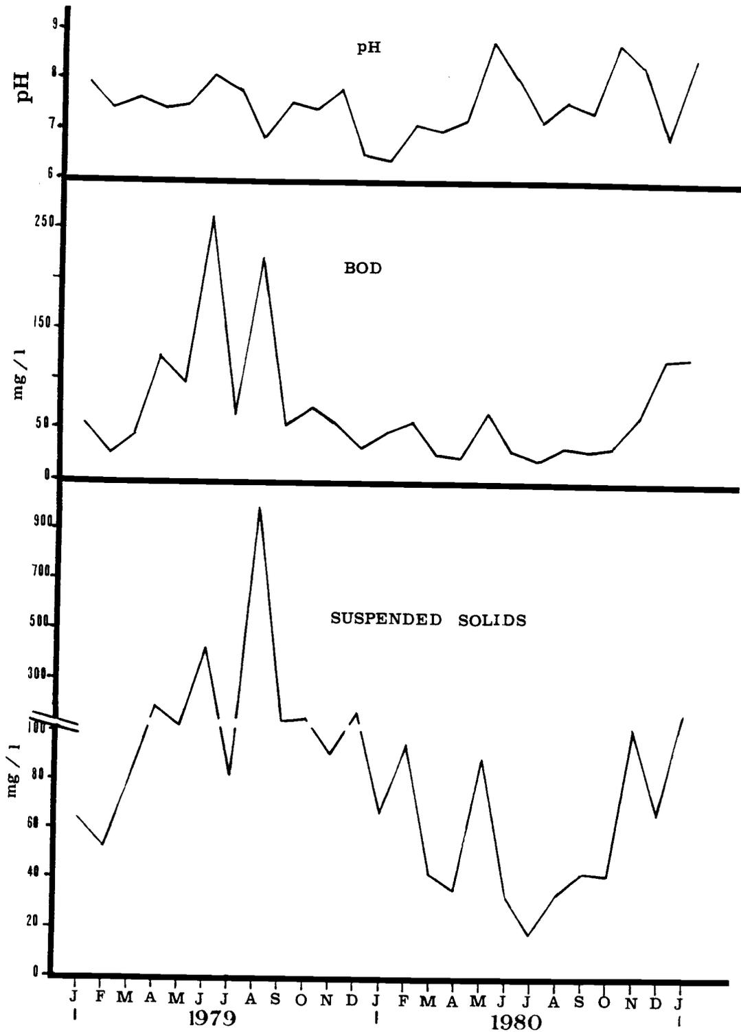
Figure 3. Influent to Pond I. Monthly values of the pH, BOD, and suspended solids during 1979 and 1980.
