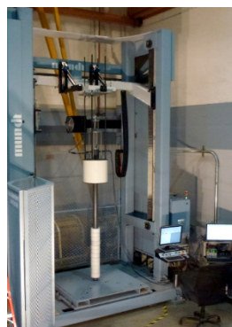
Figure 2. Testing in the Linear Test Bed (LTB). The Linear Test Bed has a maximum stroke of 2 m, force capacity of 20 kN, and a maximum speed of 1 m/s.
