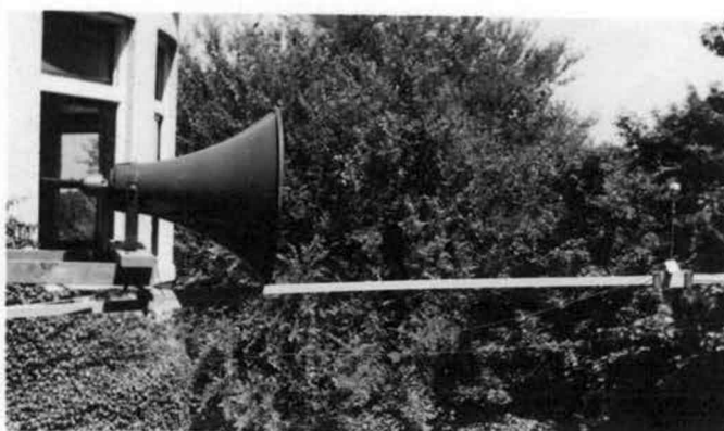
Fig. 16 - Two pictures of the loudspeaker testing location showing Driver "U" and Horn "U" extended on the apparatus boom and ready for test.
