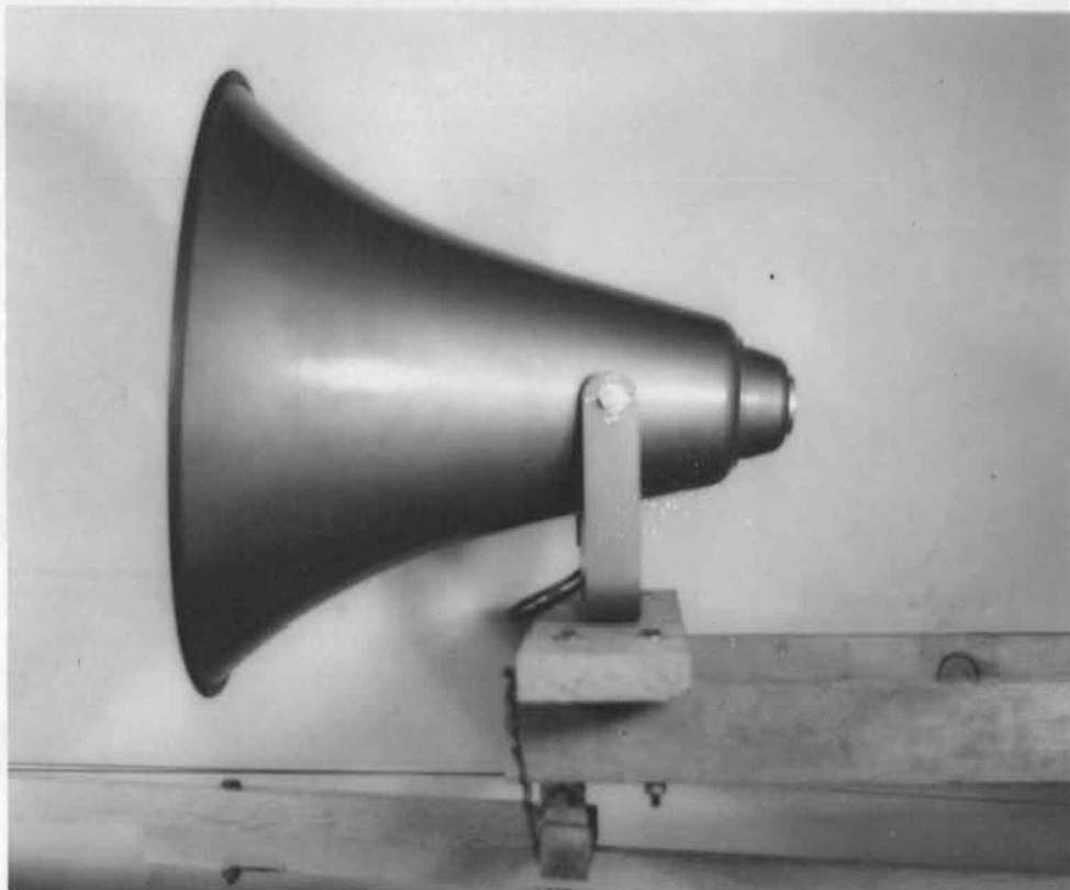
Fig. 10 - Loudspeaker unit Driver "J" and Horn "J" mounted in the test rack and ready for operation.
