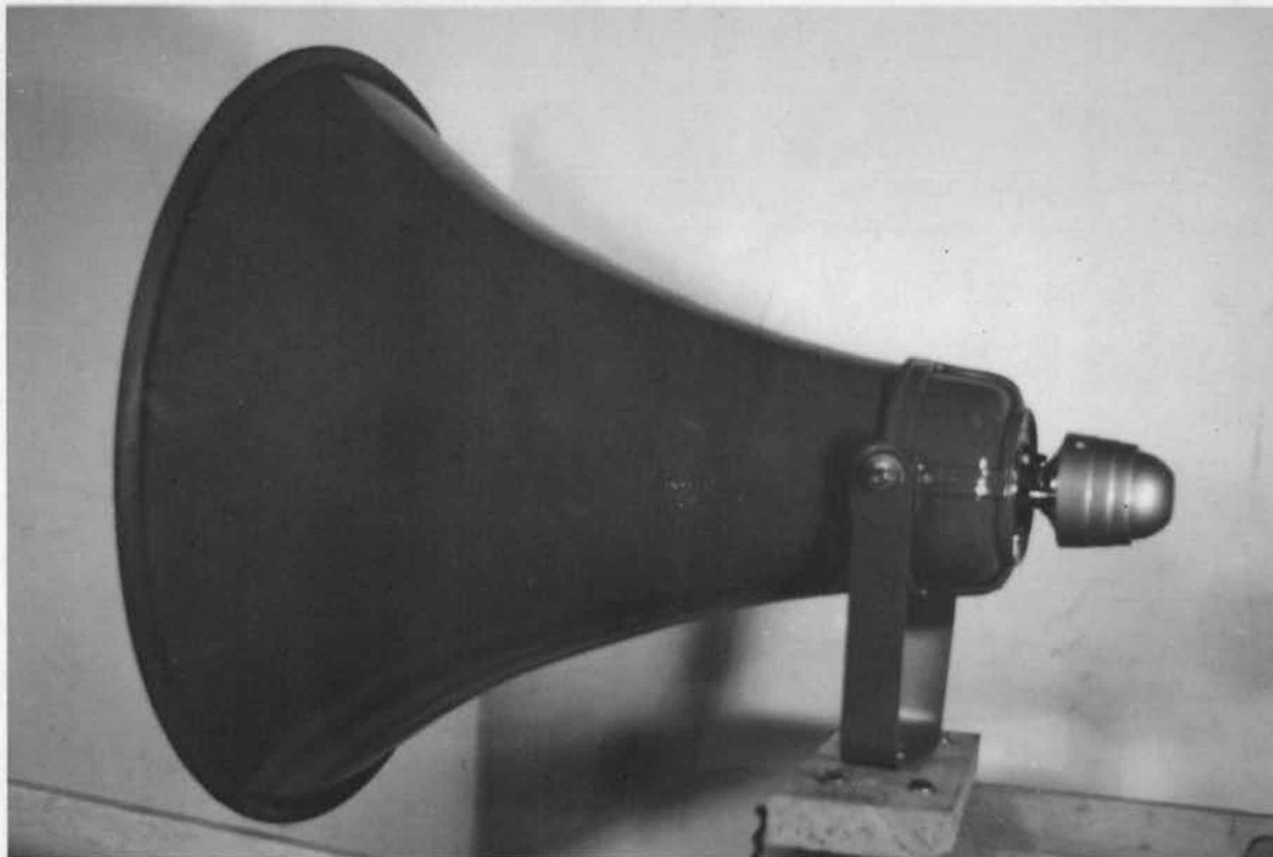
Fig. 8 - Loudspeaker unit composed of Driver "U" and Horn "U" in position and ready for test.
