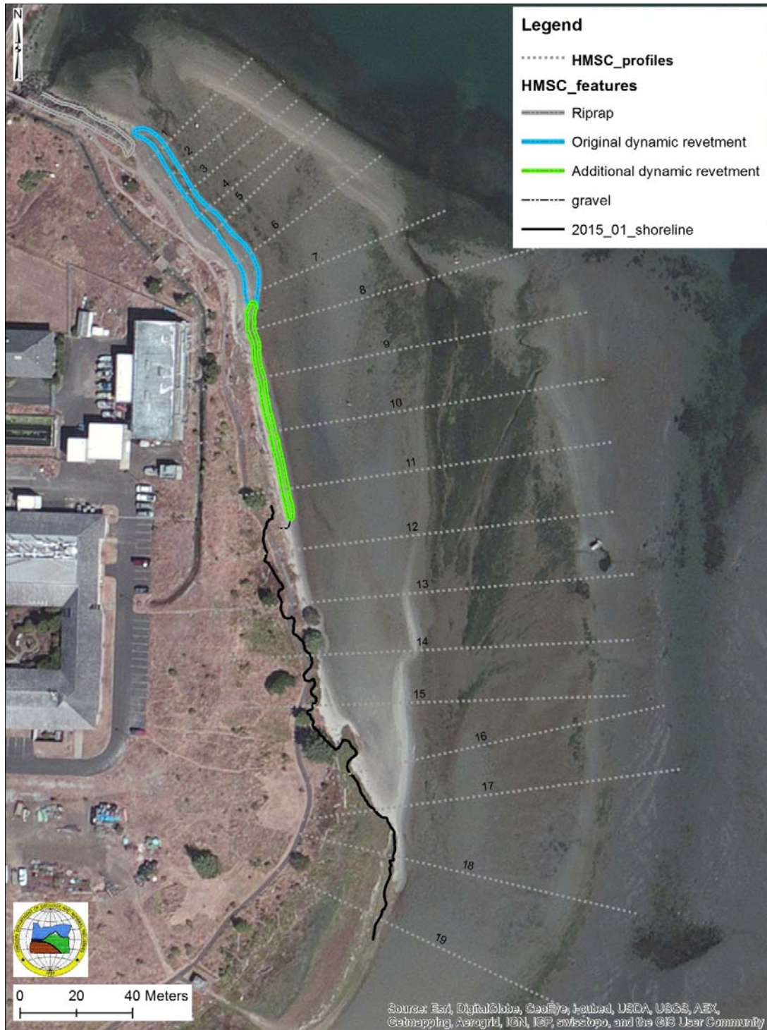
Figure 2.2: Location map showing the HMSC beach and shoreline monitoring network. Blue shaded dashed line denotes the cobble ‘lag’ toe of the original dynamic revetment, green shaded dashed line denotes the cobble ‘lag’ toe for the expanded section and grey shaded dashed line denotes the location of rip rap rock. Solid black line depicts the most recent (January 2015) measurement of the erosion scarp.
