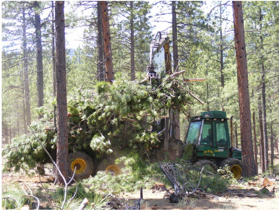
Figure 1.2 Self-loading forwarder carrying ponderosa pine harvest residues in Sisters, Oregon
