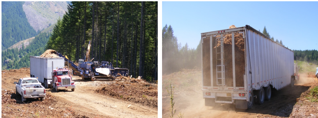
Figure 1.3 a) Forest harvest residue comminution on a cable yarding unit near Vida, Oregon; b) Chip trailer (van) transporting comminuted residues near Vida, Oregon
