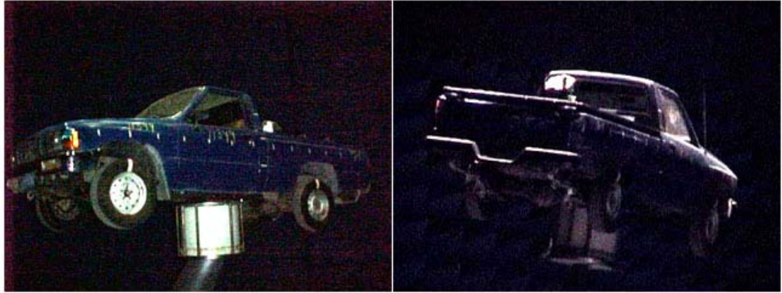
Figure 22. Photo of target on pylon in radar anechoic chamber of actual truck (The data were collected in a 10-story microwave anechoic chamber in Rancho Bernardo, CA. Data was acquired by Prof. Marple and provided for use in this research.)
