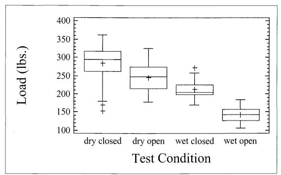
Figure 4.4 Box and whisker plots of load at failure results for dry closed, dry open, wet closed, and wet open samples.
