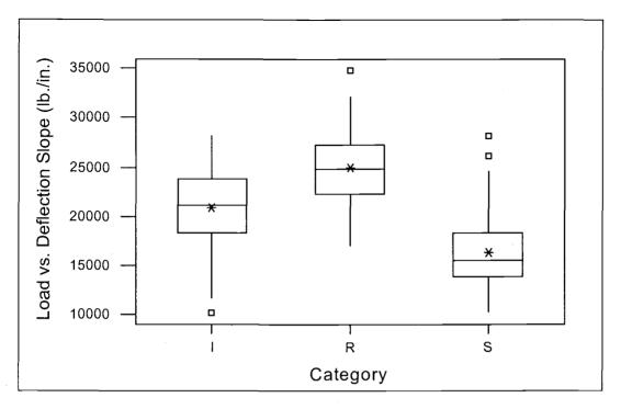
Figure A- 23. Box plot: load vs. deflection slope.
