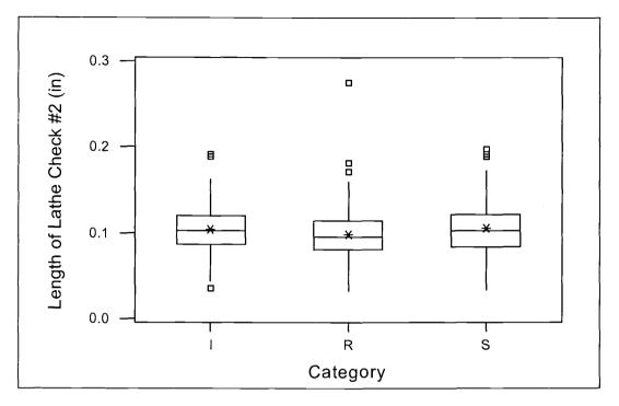
Figure A- 9. Box plot: length of lathe check #2.
