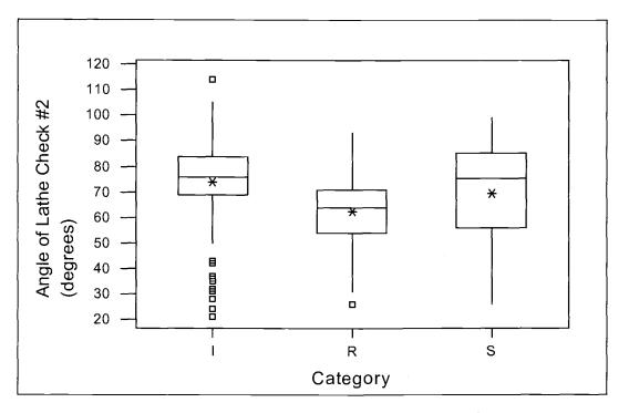
Figure A- 13. Box plot: angle of lathe check #2 to glue-line.
