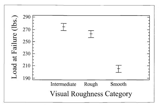
Figure 6.3. 95 percent confidence intervals for average load at failure from smooth, intermediate, and rough visual roughness categories.
