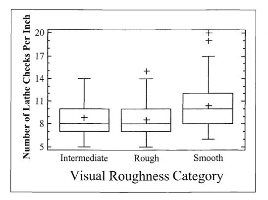
Figure 6.1. Box and whisker plots for lathe check frequency (number of lathe checks per inch) from smooth, intermediate, and rough visual categories.
