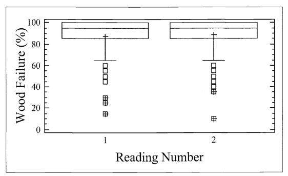
Figure 4.6. Box and whisker plots of percent wood failure readings for preliminary study samples read twice by the same individual.
