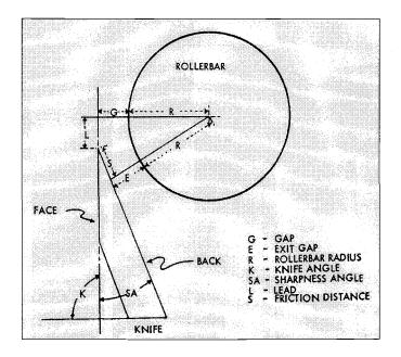
Figure 3.2. Rollerbar, lead, gap and exit gap locations in a lathe setup (15).
