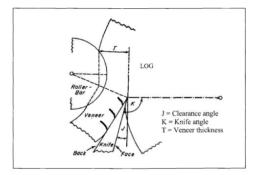
Figure 3.3. Clearance angle and knife angle locations in a lathe setup (62).
