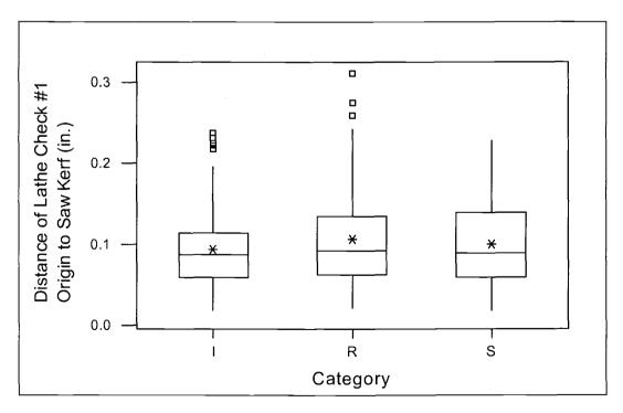
Figure A- 6. Box plot: distance of lathe check #1 origin to saw kerf.
