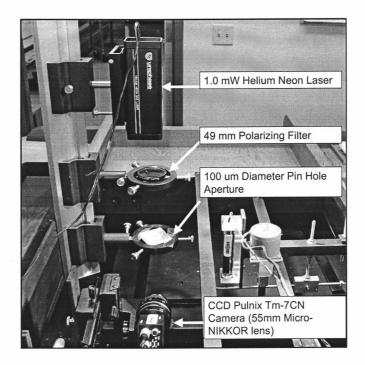
Figure 5.3. Laser scatter/optical imaging system setup.
