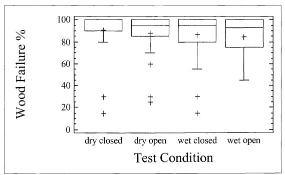
Figure 4.5 Box and whisker plots of percent wood failure results from the first certification agency for dry closed, dry open, wet closed, and wet open samples.
