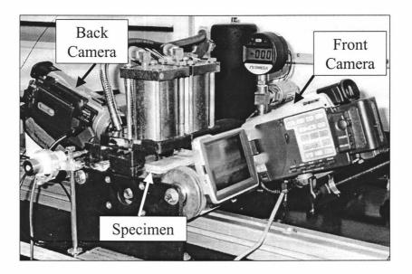
Figure 4.2. Digital video camera system setup.
