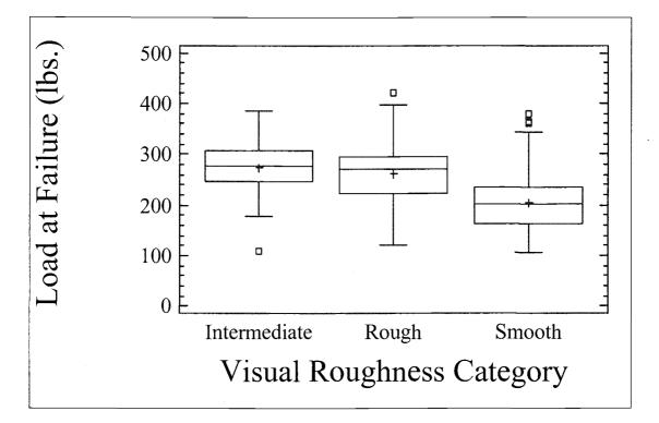
Figure 6.4. Box and whisker plots for load at failure results from smooth, intermediate, and rough visual roughness categories.
