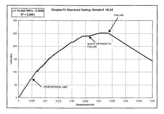
**Figure 6.9.** Typical load versus displacement (measured from head movement) graph obtained from testing plywood glue-bond samples.
