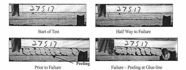
**Figure 6.12.** Failure in the loose-side glue-line due to bending and peeling forces causing rotation of the wood material between lathe checks.
