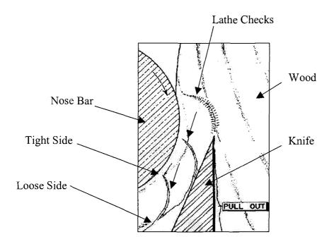
Figure 3.1. Lathe check formation during veneer production (13).
