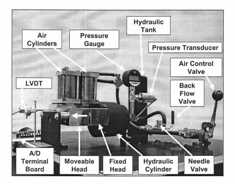
Figure 4.1. Modified TECO-Mater glue-bond test machine.
