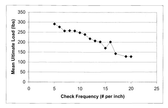
Figure 6.6. Main effects plot on mean load at failure based on lathe check frequency.
