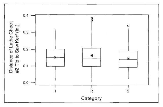
Figure A- 5. Box plot: distance of lathe check #2 tip to saw kerf.
