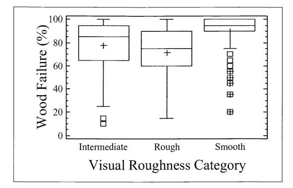
Figure 6.5. Box and whisker plots for percent wood failure readings from smooth, intermediate, and rough visual roughness categories.
