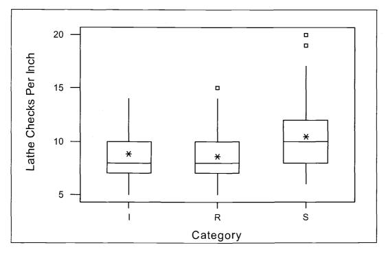
Figure A-1. Box plot: lathe check frequency.
