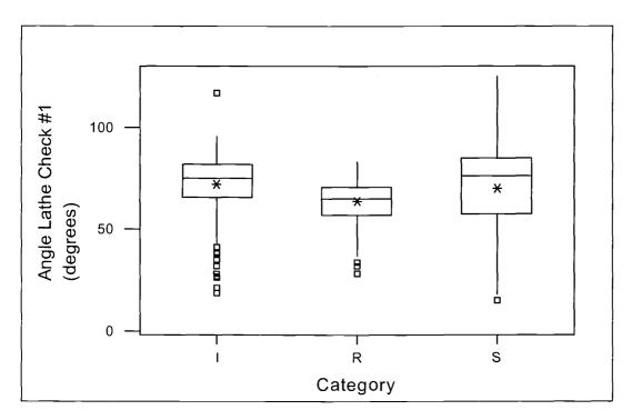
Figure A- 12. Box plot: angle of lathe check #1 to glue-line.
