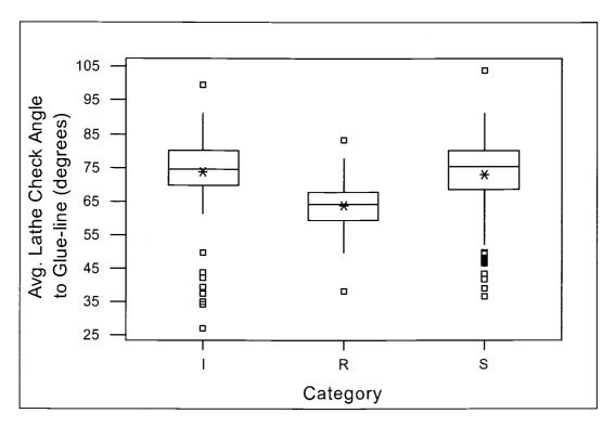
Figure A- 3. Box plot: average lathe check angle to glue-line.
