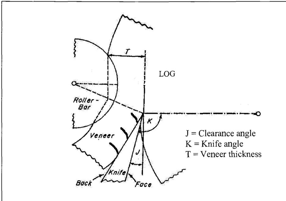
**Figure 3.3.** Clearance angle and knife angle locations in a lathe setup (62).
