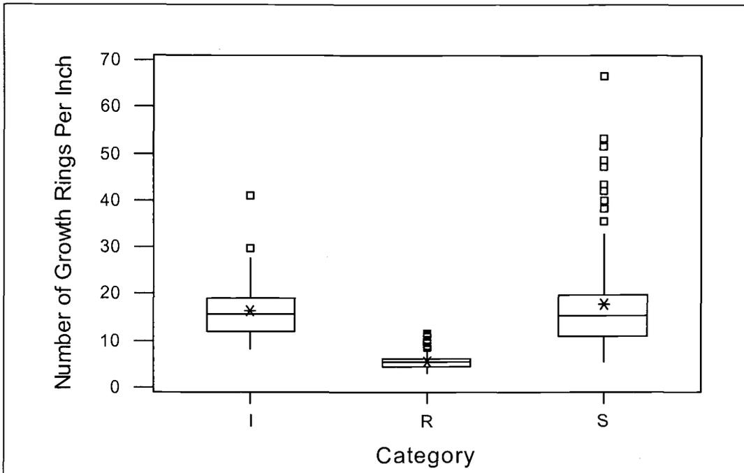
Figure A- 21. Box plot: number of growth rings per inch.
