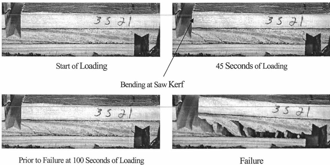
**Figure 6.8.** Apparent bending action at the test specimen's saw kerf locations.
