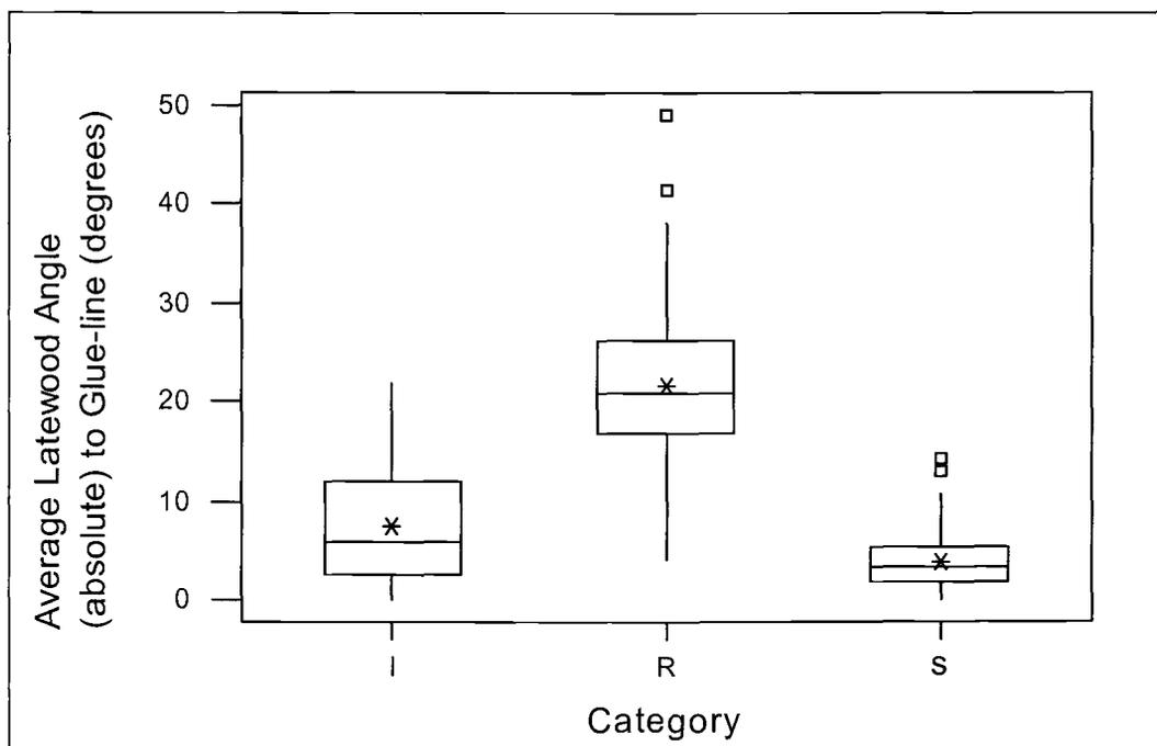
**Figure A- 16.** Box plot: average latewood band angle (absolute) to glue-line.
