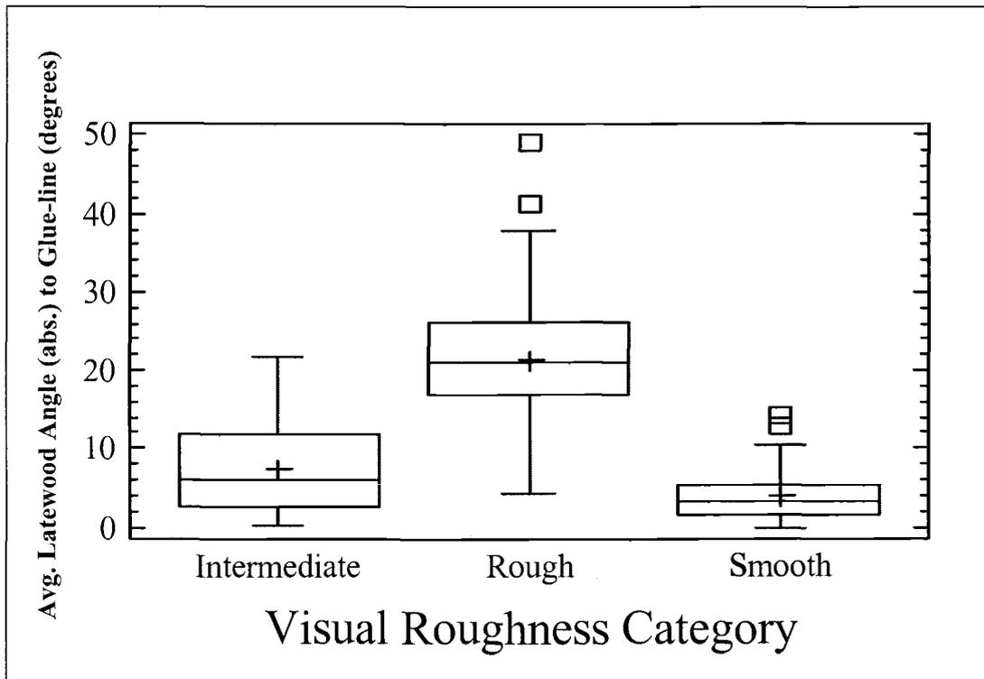
**Figure 6.2.** Box and whisker plots for average latewood angle (absolute) to the glue-line from smooth, intermediate, and rough visual categories.
