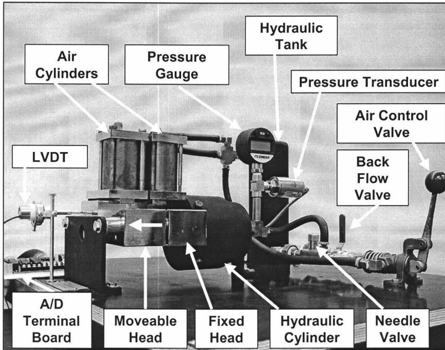
**Figure 4.1.** Modified TECO-Mater glue-bond test machine.
