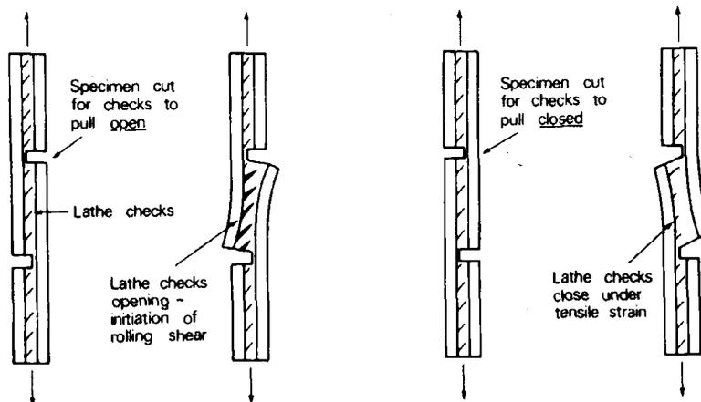
**Figure 3.5.** “Open” versus “closed” sample kerfing methods (72).
