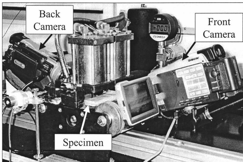
**Figure 4.2.** Digital video camera system setup.
