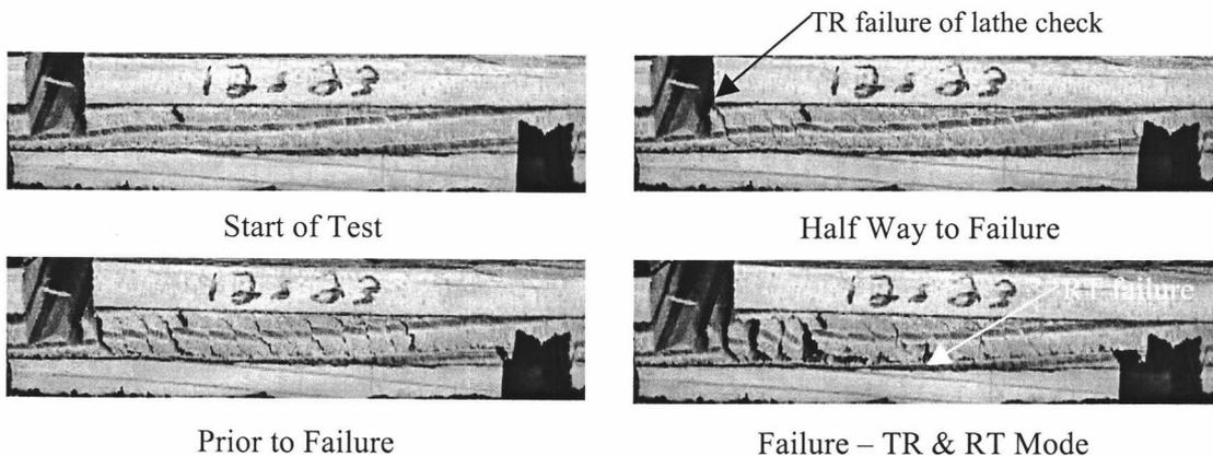
**Figure 6.10.** TR failure of first lathe check followed by RT failure in the rest of the specimen.
