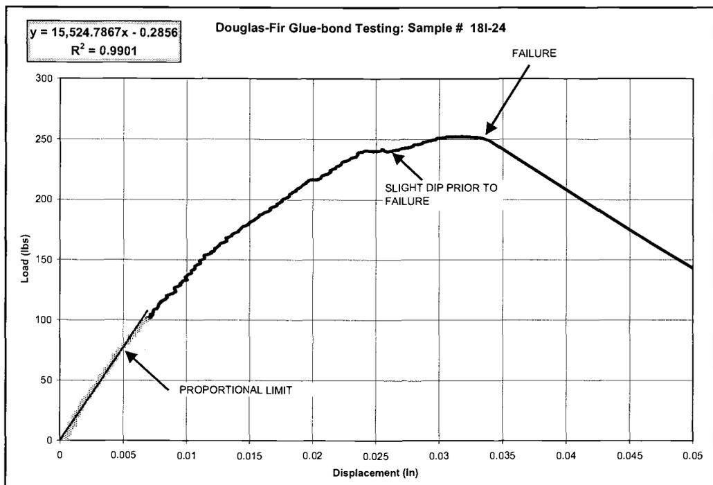
**Figure 6.9.** Typical load versus displacement (measured from head movement) graph obtained from testing plywood glue-bond samples.
