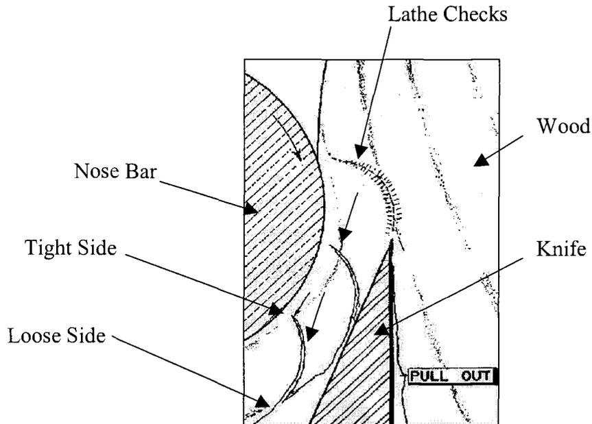
**Figure 3.1.** Lathe check formation during veneer production (13).
