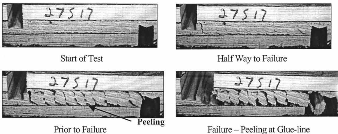
**Figure 6.12.** Failure in the loose-side glue-line due to bending and peeling forces causing rotation of the wood material between lathe checks.
