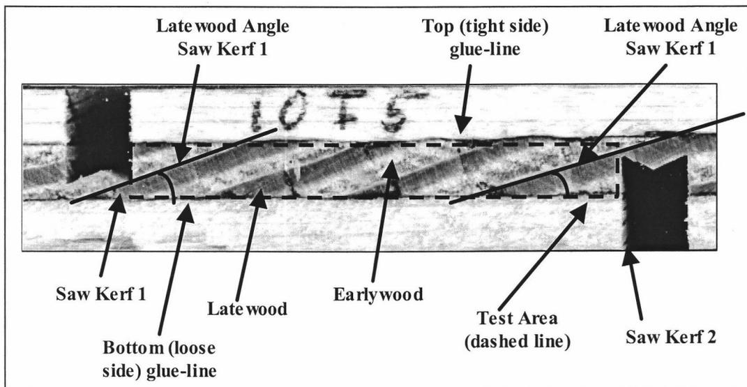
**Figure 5.4.** Example of latewood measurements recorded from scanned glue-bond samples.
