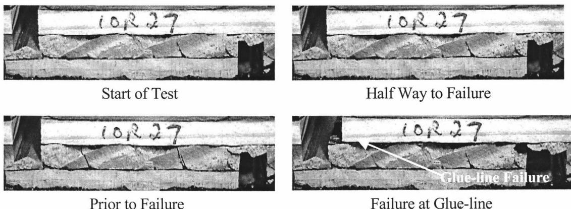
**Figure 6.13.** Failure at the glue-line due to rougher veneer surface and glue-line strength below that of the wood material.
