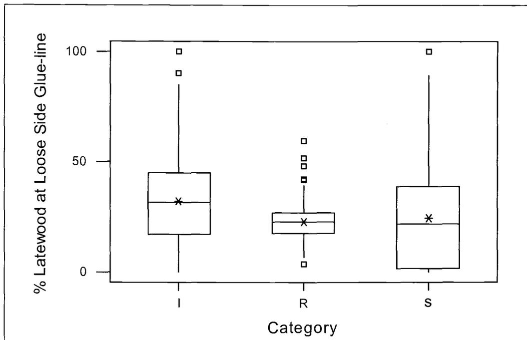
**Figure A- 15.** Box plot: percent latewood at loose-side glue-line.
