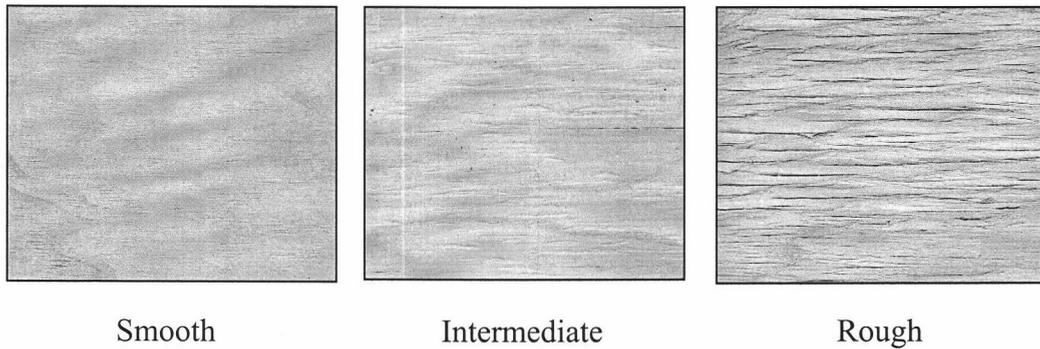
**Figure 5.1.** Example of veneers in the three visual roughness categories.
