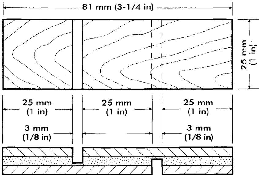
**Figure 3.4.** Bond durability specimen as outlined in PS 1 (82).
