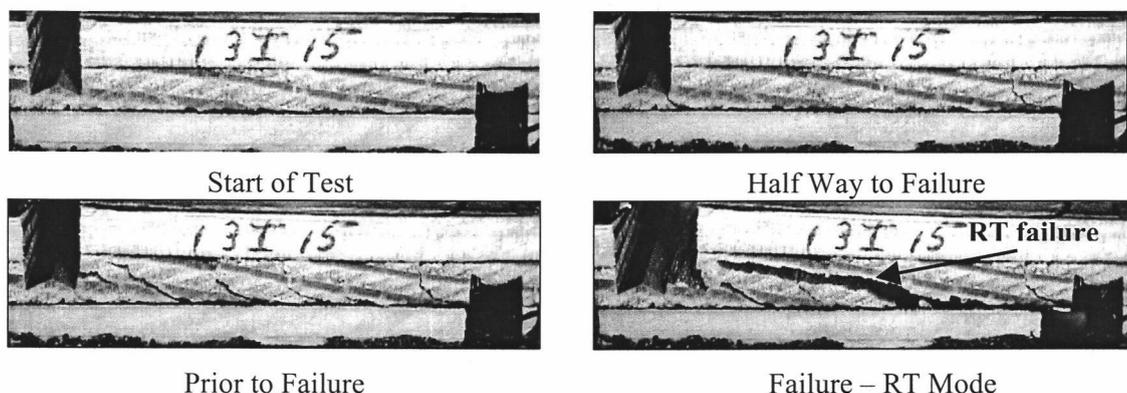
**Figure 6.11.** RT mode failure of first lathe check followed by sudden complete RT failure of the specimen.
