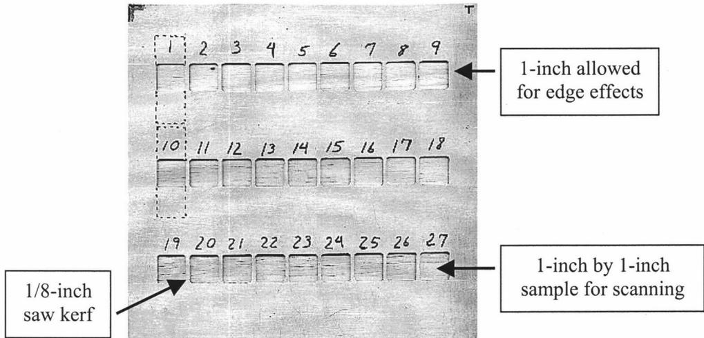
**Figure 5.2.** Metal template over a veneer sheet showing all possible scanning samples.
