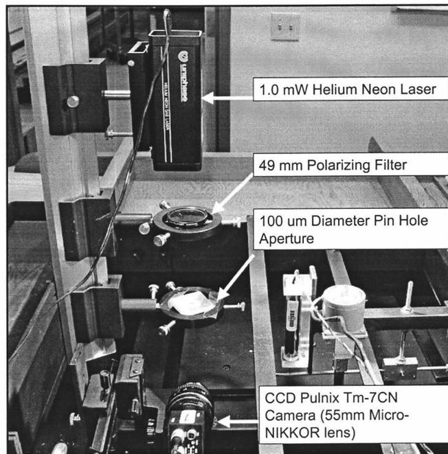
**Figure 5.3.** Laser scatter/optical imaging system setup.
