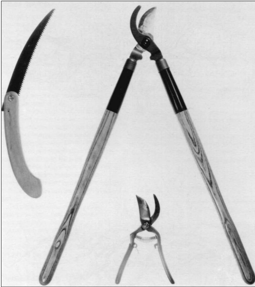
Figure 14.—Pruning saw (upper left), long-handled pruning shears (center), hand shears (bottom).
