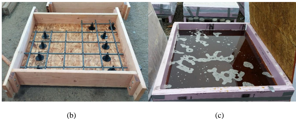
Figure 2.1 – (a) Geometrical details of the concrete slabs; (b) a sample slab with placed reinforcement before casting of concrete; (c) a sample concrete slab during ponding with the deicing solution. The section that is unreinforced was used to take measurements and to extract cores for additional testing.
