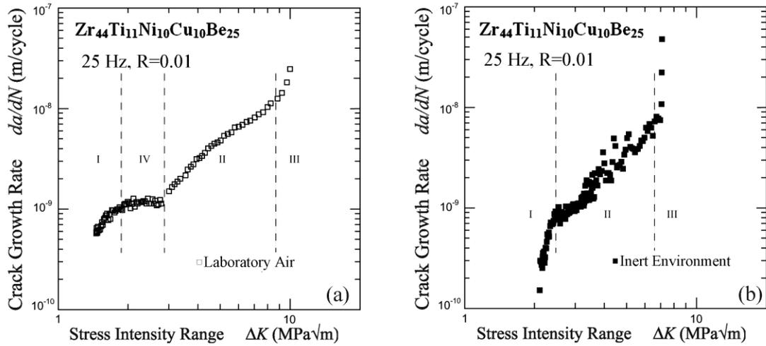
**Figure 5: Fatigue crack growth rate ( $da/dN$ ) plotted as a function of applied stress intensity range ( $\Delta K$ ), for  $Zr_{44}Ti_{11}Ni_{10}Cu_{10}Be_{25}$ . In (a), four discernible growth rate regions are seen for the laboratory air data from Ref. [12], while in (b) three distinguishable growth rate regions are indicated for the purified dry  $N_2$  experiments.**
