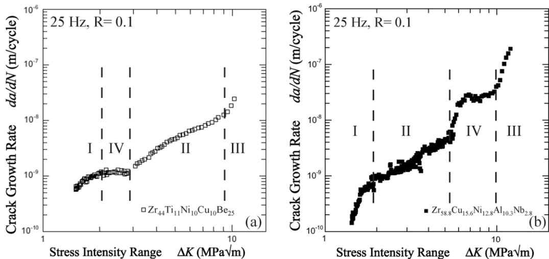
**Figure 9: Fatigue crack growth rate ( $da/dN$ ) plotted as a function of applied stress intensity range ( $\Delta K$ ), in laboratory air. In (a), four discernible growth rate regions are seen for  $\text{Zr}_{44}\text{Ti}_{11}\text{Ni}_{10}\text{Cu}_{10}\text{Be}_{25}$  data from Ref. [12] with a plateau at  $\sim 10^{-9}$  m/cycle, while in (b)  $\text{Zr}_{58.5}\text{Cu}_{15.6}\text{Ni}_{12.8}\text{Al}_{10.3}\text{Nb}_{2.8}$  shows a plateau at  $\sim 2.5 \times 10^{-8}$  m/cycle.**
