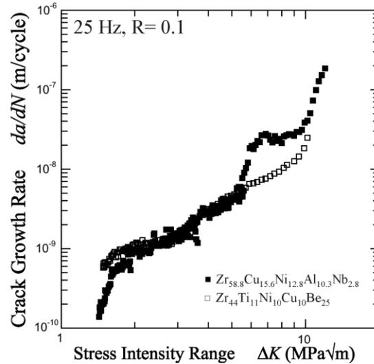
**Figure 8: Fatigue crack growth rates ( $da/dN$ ) plotted as a function of applied stress intensity range ( $\Delta K$ ), for  $\text{Zr}_{44}\text{Ti}_{11}\text{Ni}_{10}\text{Cu}_{10}\text{Be}_{25}$  and  $\text{Zr}_{58.5}\text{Cu}_{15.6}\text{Ni}_{12.8}\text{Al}_{10.3}\text{Nb}_{2.8}$  BMGs tested in laboratory air. Data for  $\text{Zr}_{44}\text{Ti}_{11}\text{Ni}_{10}\text{Cu}_{10}\text{Be}_{25}$  were taken from Ref. [12].**
