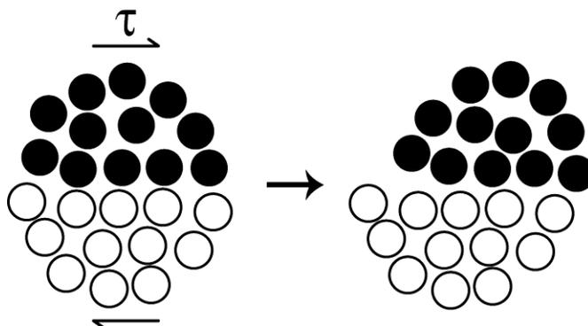
**Figure 1: Motion of atomic clusters in an amorphous material: an atomic rotation of the darker top cluster of atoms relative to the lighter cluster at the bottom.**
