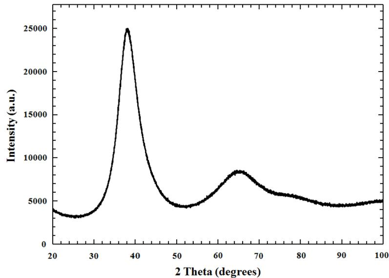
**Figure 7: X-ray diffraction (XRD) scan of fully amorphous  $Zr_{58.5}Cu_{15.6}Ni_{12.8}Al_{10.3}Nb_{2.8}$ . The scan was run at 0.1 degrees per second at room temperature.**
