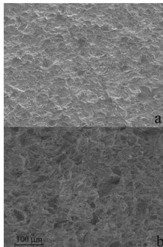
**Figure 6: Scanning electron micrograph comparisons of medium-growth-rate fatigue fracture surfaces: (a) sample fatigued in purified dry  $\text{N}_2$  (b) sample fatigued in laboratory air.  $\Delta K$  was  $\sim 3 \text{ MPa}\sqrt{\text{m}}$  for both samples and the nominal crack growth direction was left to right.**
