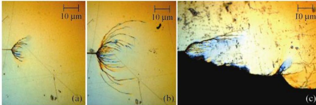
**Figure 10: Optical micrograph comparisons of crack branching perpendicular to the initial crack plane: (a) after initial  $K_c$  test interruption for Sample 3 (b) branch growth after Sample 3 was re-loaded to higher level (c) scalloped edge evidences crack branching in broken Sample 1.**
