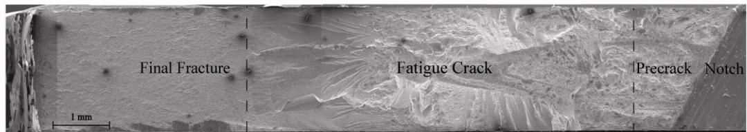
**Figure 11: Scanning electron micrograph of  $Zr_{58.5}Cu_{15.6}Ni_{12.8}Al_{10.3}Nb_{2.8}$  fracture surface, with crack propagating from the right hand side of the image toward the left hand side of the image. This micrograph of Sample 1 shows the rough surface morphology found in each sample.**
