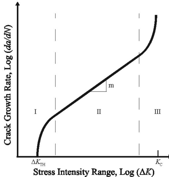
**Figure 2: Characteristic fatigue growth curve for metals.**
