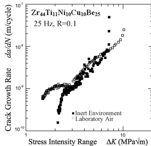
**Figure 4: Fatigue crack growth rates ( $da/dN$ ) plotted as a function of applied stress intensity range ( $\Delta K$ ), for a  $Zr_{44}Ti_{11}Ni_{10}Cu_{10}Be_{25}$  BMG tested in ambient laboratory air and purified dry  $N_2$ . Air data were taken from Ref. [12].**
