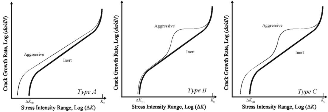
**Figure 3: Types of environmental effect on the fatigue curve of metals.**
