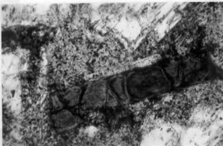
Figure 10. PHOTOMICROGRAPH OF A PORPHYRITIC ANDESITE FROM THE LOWER MEMBER OF THE CLARNO FORMATION. THE LARGE CRYSTAL IN THE CENTER OF THE PICTURE IS AN IRON-RICH MONTMORILLONITE CLAY MINERAL PSEUDOMORPHOUS AFTER CLINOPYROXENE. 35X, PLAIN LIGHT.
