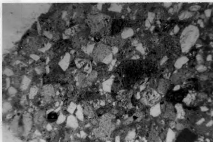
Figure 7. PHOTOMICROGRAPH OF A TUFFACEOUS SANDSTONE SHOWING A ROCK FRAGMENT WITH A PROJECTING PLAGIOCLASE GRAIN (CENTER OF PICTURE). NOTE CLEAR, ANGULAR PLAGIOCLASE GRAINS IN THE MATRIX. 25X, PLAIN LIGHT.
