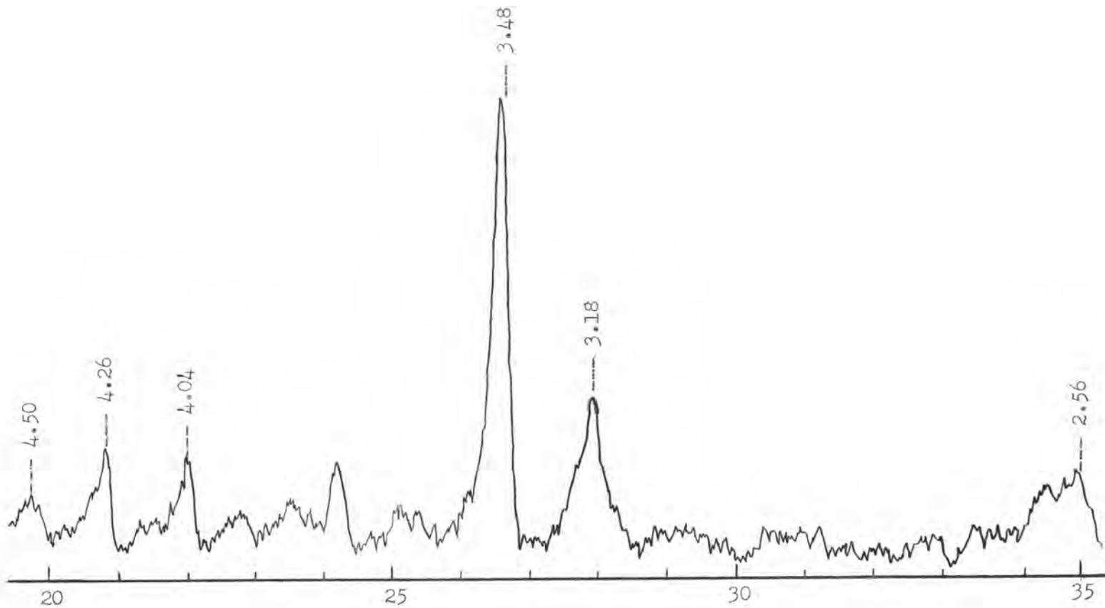
Figure 2. X-RAY DIFFRACTION PATTERN OF THE SANDSTONE FROM THE MUDDY RANCH PHYLLITE.
