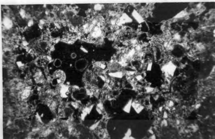
Figure 6. PHOTOMICROGRAPH OF TUFF BRECCIA. IRREGULAR SHAPED PALAGONITE PARTICLE (CENTER), AND DARK ROCK FRAGMENTS. NOTE ANGULAR FELDSPAR GRAINS IN THE MATRIX, AND ROCK FRAGMENT WITH PROJECTING PHENOCRYSTS OF PLAGIOCLASE (UPPER RIGHT CENTER). 25X, PLAIN LIGHT.
