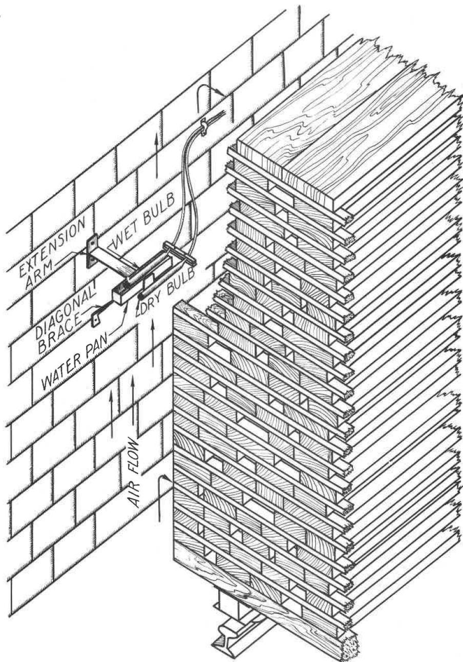
Figure 3. --Control bulbs mounted on kiln wall so that the bulbs are far enough from the wall to be in the entering-air stream.
