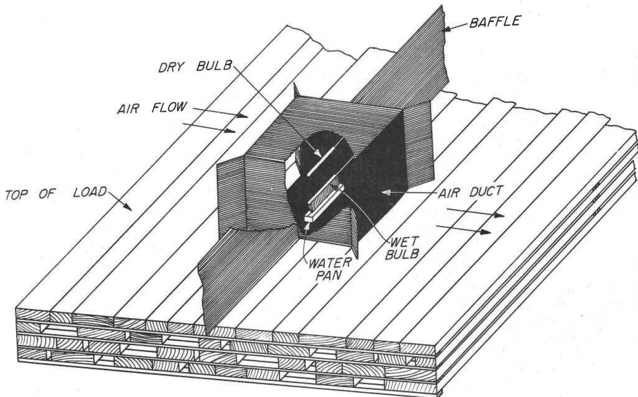
Figure 6. --Single dry bulb mounted above the load in a single-track kiln, so that it will control the entering-air temperature regardless of the direction of air circulation. The wet bulb may be located in a more accessible location.
