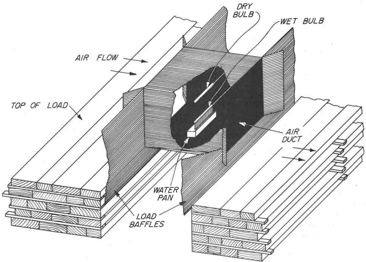
Figure 7. --Single dry bulb located above the loads in a double-track kiln, so that it will control the entering-air temperature regardless of the direction of air circulation. The wet bulb may be located in a more accessible location.
