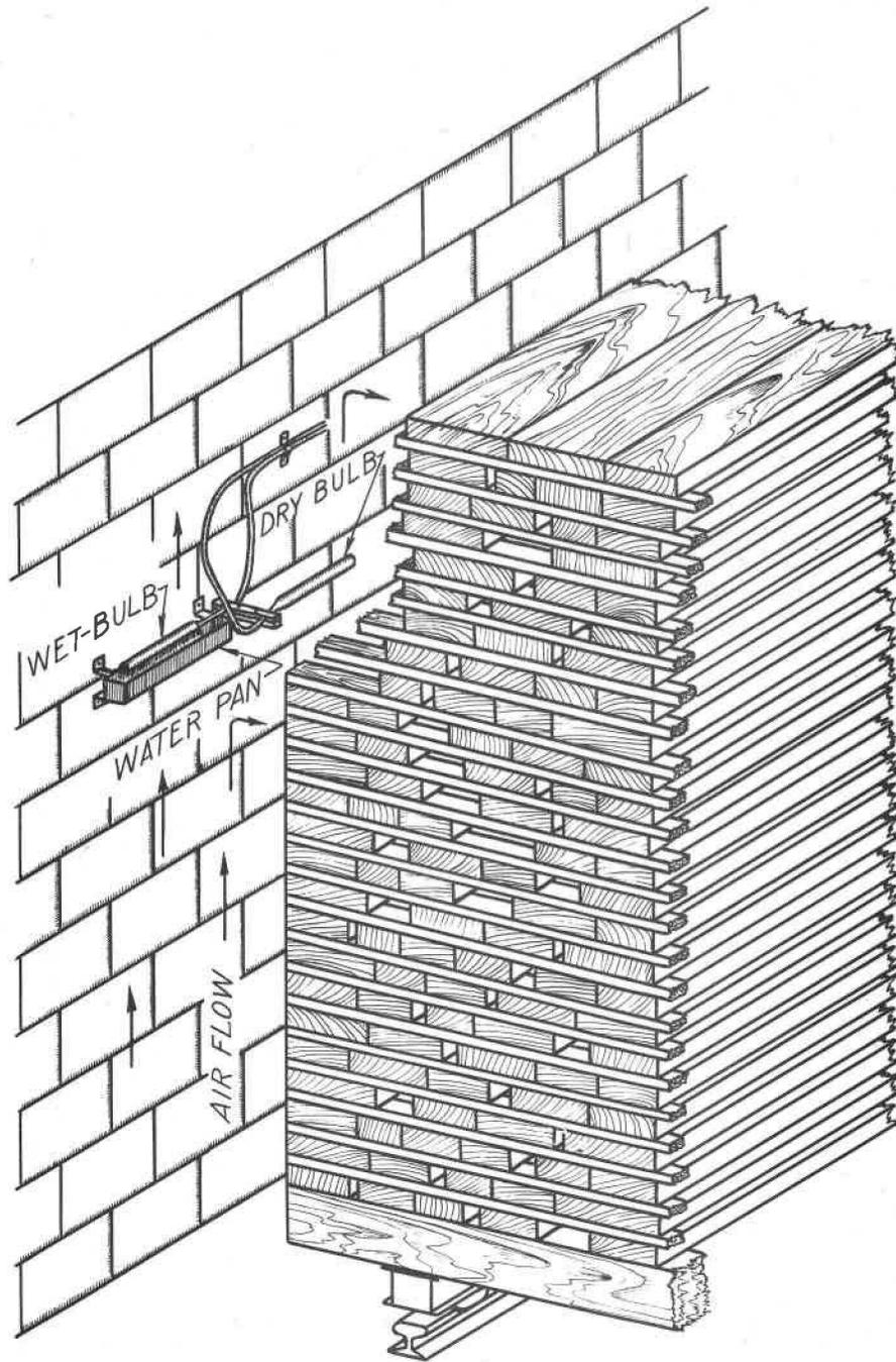
Figure 2. --Control bulb mounted on kiln wall. These bulbs may be too close to the wall to permit circulating air to contact them properly.
