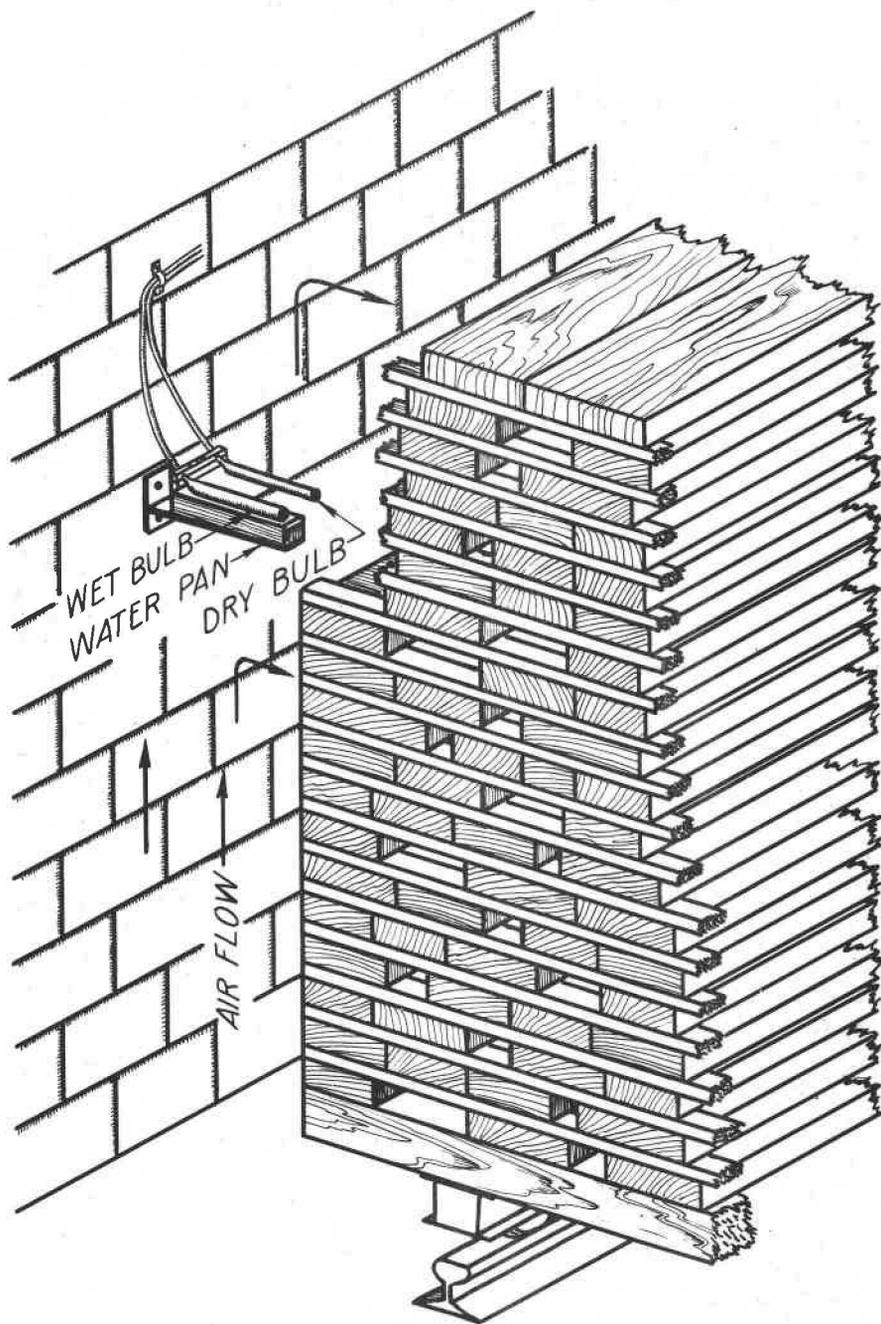
Figure 4. --Control bulbs mounted perpendicular to kiln wall.
