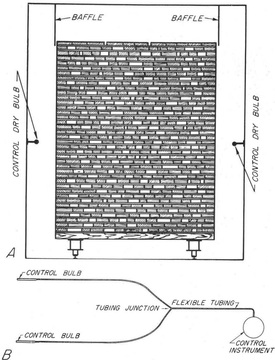
Figure 9. --Dual dry-bulb control system. In A, dry bulbs are located on opposite kiln walls. B presents schematic arrangement of dual dry bulbs, capillary tubing, and control instrument.
