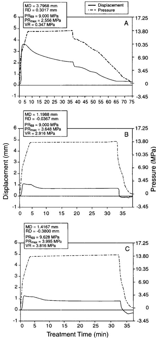
FIG. 3. Effect of venting rate on deformation of white spruce lumber during supercritical fluid impregnation with carbon dioxide when the target venting rate is (A) 0.359 MPa/min, (B) 2.560 MPa/min, and (C) 3.788 MPa/min. Measurements as defined in Fig. 2.
